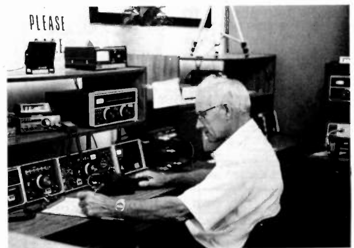
Three complete HF stations with SSTV and RTTY made up the amateur radio exhibit at the Knoxville World's Fair. Information on amateur radio for non-hams was available at WA4KFS.
