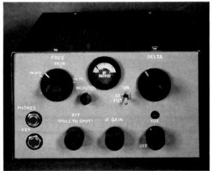
The bfo control (labeled RIT) is mounted where the sidetone level pot used to be. That control (now called MONITOR to save space) is mounted just below and left of the meter.
