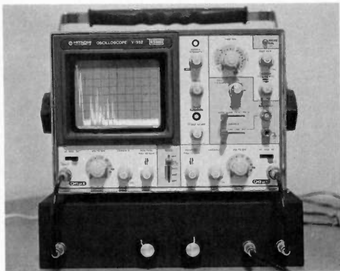
Photo A. High frequency spectrum analyzer covers 0 to 60 MHz.
