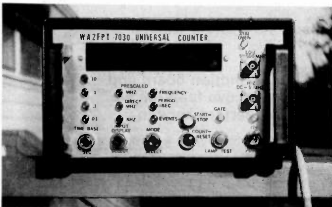
Photo A. Push-button selection is used to control the 7030 Universal Counter.
