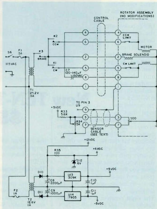
Fig. 4. Power supply and connections to rotator assembly. All circuitry must be insulated from earth ground except potentiometer wiper and motor in the rotator assembly and the cabinet ground on the 115-V ac line.
