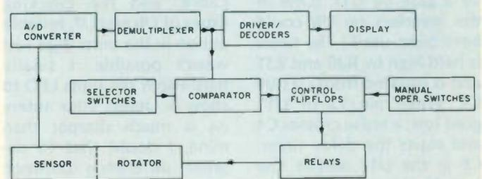
Fig. 1. Automatic rotator control block diagram.
