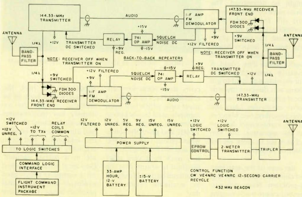
Fig. 1. Flight package.
