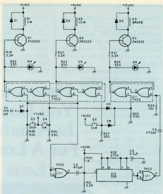
Fig. 3. Control schematic. All circuitry must be insulated from earth ground.
