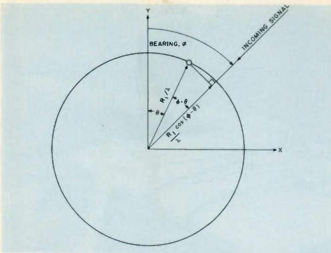
Fig. 2. Geometry used to derive the signal received by a rotating antenna.
