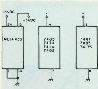
Fig. 5. Supply connections for integrated circuits.
