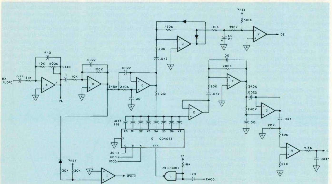
Fig. 13. Audio signal processor circuit schematic. Notes: All op amps are 1/2 LM1458 except H, which is 1/2 CA3240. All diodes are 1N4148. Logic power is  $V_{dd} = +5$ ,  $V_{ee} = -6$ ,  $V_{ss} = \triangle$ . Op amp power is  $+5$  and  $-6$  V dc.
