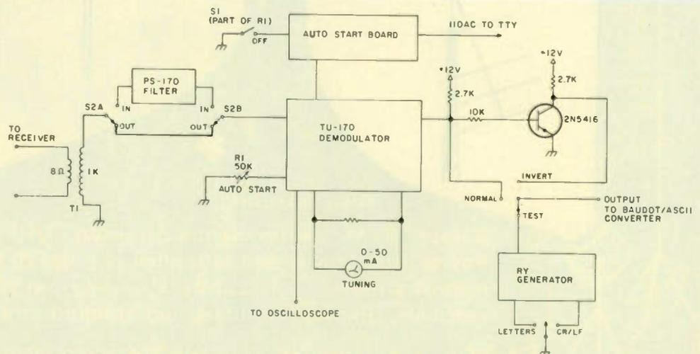
Fig. 2. Block diagram of the TU.
