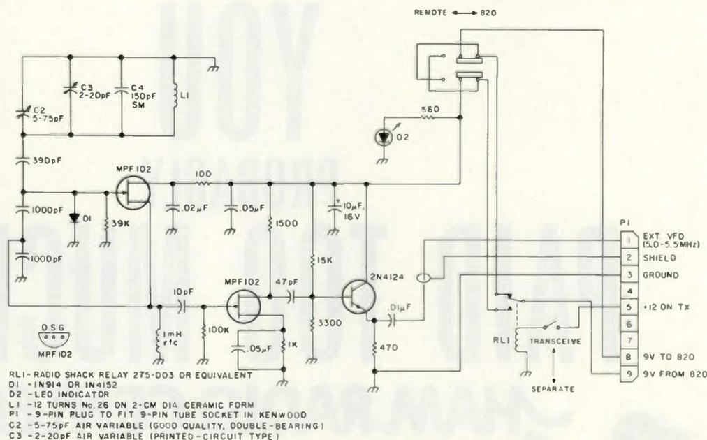
Fig. 1. Schematic for the Kenwood TS-820S remote vfo.
