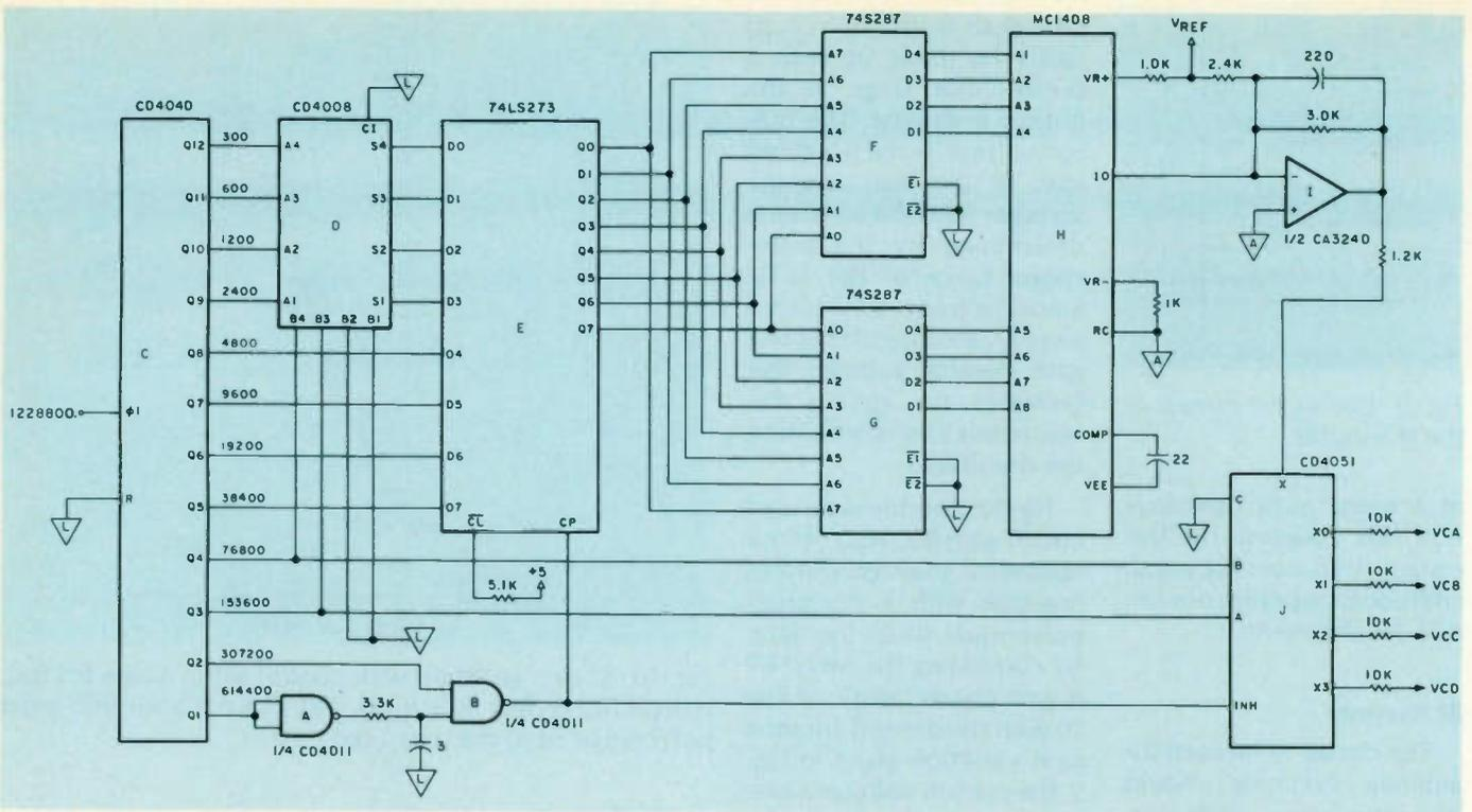
Fig. 12. Circuit schematic of the control voltage waveform generator. Notes: Logic power is  $V_{cc} = V_{dd} = +5$ ,  $V_{ee} = -6$ ,  $V_{ss} = GND = \triangle$ . Op amp power is  $+5$  and  $-6$  V dc.
