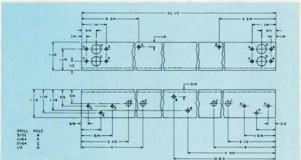
Fig. 23. Side arm construction detail. Two are required.
