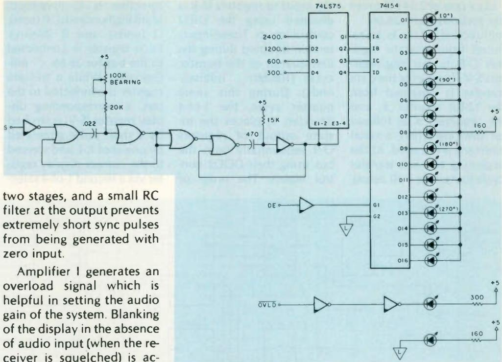
two stages, and a small RC filter at the output prevents extremely short sync pulses from being generated with zero input.
