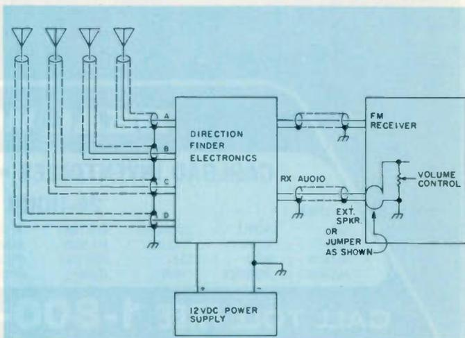
Fig. 30. Basic system connection to antenna, power source, and FM receiver. If a transceiver is used, be sure to disable the transmitter to prevent inadvertent transmission into the RDF electronics.
