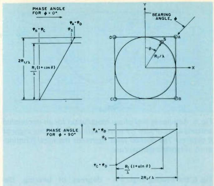
Fig. 4. Top view of a four-antenna array showing the interpolation of phase angle between opposite sides of the array.
