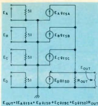
Fig. 9. Equivalent circuit of the rf summer.
