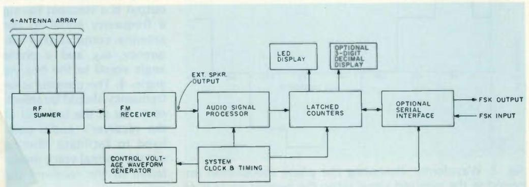
Fig. 1. Block diagram of the complete direction-finding system.
