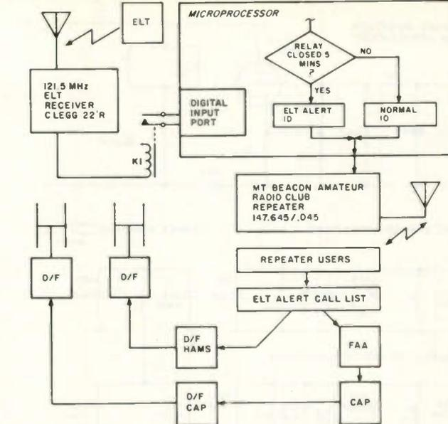
Fig. 1. Emergency Locator Transmitter (ELT) alerting system.
