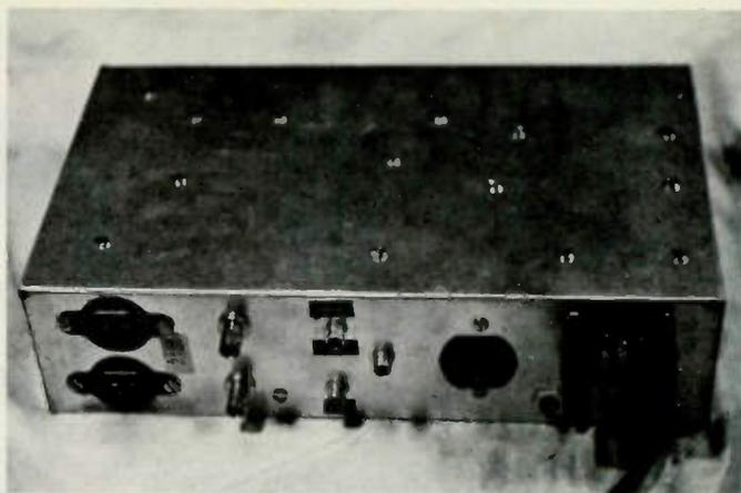
Photo C. Rear view. BNC jacks are for the tuning scope.
