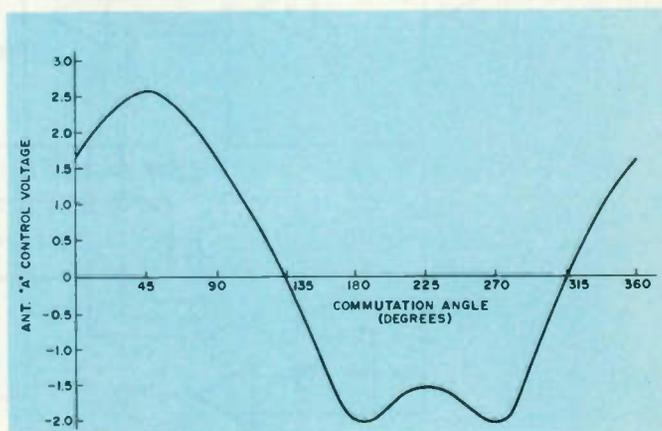
Fig. 11. FET control voltage required to produce the amplitude variation shown in Fig. 5.
