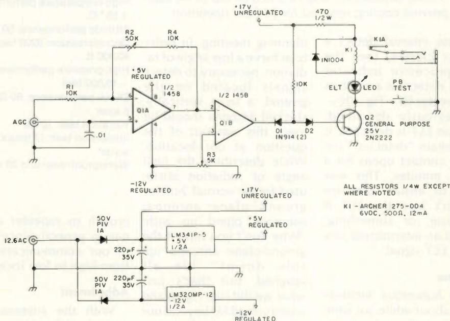
Fig. 2. Interface from Clegg 22'er to microprocessor.
