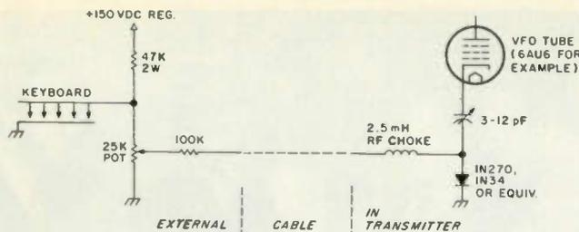
Fig. 2. Shift-pot circuit.
