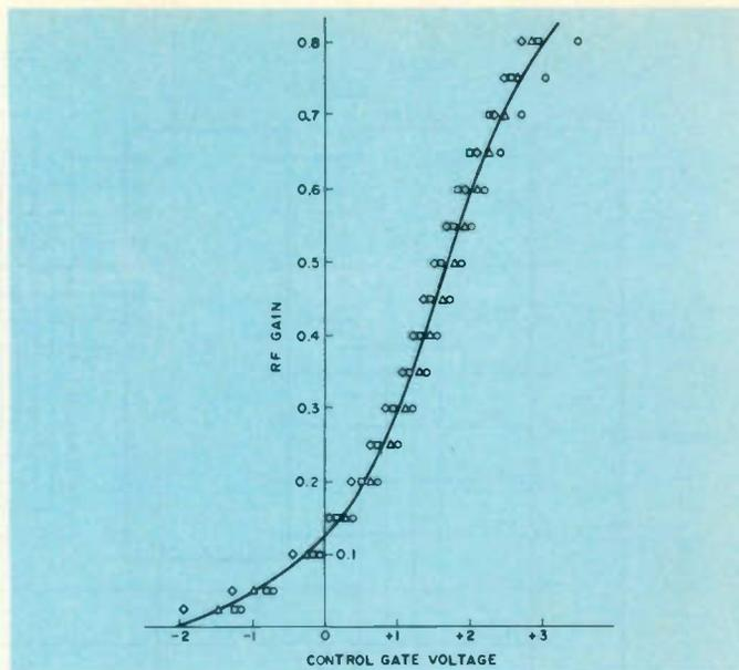
Fig. 10. Rf gain variation with control gate voltage for four typical field-effect transistors. The curve is a seventh-order polynomial fit to the measured data.
