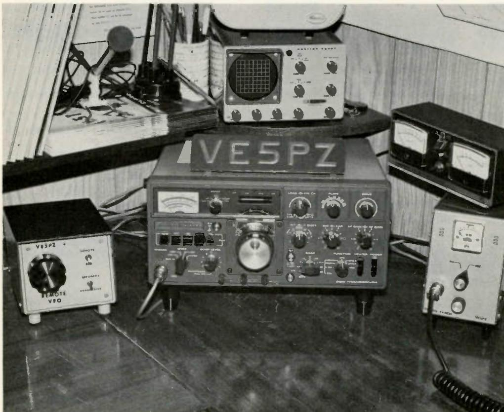
Photo A. The completed remote vfo.
