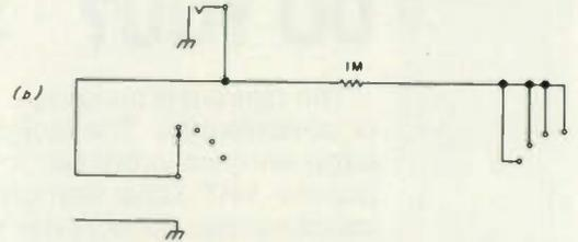
Fig. 2. Moving the 1M resistor inside the IM-17 allows two test leads (plugged into the accessory jack) to be used for all functions.
