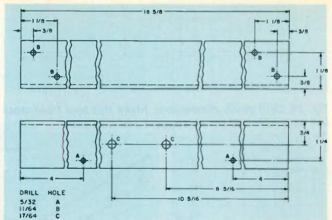
Fig. 22. Center support detail. Only one is required.
