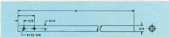
Fig. 20. Vertical element dimensions. Four are required.
