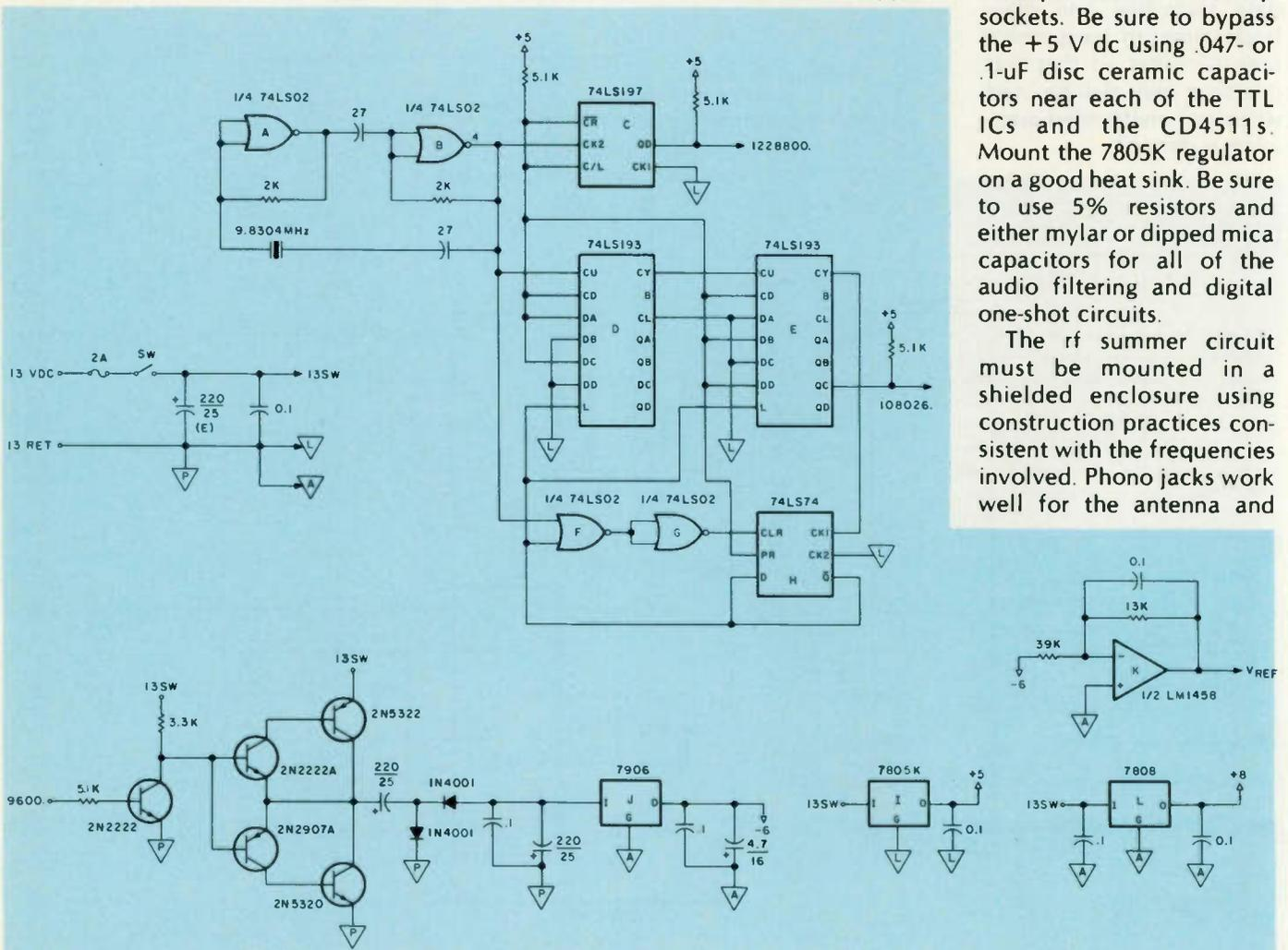
Fig. 17. Schematic of the power supply and clock circuitry. Notes: Power to LM1458 is +5 and -6 V dc. Logic power is  $V_{cc} = +5$ ,  $GND = \triangle$ .
