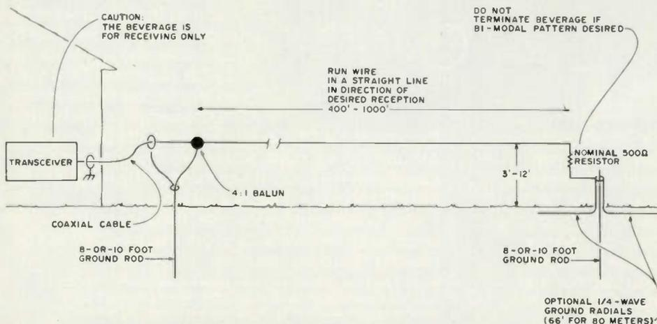
Fig. 1. Installation of the beverage antenna.
