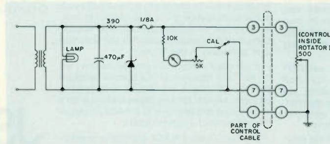
Fig. 6. Unmodified sensing circuit of the Ham III rotator. Wiper of control in rotator is connected to earth ground.
