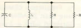
Fig. 1. Negative-resistance oscillator. L and C are the resonant circuit elements. R represents all losses, including output power. The negative resistance of the Gunn diode is represented by -R .
