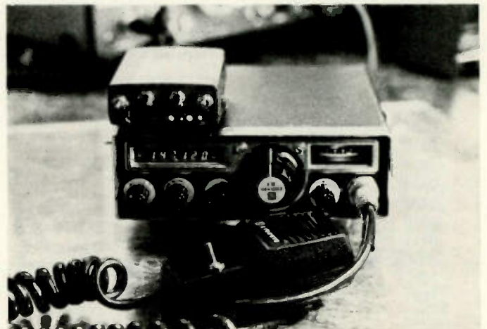
View of the scanner on top of the KDK. Velcro™ is used to hold it in place.
