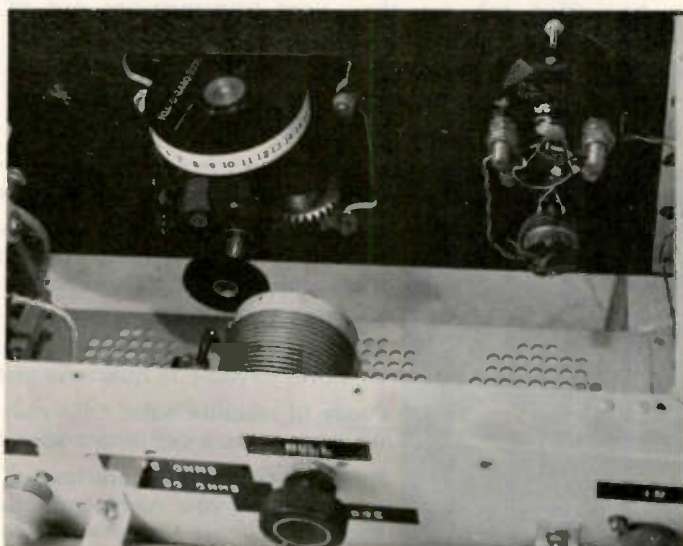
Photo C. ARC-5 roller-coil gear is mounted directly to the dial shaft. Note the protective diodes and bypass capacitor across the swr meter.
