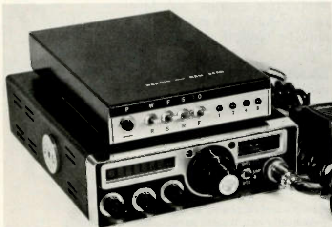
The scanner built by Felix Foggia WA2OFD. Felix chose the PC board route and housed the unit in a 5" x 7" x 3" enclosure cut down to 5" x 7" x 1".
