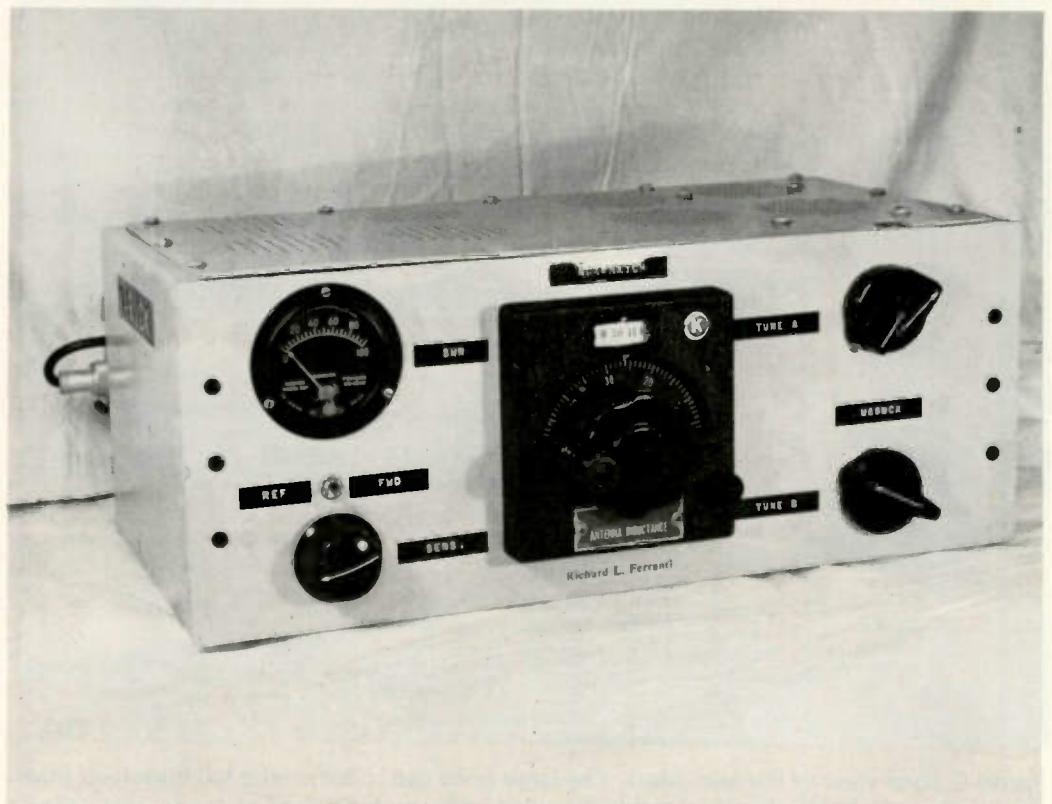
Photo B. The NCX-Match. The swr meter need not be calibrated since you're tuning for a minimum at all times.
