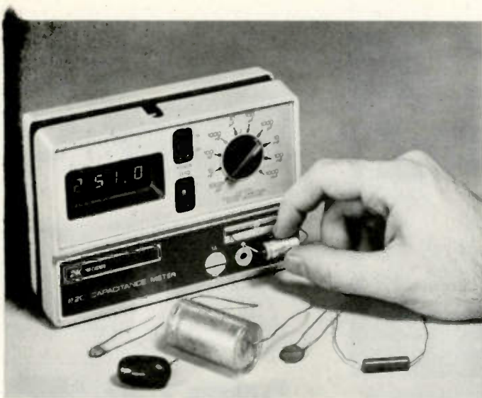
The model 820 portable digital capacitance meter from B&K Precision.
