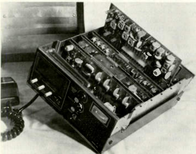
Photo B. CONAR 452 transceiver with top cover removed and receiver board extended.
