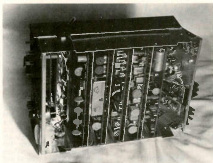
Photo C. Top cover removed to show swing-out panels and T-R relay.
