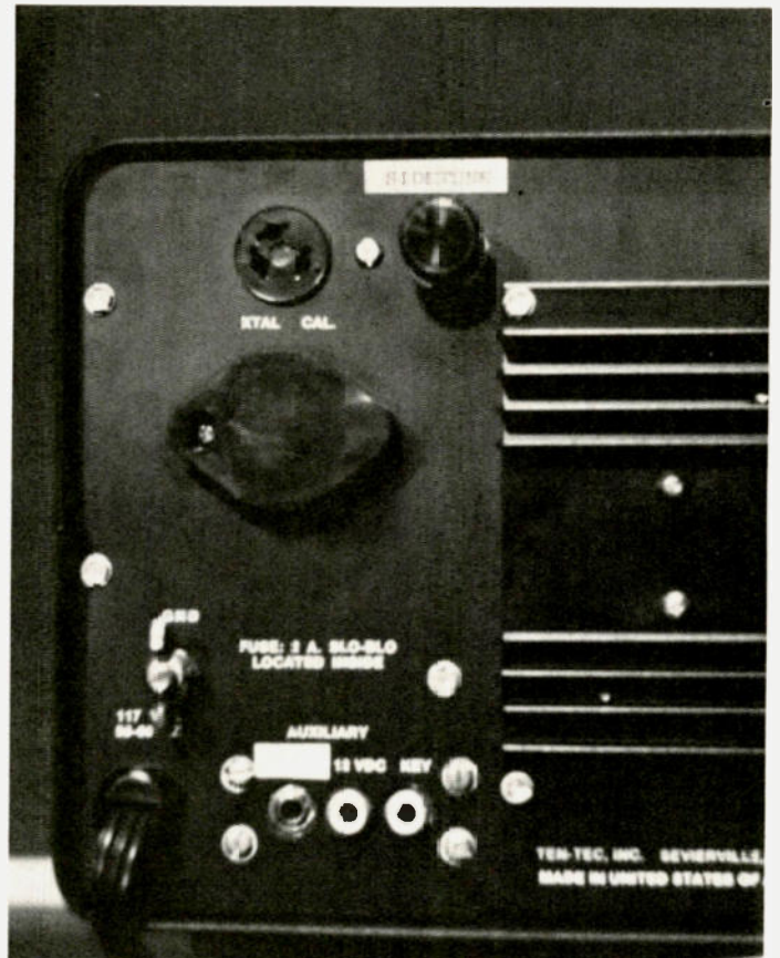
Mounting of the sidetone control and the auxiliary speaker jack.
