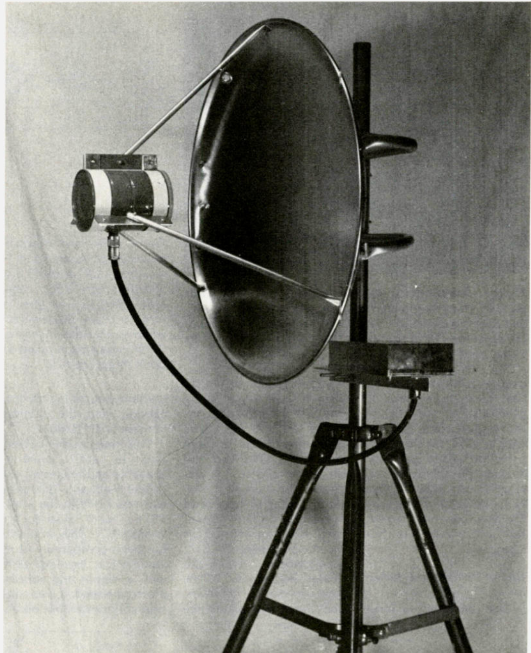
Photo D. This photo shows a complete MDS receive system. The tripod, mast, and U-clamps are standard TV items. All connectors and the box containing the downconverter should be weatherproofed.
