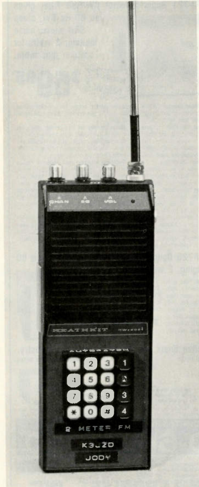
Photo A. Heathkit HW-2021 with the touchtone pad and 1/4-wave antenna installed.
