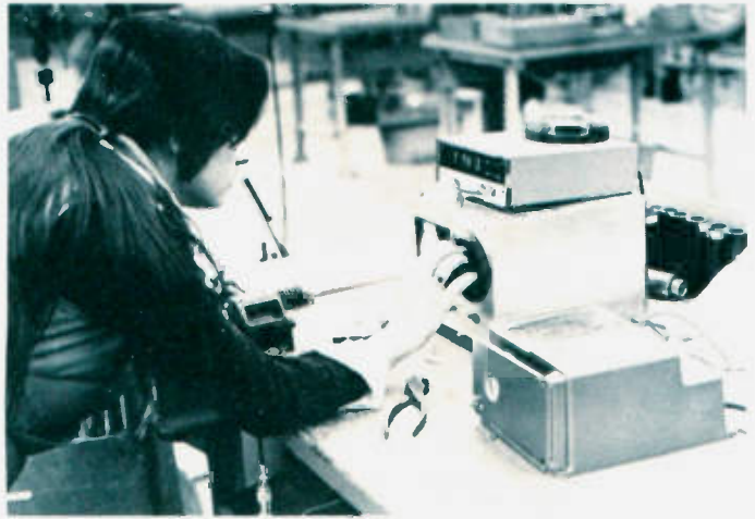
Debbie Narcos is checking the pruning of a coil with an oscillator and frequency counter. They come to her a bit low in frequency, and she gets them right on with the coaxial cable "pencil sharpener" next to her hand.
