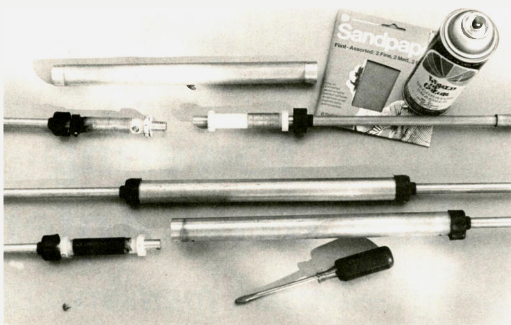
Photo B. This shows what's in a trap and how it's disassembled. The coil in the upper left was charred by a carbonized path, as described in the text. The driven-element coils are coated with Corona Dope to improve rf insulation.
