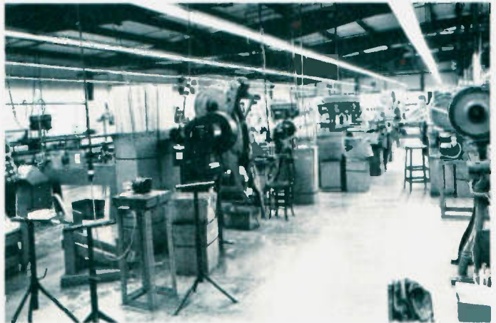
Here's the press department where elements of the various antennas are cut to length and drilled for mountings.
