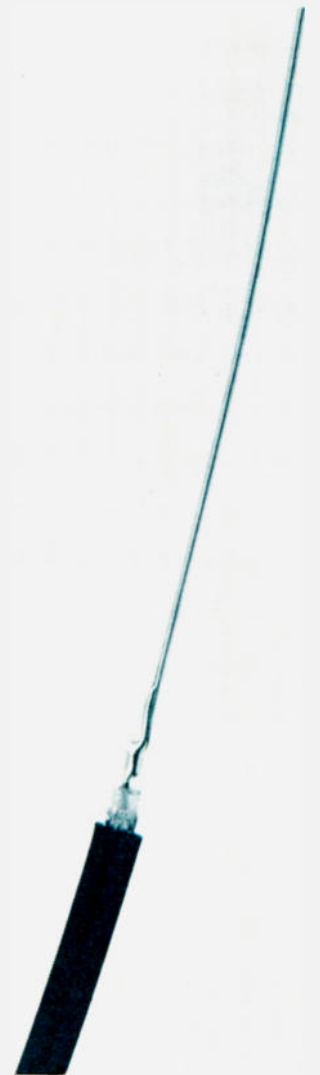
Photo B. Electrical center of T 2 LT vertical antenna.
