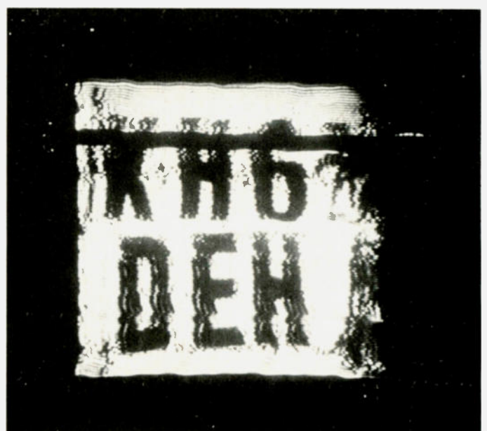
ID of KH6DEH in Hawaii as received in Alabama. The missed lines near the top of the picture were due to a brief burst of noise.
