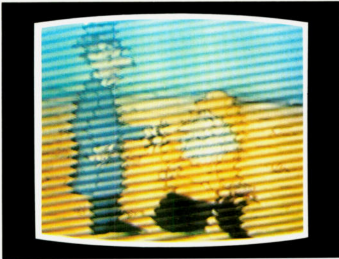
Radio transmitter interference. This is what your picture looks like when it is picking up the transmission of CB, amateur, police, or other radio transmitters. It will normally affect VHF channels only. You may notice that the interference pattern changes or moves as the radio transmitter operator talks. Do not confuse this interference with a horizontal control problem.
