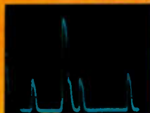
Pan Display: Use to check source of interference during "QSO" without moving off-frequency. Also determines location and strength of adjacent frequencies. (Requires BS-5 or BS-8 option)
