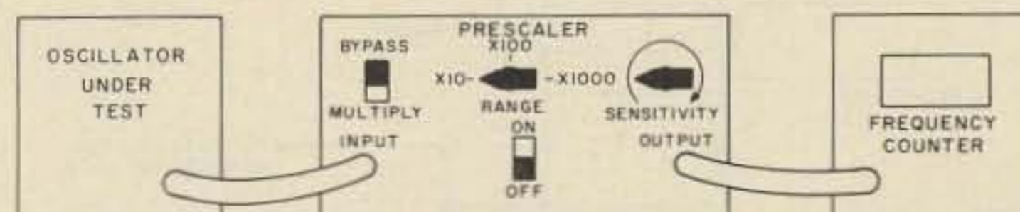
Fig. 11. Test setup for high resolution frequency measurement.
