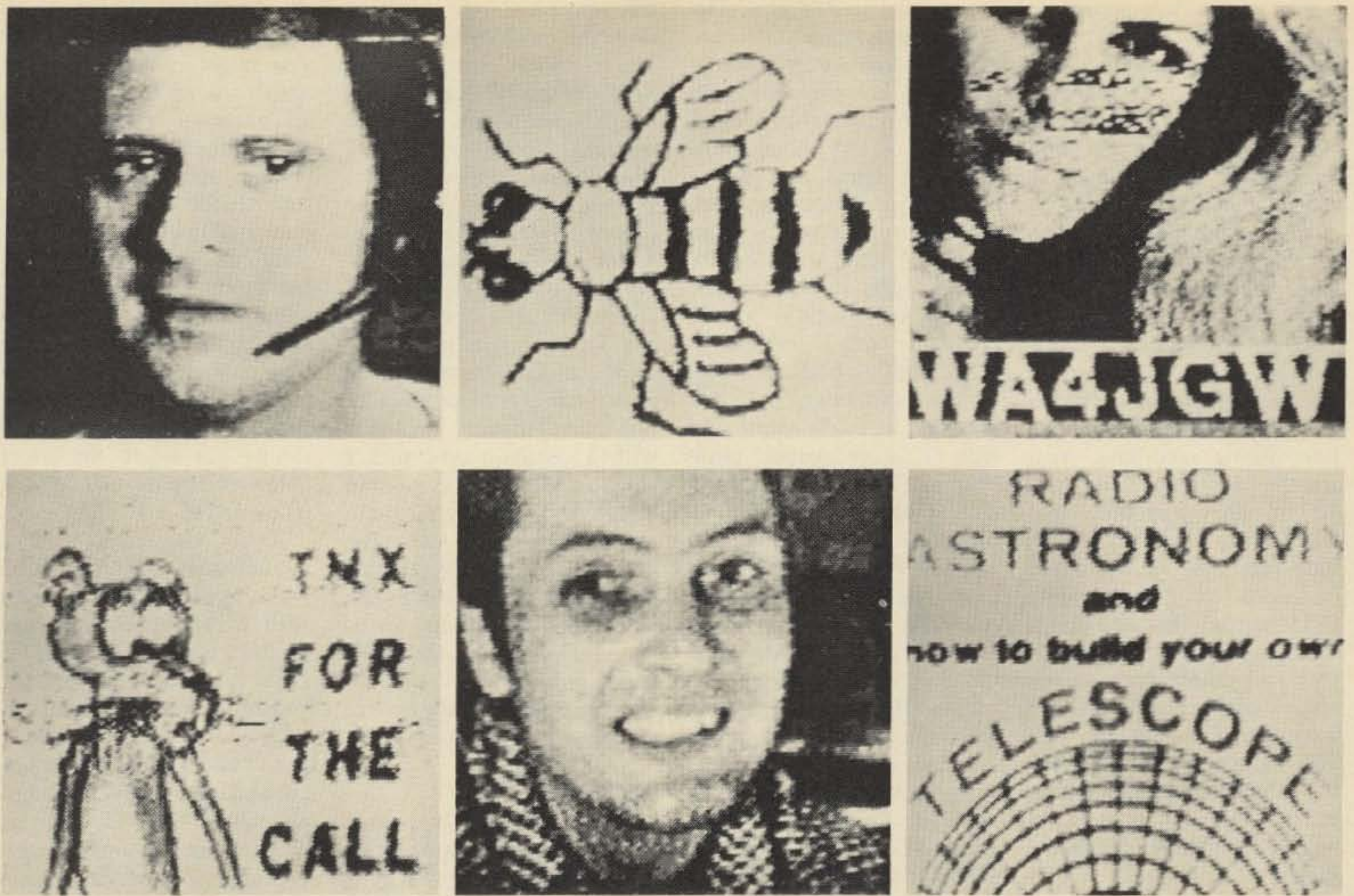
Fig. 4. A collection of miscellaneous SSV pictures logged on 20 meters and displayed on the Robot 400. Only a simple dipole was used for the antenna system and, despite the current state of the band, the 400 delivered excellent pictures. Picture quality in terms of sharpness and contrast is limited only by the care with which pictures are set up at the transmitting end. If you are willing to alter the receive BRIGHTNESS and CONTRAST controls from their proper settings, even pictures of poor quality can be improved considerably. I tend not to alter these controls once they are properly set, as I want to be constantly in a position to realistically evaluate picture quality, and the replay (from the 400 memory) of a station's pictures can do wonders in getting the operator at the other end to set the pictures up more carefully!
