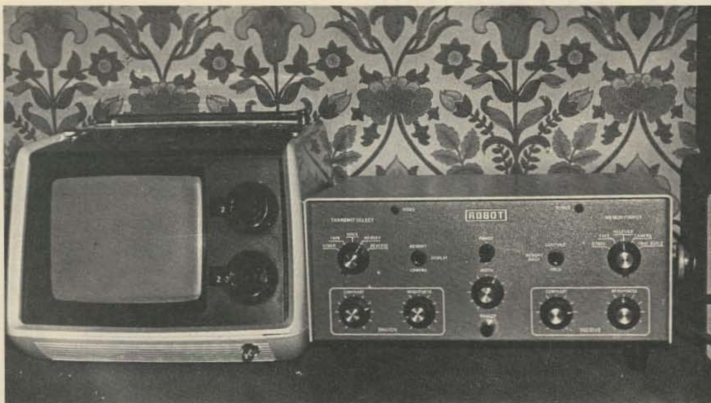
Fig. 1. The Robot Model 400 digital scan converter and the Sony TV-770 which has been modified to serve as a video monitor. A set of this size is ideal for viewing at the distances encountered in most installations. The 400 is very compact and generates essentially no heat, allowing it to be placed anywhere that is convenient.
