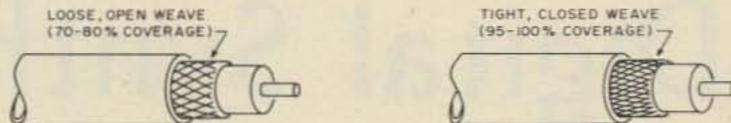
Fig. 7. Cheap coax: bad on left, good on right.
