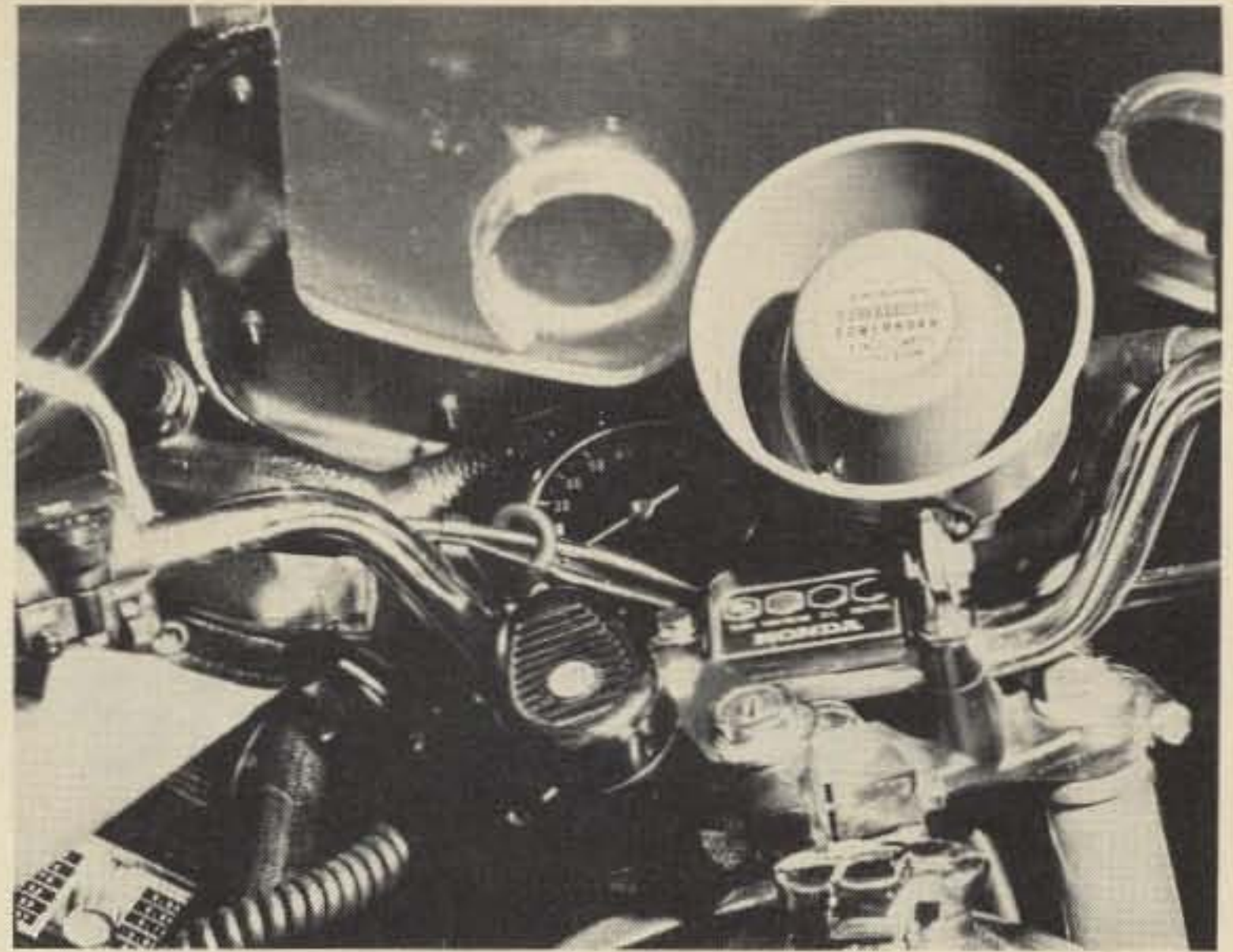
First try at going mobile — external speaker and hand-held microphone.
