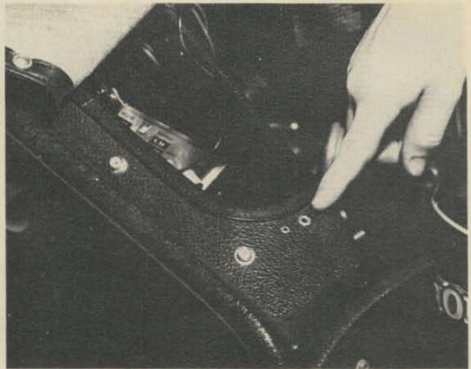
Helmet jacks mounted in fairing.
