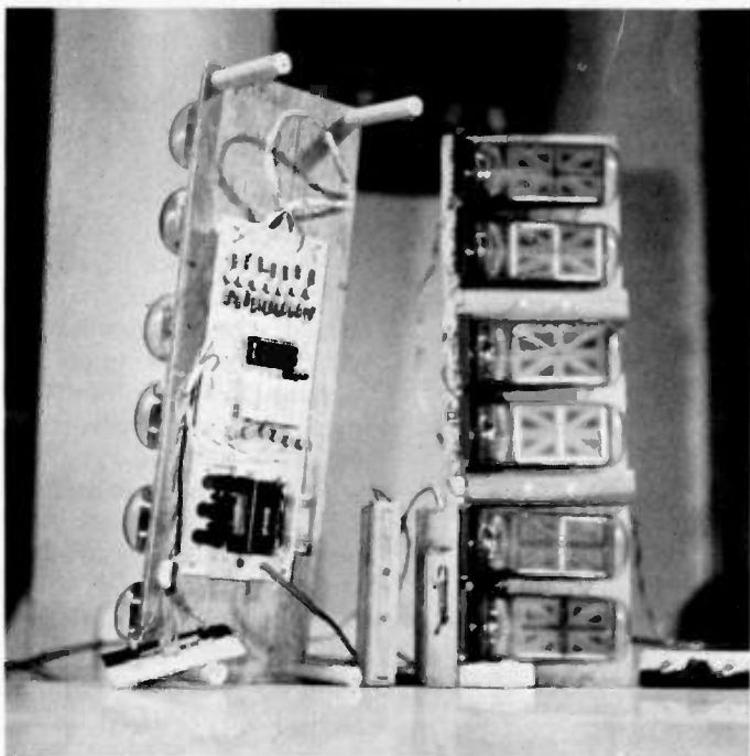
Two clocks, ready for cabinet, standing on end. A pair of colon blocks, viewed from the front and rear, stand between the clocks.
