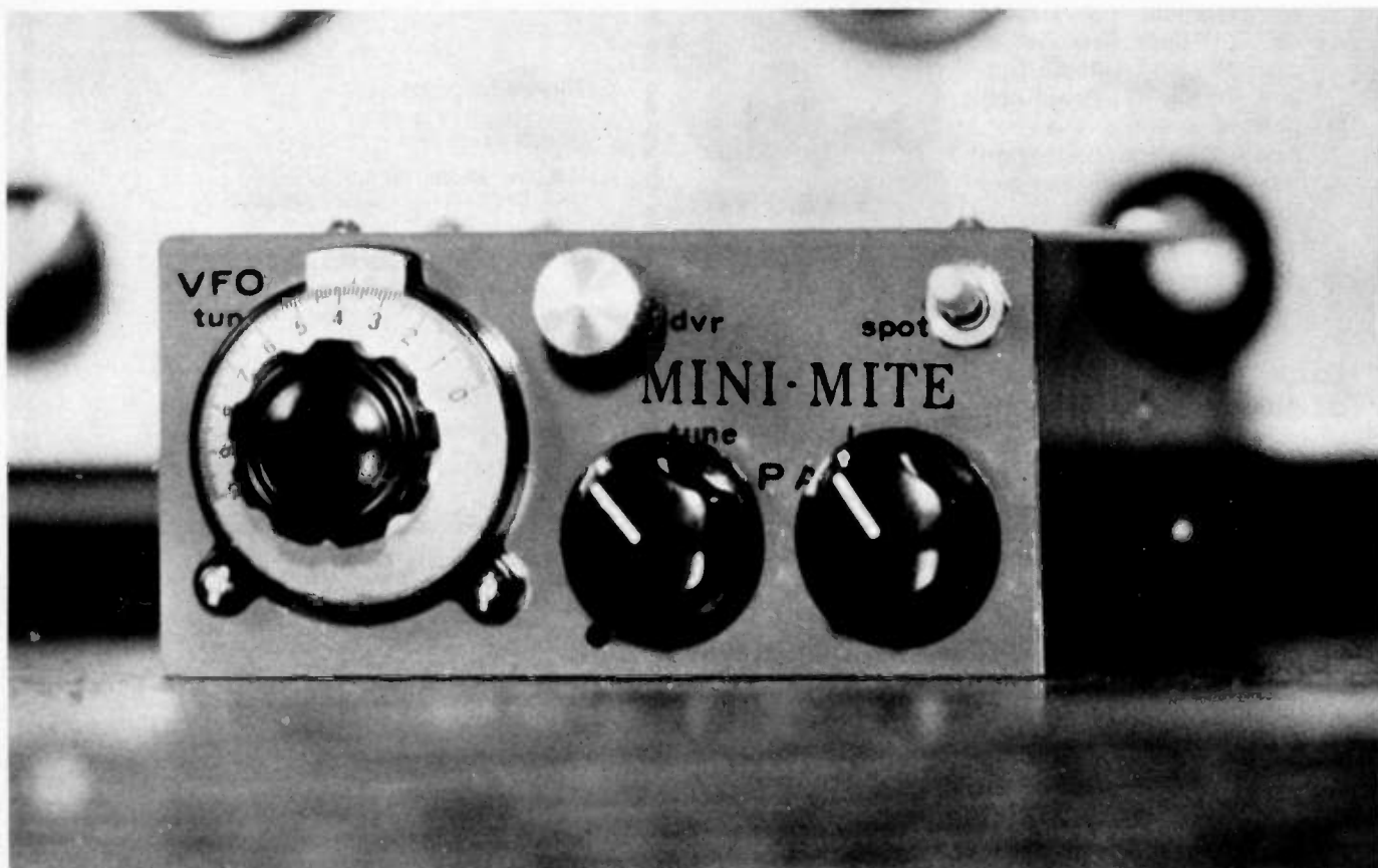
The Mini-Mite, a "kilowatt" among QRP rigs, runs 7 Watts peak power for cutting through the QRM and clearing the frequency for the little QRP rigs.
