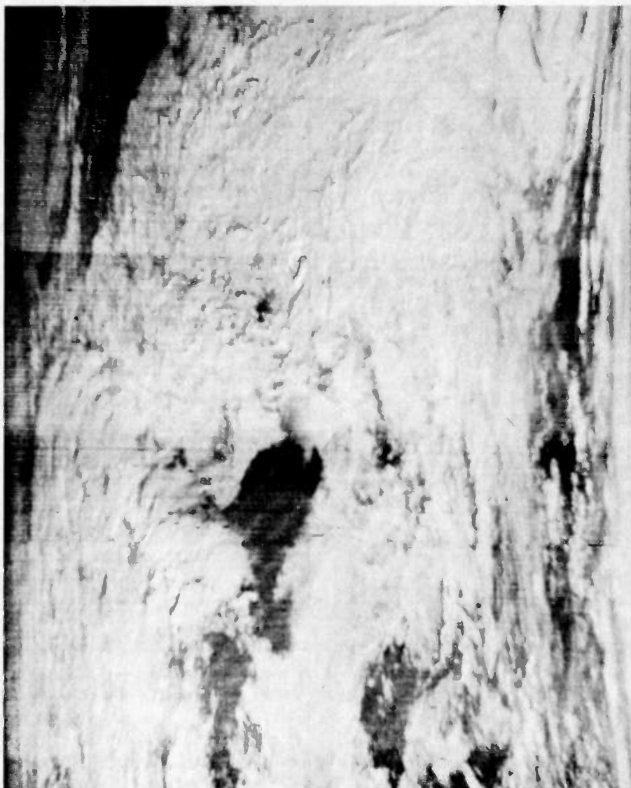
Photo 7. One drawback in improperly operated CRT display systems is that trace “blooming” often obscures fine features in very bright clouds. This photo of a NOAA pass over the central U.S. on a very cloudy winter day shows that properly operated CRT systems need not have this problem. This particular picture was displayed on the 5” CRT monitor described in reference (19).
