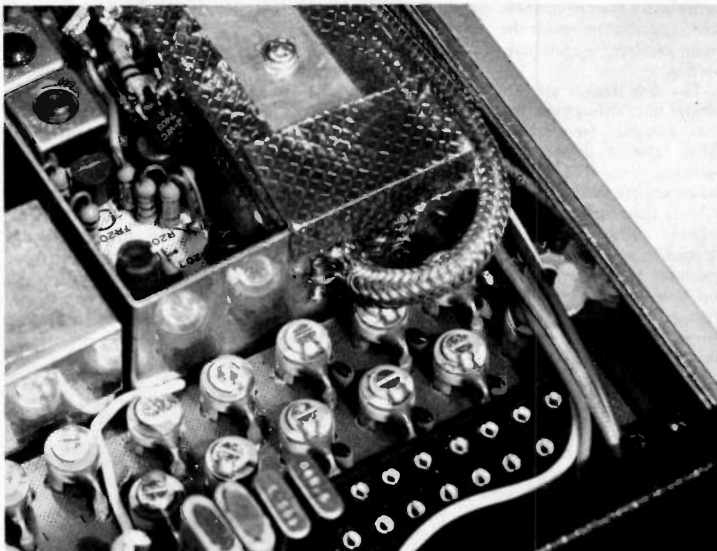
Front right view of the transceiver with the top cover removed, showing the receive coax cable entry into the rf compartment. Note that the outer braid is soldered to the outer wall of the compartment.
