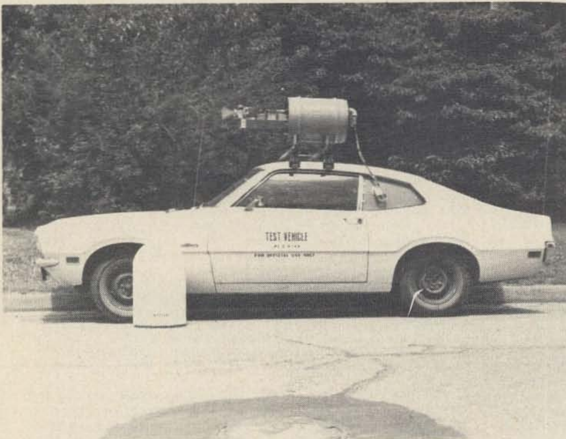
Here is a photograph of the 3cm mobile amateur rig presently being operated by WA4WDL. It has receivers for 10cm and 3cm along with a solid state transmitter for 3cm. It has a doppler radar system for anti-collision research and has the capability of legally confusing police radar units!
