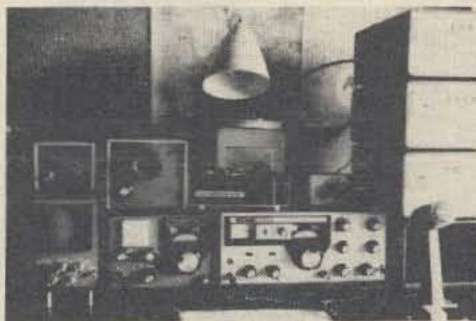
Shack layout of JA0BZC. The SSTV gear at the left and all the other equipment besides the FT-200 is homebrew.
