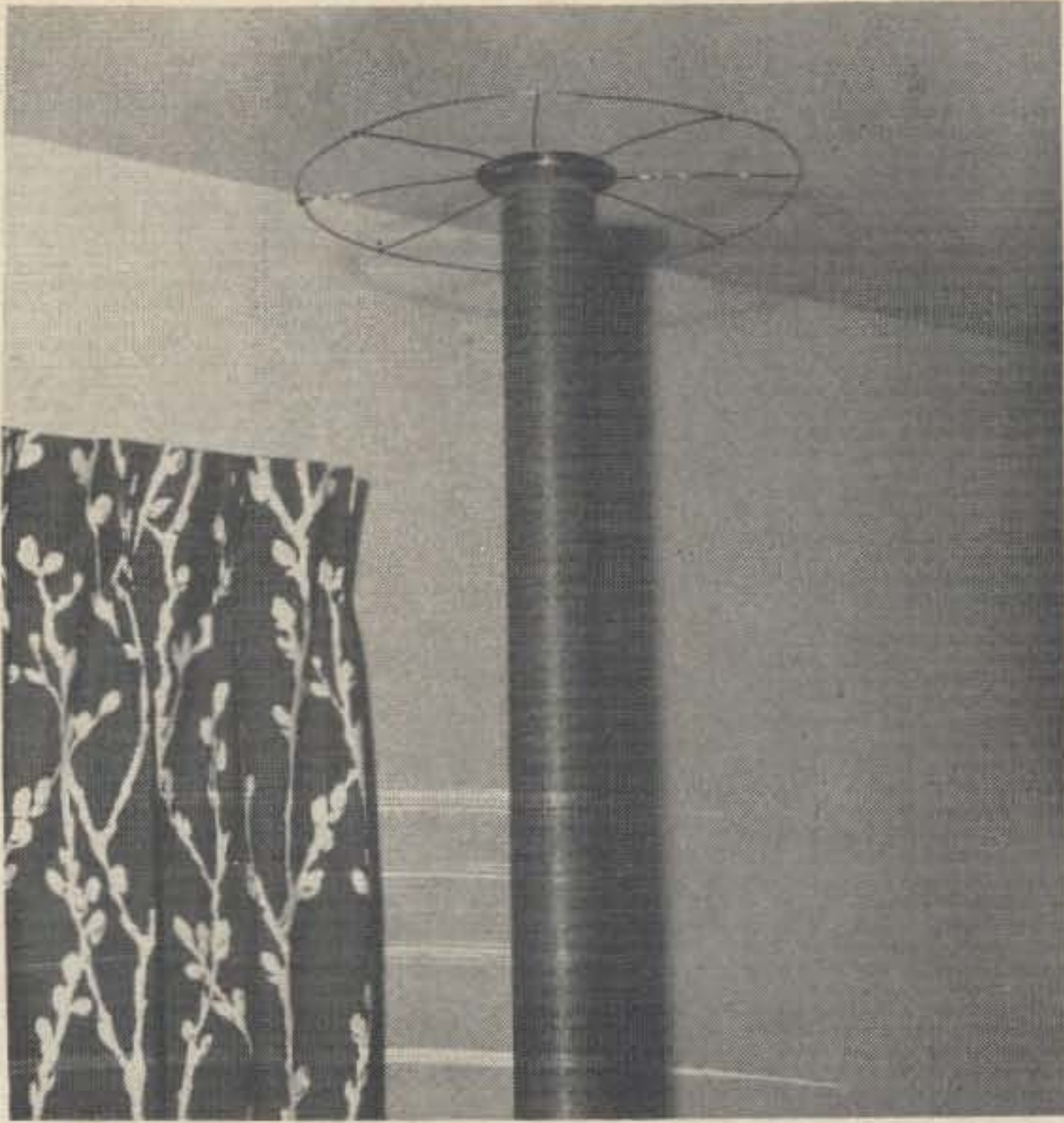
This particular model almost reaches the ceiling of the shack. A wire capacity hat was added to increase the effective height and bring more rf current up the coil.
