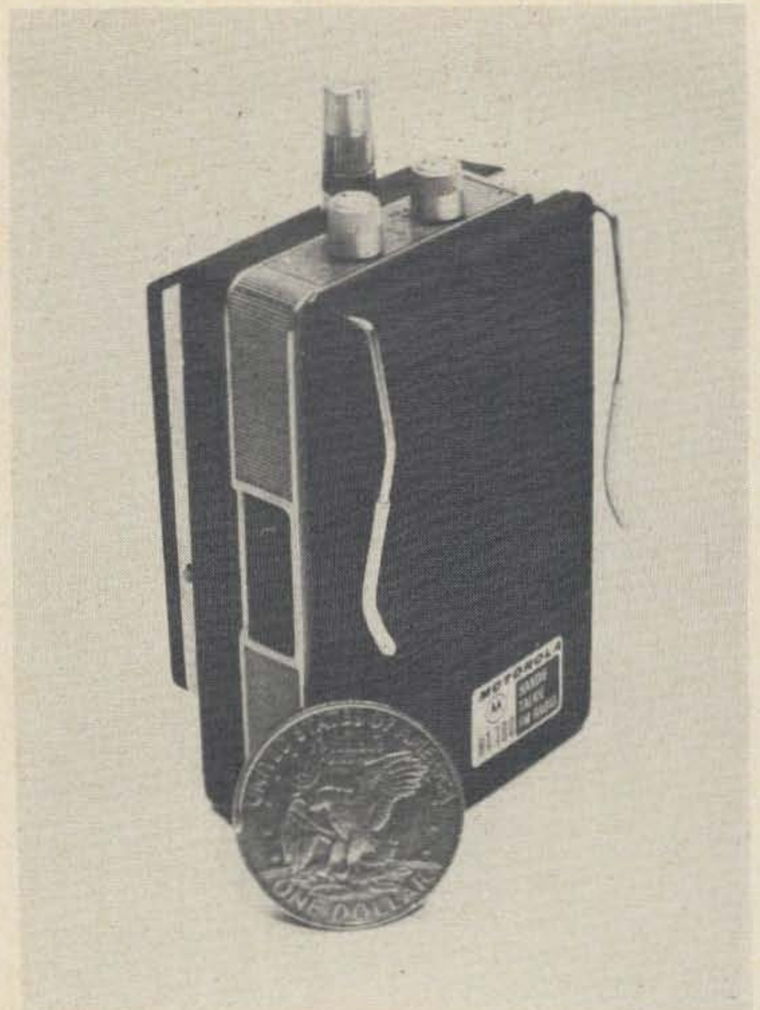
A belt clip fashioned from modified hair curler springs. The springs are epoxied into small holes drilled into the panel.
