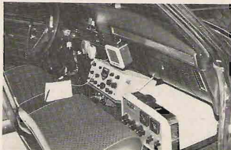
Photo. 2. The KWM-1 and SB-220 are mounted under the dash. The second mike is for the Motorola 2 meter FM fixed frequency two way radio. A common speaker is used for the KWM-1 and FM radio.
