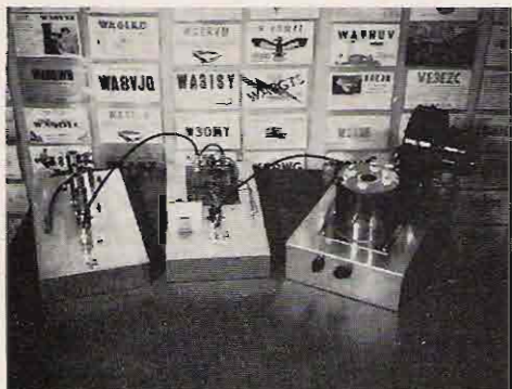
The 382 Mc oscillator chain is on the left, the 432 Mc mixer with an added buffer amplifier in the center, and a 500 watt cavity on the right.
