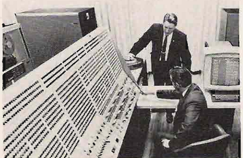
The IBM 360/195 - the largest computer in IBM's line. This machine can process an instruction in only 54 nonoseconds.
