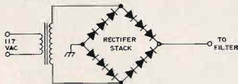
Fig. 1. Standard bridge rectifier using series silicon diodes.
