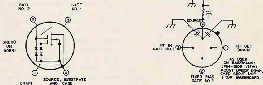
Fig. 1. The 3N200 and its connections when mounted upside down on baseboard.
