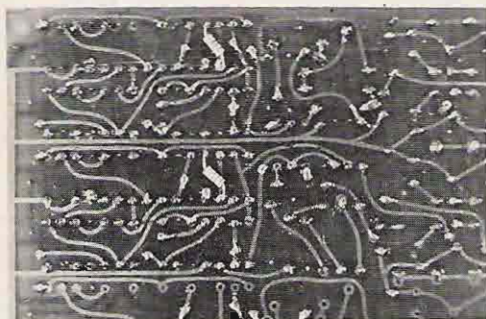
Arrangement of 1/10th watt, 2700 \Omega resistors under the board
