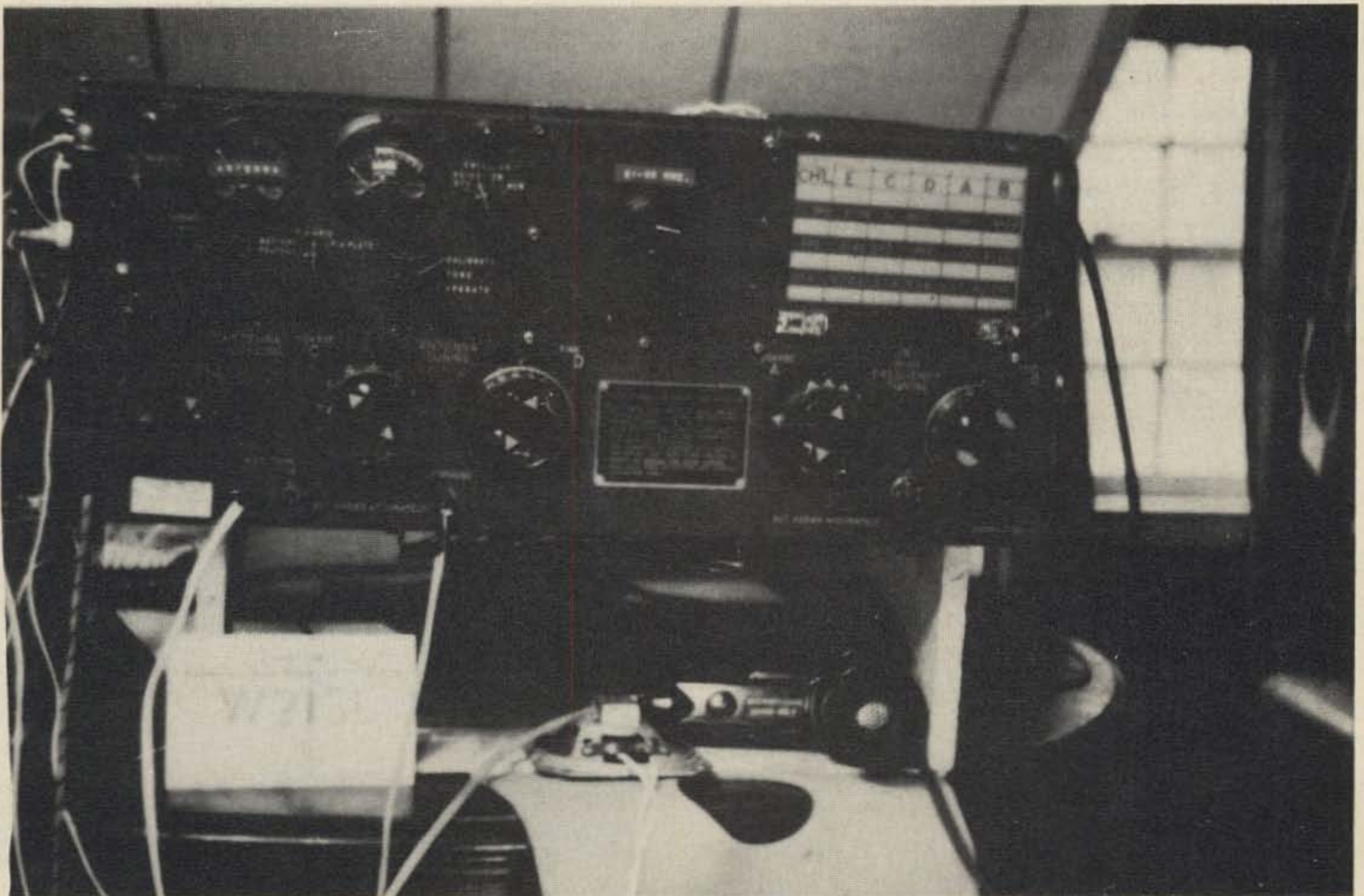
Front view of rig shows tuning knob of C3, dynamic mike, speaker for sidetone, and tuning chart.
