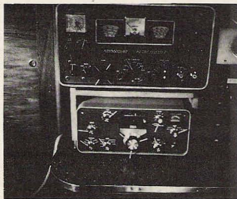
All controls "pegged" for ease of operation. Distance between knobs is a factor when choosing equipment which has to be "pegged."
