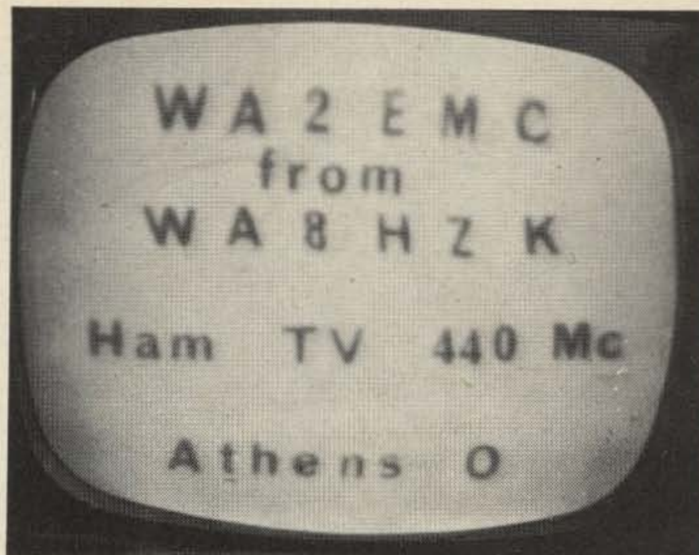
Fig. 2. Signal produced by WA8HZK/8's flying spot scanner transmitter as viewed on the receiver at his shack. The three-tube unit, designed by W2VCG, is capable of transmitting high resolution pictures of photographs and overlays, such as this identification slide.
