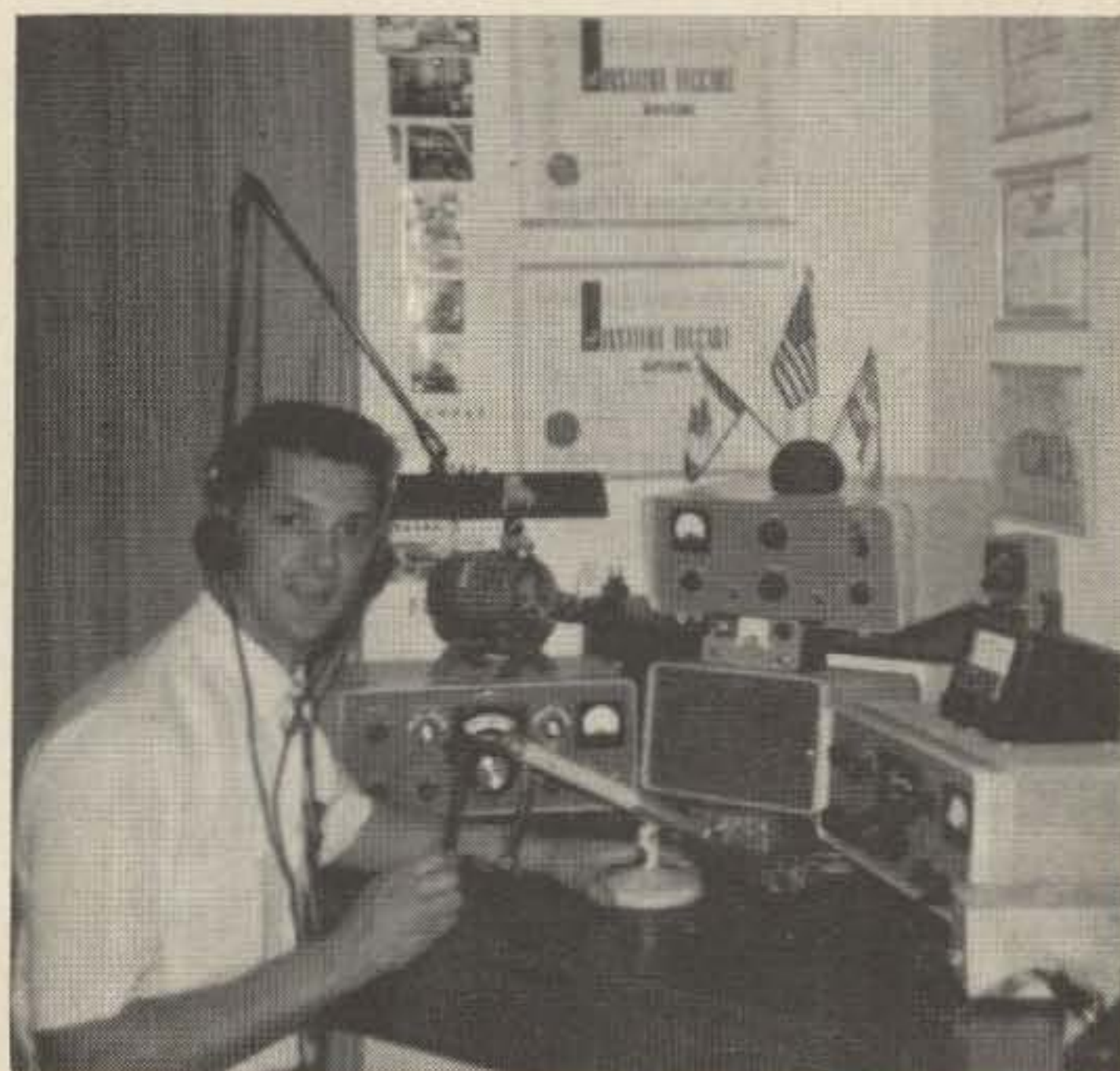
The station at VE2AES. The compactness of the linear in the center can be noted by comparing its size to the transmitter and receiver.
