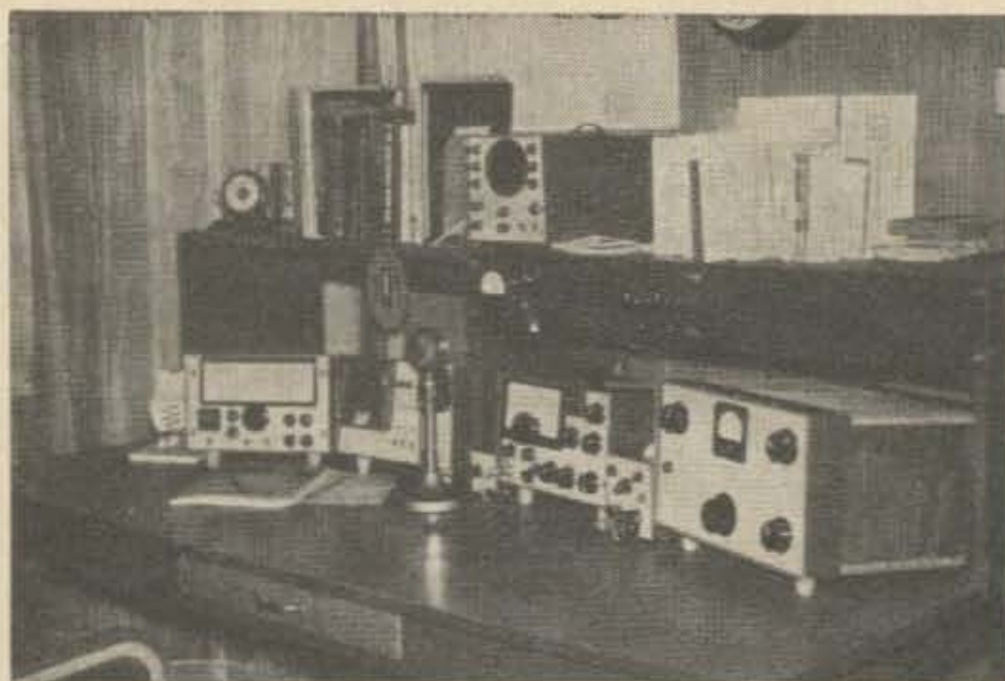
Left to right at W9DSP: All transistor receiver covering 3.5 to 30 MHz with room for 6 and 2 in the future; includes FET's. Power supply and control. 125 watt DC input transmitter; all transistor except for three tubes. Includes VOX, VFO, PTT, five bands. Solid-state electronic keyer. tube-type linear with pair of 572B's and self-contained power supply. And on the shelf, an all-solid state (except CRT) scope and RTTY terminal unit.
