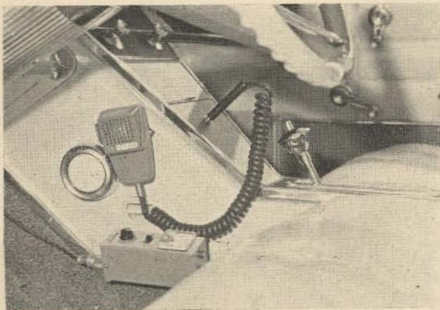
Mike and SWR bridge are installed neatly by the driver in the console.
