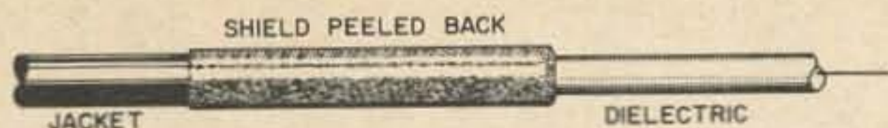
Fig. 3. Peeling the shield of RG-8/U back over the jacket makes a fine skirt—if you have a great deal of patience!
