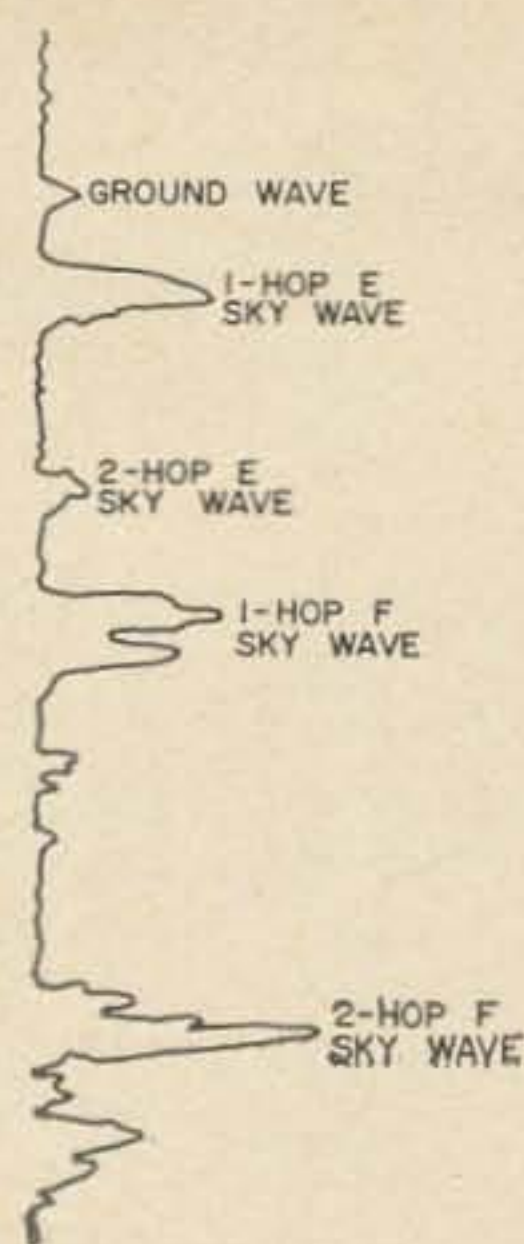
Fig. 2. Typical train of Loran pulses as they might appear during night-time hours on the navigator’s set. The ground wave, if close enough to the station, always is seen first with the various sky waves following.
