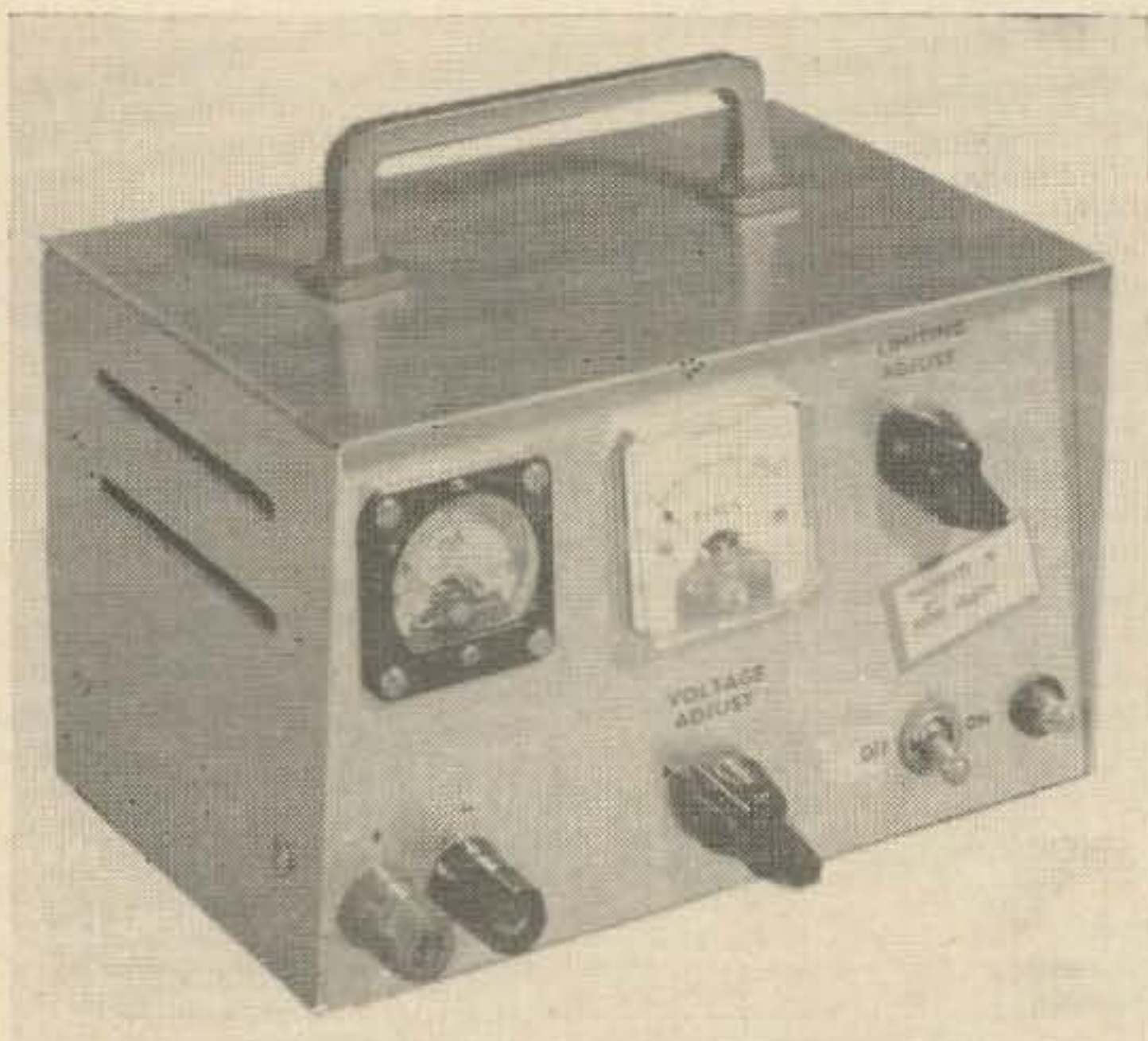
Fig. 1. Laboratory-type power supply. Q1 is a 2N375 or 2N1542A; Q2, Q3 and Q4, 2N508; CR1, 2, 3, 4, 8, 9, 10, 11, 12, 1N4002 or 1N2069; CR5 and CR6, HB5 or FD1135; CR7, 1N755 or two 1N468's in series.
