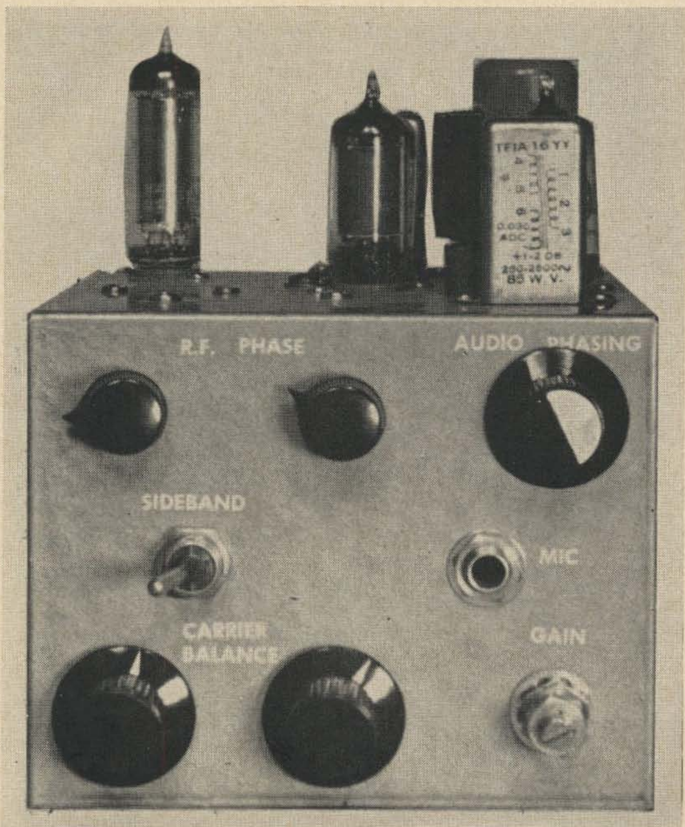
Front view of the phasing SSB exciter. The audio balance control is on the rear. Note that mic gain is a screwdriver adjusted control.
