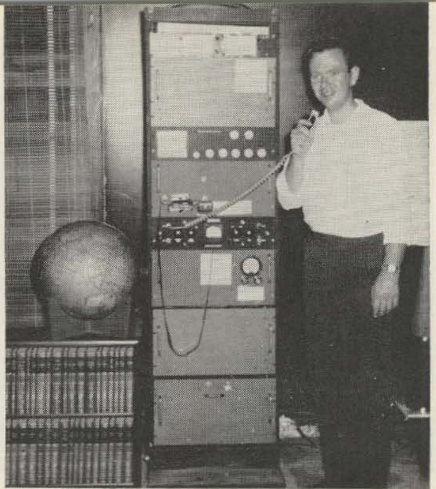
The author and the repeater. Panels, top to bottom: 1) Preselective LC tuned filter 2) Six meter receiver 3) Audio panel 4) Tape deck 5) Modulator 6) 220 mc control receiver 7) Control panel 8) Six meter Transmitter
