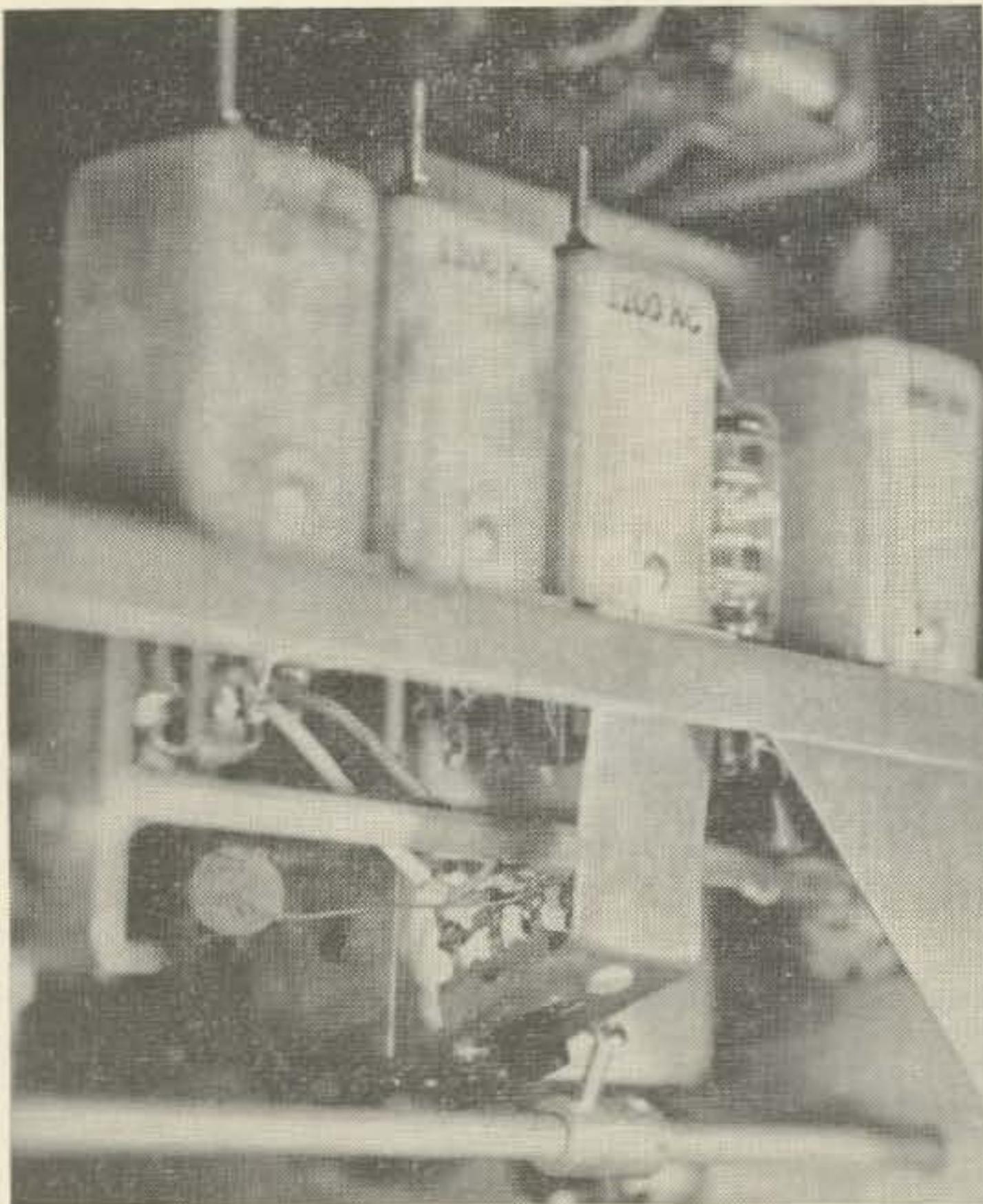
Photo 2.—A side view of the conversion showing the position of the switch, shaft coupler and mounting bracket.
