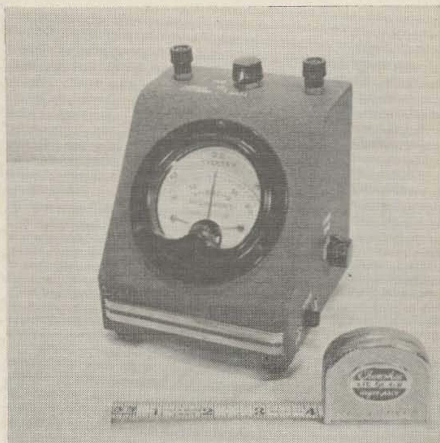
Fig. 3. The experimental wide range microammeter. The circuit fits easily into a three-inch meter case. The side of the case holds the power switch and the zero adjustment. An army surplus meter is used, removed from a teletype bias meter circuit, having a sensitivity of approximately one milliamperere each side of center.
