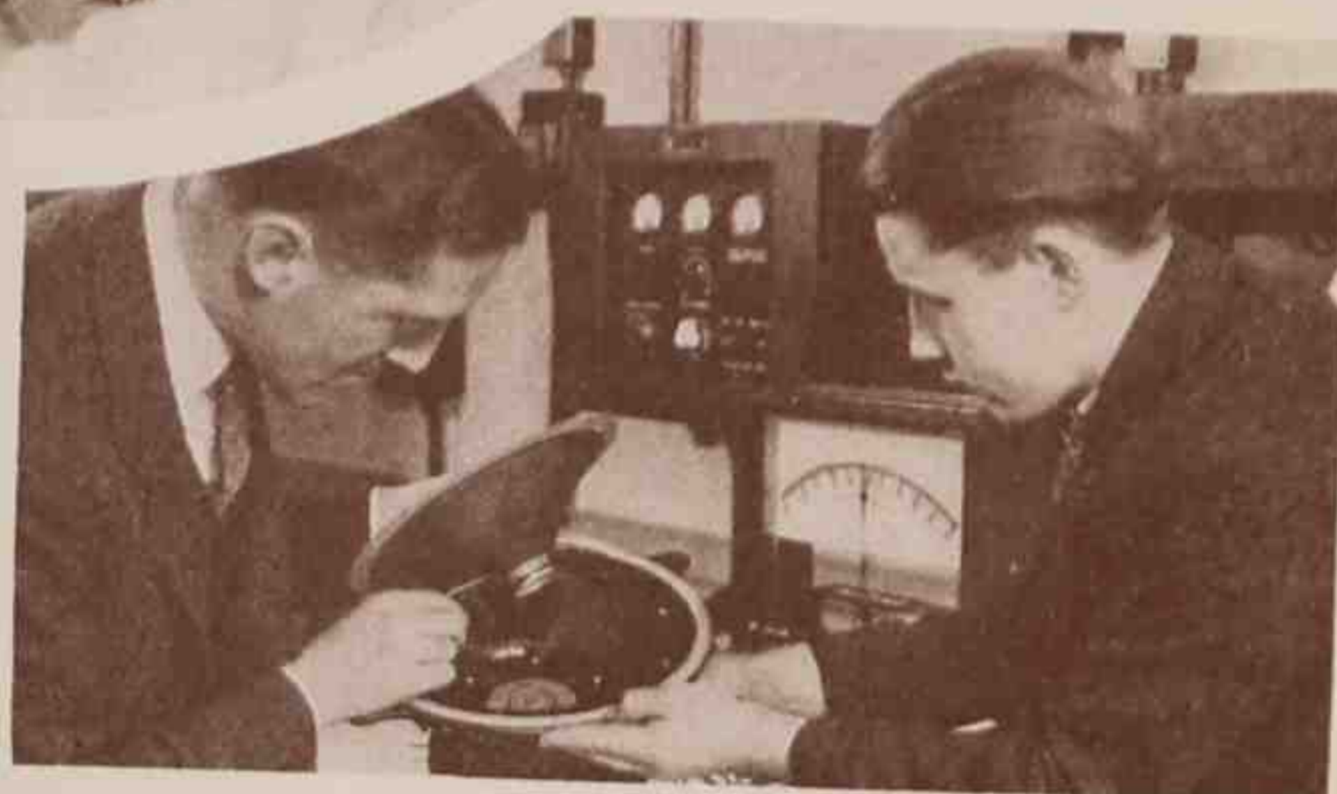
Oval—Oscillograph method of adjusting receiver circuits. Left—The assembled receiver undergoing an output test. Right—Assembling a loud speaker
