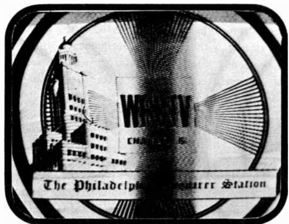
Fig. 13-7 (a) "Windshield wiper" interference from another TV station.
