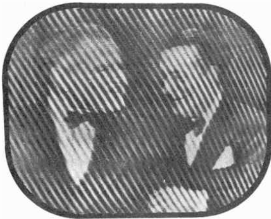
Medium strength interference caused by a neighboring receiver.
