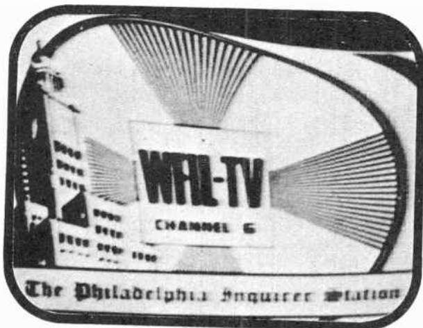
Picture pushed out of shape by the magnetic field of a PM speaker near the flare of the kinescope.
