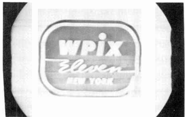
Smear Due To Ungrounded Kinescope Coating
