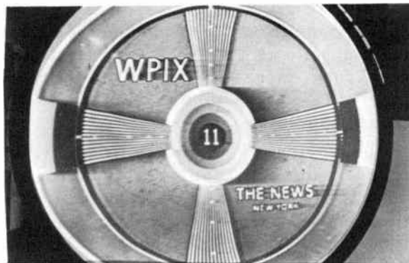
Smeared Dark Picture Due to Defective Kinescope
