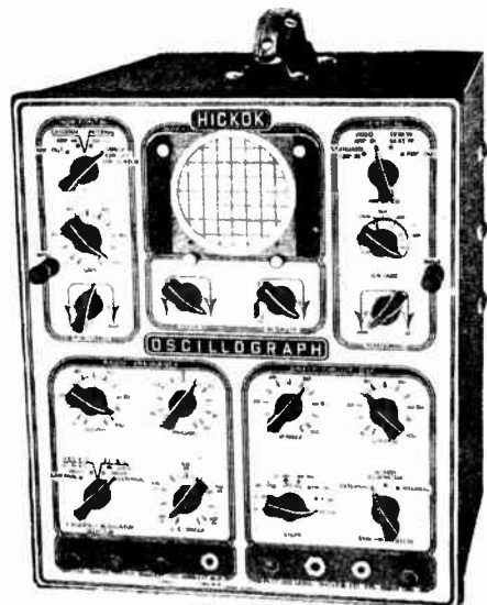
Figure 281. Most oscilloscopes employ three inch cathode ray tubes and have the required controls for adjustment to "see" signals of various types.
