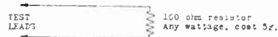
Figure 266. The presence of voltage may be observed with the aid of a resistor and test leads. This is an emergency method for locating faults and should not be used if test instruments are available.
