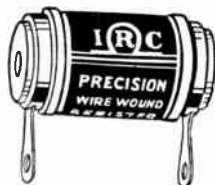
Figure 40. Certain circuits require the use of resistors of very high accuracy. A precision resistor used in meter circuits is illustrated.
