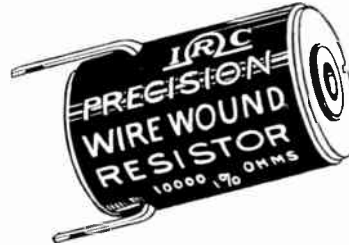
Figure 108. To increase the reading of meters, series and shunt resistors are needed. These resistors are of the precision type, usually 1% accuracy.
