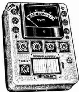
Figure 274. A tube tester with its meter scale calibrated GOOD-BAD. This permits the non-technical customer to see for himself the results of the test.
