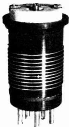
Figure 191. A short-wave plug-in coil with adjustable trimmer condenser. This coil is wound on a four-prong form, but five and six prong forms are used quite often.
