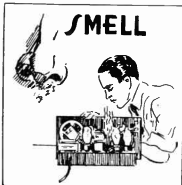
Figures 382 and 383. A smoking part will indicate a probable fault in the associated circuit. Touching the grid caps and other sensitive points will produce results which may suggest the stage or part at fault.
