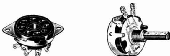
Figure 15. It is interesting to note that tube sockets may be mounted with bolts or rivets. A volume control is usually mounted by means of the threaded section around the shaft.
