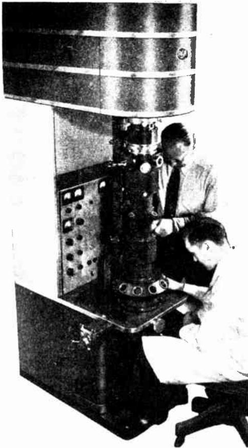
Figure 359. A complete view of an RCA electron microscope in application. Notice the six observation windows.
