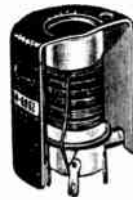
Figure 11. Radio coils are housed in metal cans.
