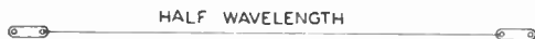
Figure 249. Diagram showing a simple half-wave antenna or dipole. Regardless of how power is fed to the dipole from the transmitter, it always has the same characteristics. For maximum radiation, it must be cut to exactly the right length.
