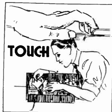
Figures 382 and 383. A smoking part will indicate a probable fault in the associated circuit. Touching the grid caps and other sensitive points will produce results which may suggest the stage or part at fault.
