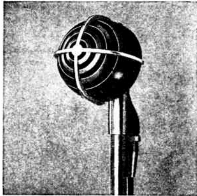
Figure 153. Crystal microphones are commonly used for public address and broadcasting requirements. The microphone itself is mounted on a desk or floor stand.
