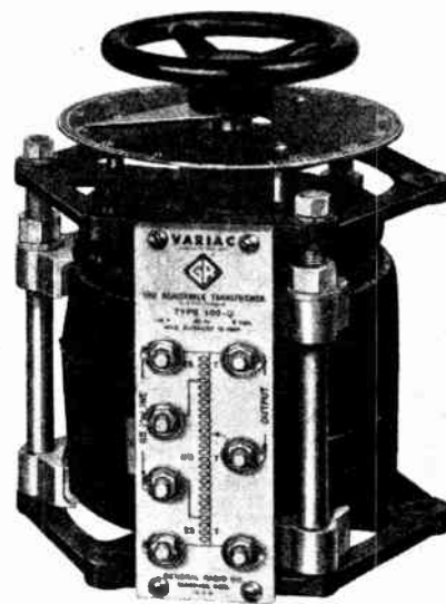
Figure 88. As you can see from the terminal panel of this Variac type transformer, the tap of the auto-transformer can be changed by rotating the handle and any voltage from zero to maximum can be obtained. The efficiency of a Variac is almost the same for all settings.
