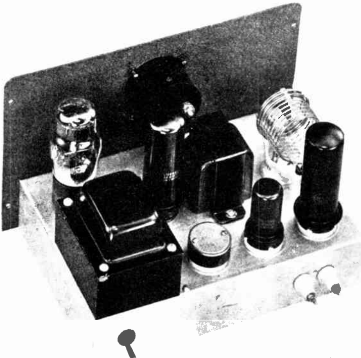
Figure 237. Inside, top view of a two-stage modulated transmitter. See if you can find the corresponding parts in the schematic diagram.
