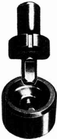
Figure 21. This type of socket punch is employed by radio servicemen and in experimental laboratories for punching the required cut-outs for tube sockets.
