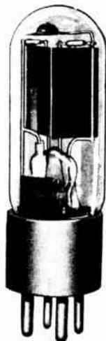
Figure 126. This is an illustration of a photo-cell used in motion picture sound equipment. The large plate is the cathode, the center wire is the anode.
