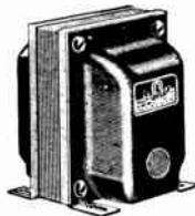
Figure 78. Transformers used with low (power or audio) frequencies have iron cores. The illustration shows an upright type power transformer used in radio sets. Wire leads come out of the bottom. The transformer is bolted to the chassis and the wire leads go through an opening in the chassis.
