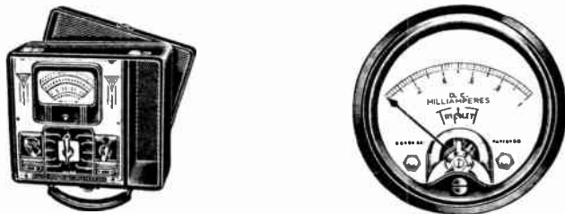
Figure 106. Meters, used individually or in radio test equipment, depend on magnetic effects for their operation.
