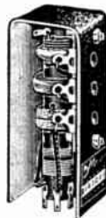
Figure 85. A multi-band coil combines several coils in a single shield. Small trimmer condensers for each band are also included in the shield. In some radio sets, each coil is individually shielded and the trimmers are placed outside of the shield.
