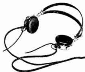
Figure 164. Head phones are employed to convert electrical energy at audio frequencies to corresponding acoustical (sound) energy.
