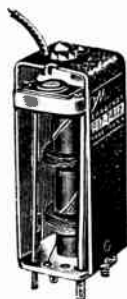
Figure 83. An inside view of an I.F. transformer. The primary and secondary coils are mounted on a wood rod, and are spaced apart. The two trimmer condensers are mounted at the top of the shield.
