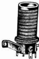
Figure 79. The antenna coil illustrated is a transformer used for radio frequencies. An air core is used and the wire is wound on insulated tubing. Connections are made to lugs.
