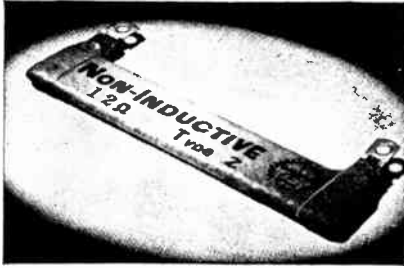
Wire-wound resistors, using cylindrical cores, have considerable self-inductance which is not permissible in some circuits. If the resistance wire is wound in a special way on flat strips, the units will have almost no inductance.
