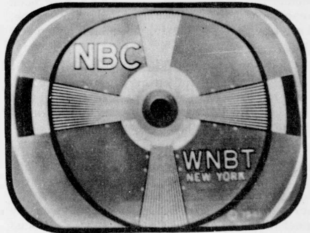
Fig. 132. Vertical Linearity Control Misadjusted
