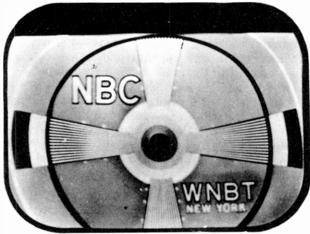
Fig. 129. Vertical Centering Control Misadjusted
