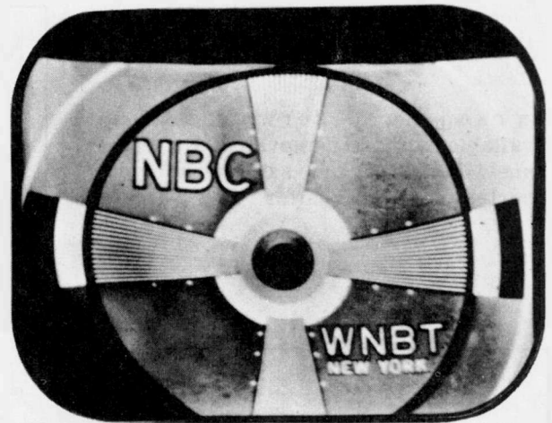
Fig. 117. Focus Coil and Ion Trap Misaligned
