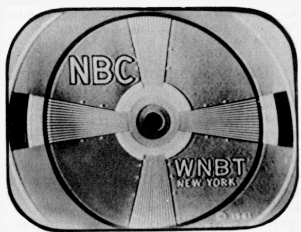
Fig. 230. A Station Test Pattern Showing the Effect Due to either Transient Oscillation or a Reversed Polarity Smear. (See Figure 229C.) Photo Courtesy National Broadcasting Company and the R. C. A. Service Company, Inc.
