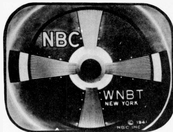
Fig. 242. Station Test Pattern Showing the Effect of Misadjustment of the Contrast Control. Photo Courtesy National Broadcasting Company and the R. C. A. Service Company, Inc.
