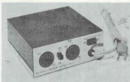
FIG. 47. A power supply designed to be used with a preamplifier.
