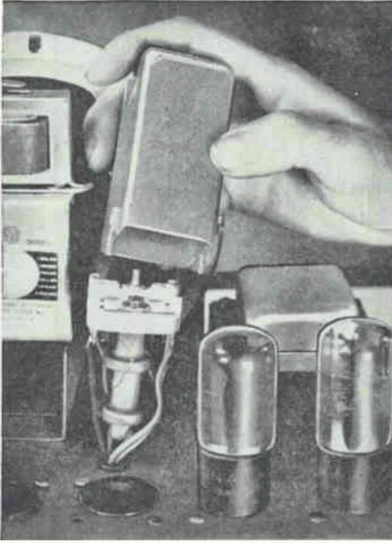
FIG. 14. This is what you see inside the i. f. transformer when you lift the metal shield can.
