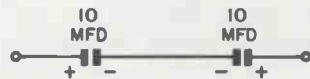
FIG. 59. Two 10-mfd electrolytics connected "back-to-back" for use as 5 mfd in a cross-over network.
