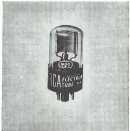
FIG. 6. Diode phototube with octal base (vacuum).
