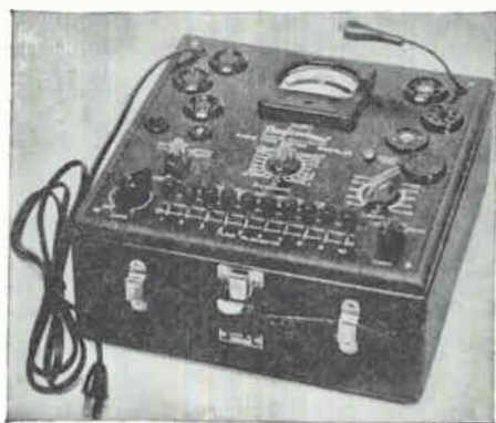
FIG. 10. Radio men use tube testers like this to test tubes.
