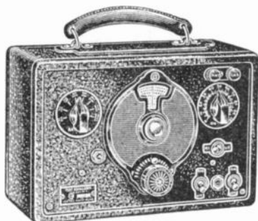
A Typical Test Oscillator—RCA Model TMV 197-C, with 90 to 25,000 kc. R.F. frequency range and 400 cycle audio output signal.
