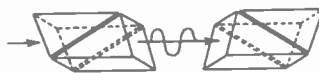
FIG. 30B. When two Nicol prisms are arranged like this, no light can pass through the combination. The polarized light coming out of the first prism is totally reflected by the second prism. If the second prism is rotated 90^\circ , polarized light will pass through.
