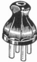
Type of plug attached to speaker cable which usually has 4 or 5 prongs. They plug into a 4 or 5 prong socket situated on the chassis.
