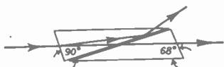
FIG. 30A. Cross-section of a Nicol prism, showing how the incident beam is split into two beams by refraction, one beam being reflected at the Canada balsam layer which separates the two sections of the prism, and the other beam being transmitted through this layer.
