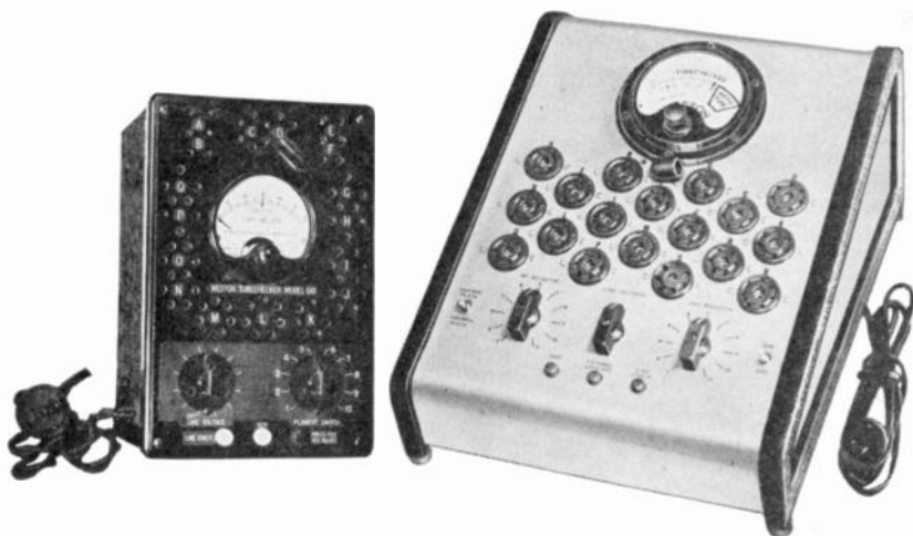
Weston Model 674 Counter Tube Checker, employing a group of sockets for similar tubes, a combination switch gear and plate voltage selector and a filament voltage selector. This checker has an "english" reading scale and has incorporated a cathode leakage test.
