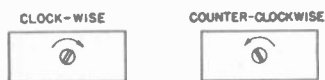
FIG. 7. Turning a trimmer condenser screw clockwise usually increases the capacity, decreasing the frequency of the resonant circuit. Turning a trimmer condenser counter-clockwise usually decreases the capacity, increasing the frequency of the resonant circuit.
