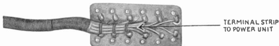
Type of terminal strips used to connect RF-detector chassis to power pack A.F. chassis when built separately. Bolt and nut system usually found on power pack chassis.
