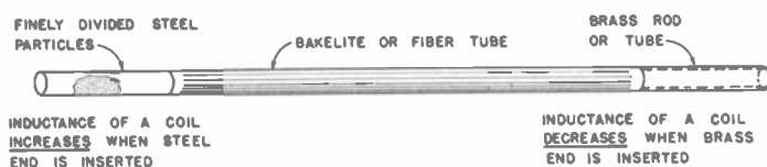
FIG. 2. The "tuning wand," construction of which is shown here, is used to make a positive check-up on the need for alignment in a super, as well as to tell how to adjust the preselector-mixer-oscillator alignment condensers.
