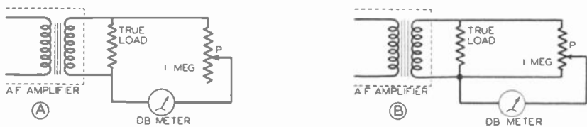
FIG. 9. Two methods of connecting a db meter to measure variations in db level directly regardless of what the output level is.
