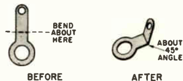
Fig. 14. Before you mount the solder lug, bend it as shown here.
