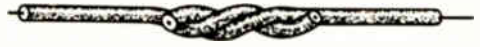
Fig. 16-2. How to make a dummy open part with two pieces of wire.
