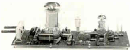
Fig. 24. Phenolic side of an etched circuit board with the parts installed.
