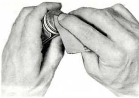
Fig. 44. How to clean the center of the bottom of a flashlight cell with a piece of sandpaper.
