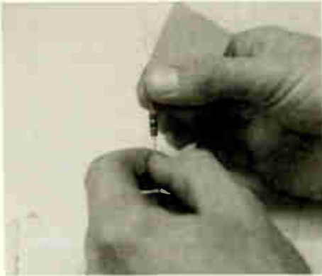
Fig. 16. Using sandpaper to clean a lead.
