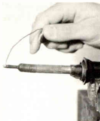
Fig. 9. How to apply solder to tin the tip of the iron.
