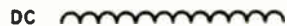
Fig. 18. Only a small ripple will be noticeable in the output of a dc generator having 6 coils and 12 commutator sections.
