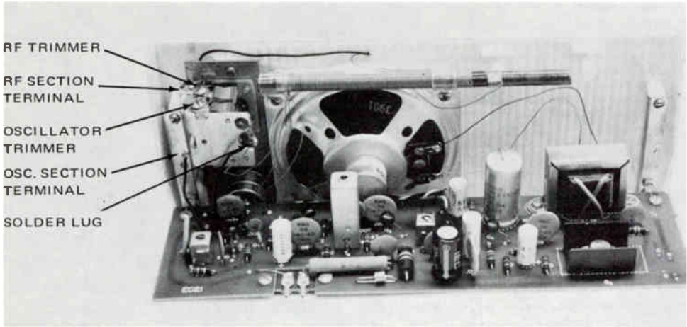
Fig. 16. Top view of receiver with wiring completed.
