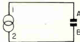
Fig. 17. A capacitor connected across a generator.
