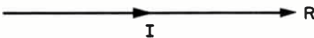
Fig. 26. The voltage across a resistor is in phase with the current, so the vector for the resistor voltage is drawn on top of the current vector.
