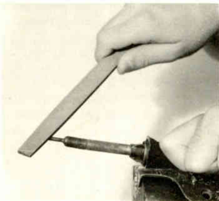
Fig. 5. To file the tip of your iron, hold it against a vise as shown here.
