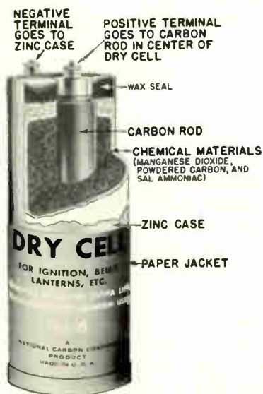
Fig. 1. Construction of a dry cell.
