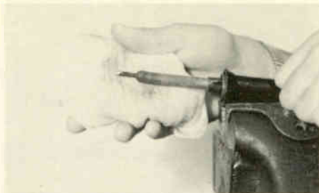
Fig. 10. Wiping excess solder from the iron with a piece of cloth.
