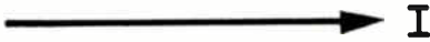
Fig. 25. The current vector is drawn horizontally and used as a reference point for the other vectors.
