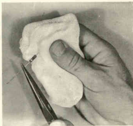
Fig. 1-7. Removing the excessive solder from a resistor lead.
