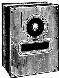
FIG. 15. Jensen Peridynamic loudspeaker unit. Reinforcing bass notes emerge from the rectangular opening below the cone.
