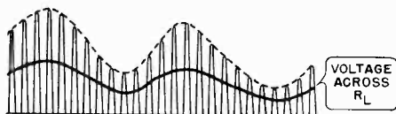
FIG. 8. How the voltage across R_L follows the average of the rectified pulses when the plate resistance of the circuit in Fig. 7 is high.
