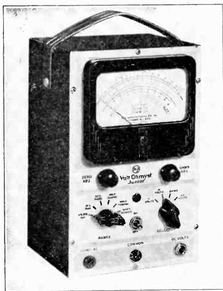
FIG. 11. The RCA-Rider Volt-Ohmyst Jr. is a typical d.c. type v.t.v.m. using the balanced bridge circuit.
