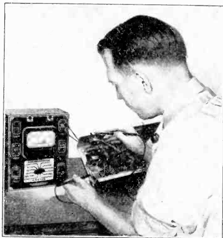
Serviceman using a d.c. voltmeter to check the plate voltages of tubes in a defective receiver. A few simple measurements with meters are often enough to locate a defective part.
