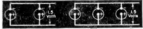
FIG. 20. Parallel connections of dry cells. Remember that when cells are connected together in parallel, the voltage is that of one cell, but the current-furnishing ability is increased.
