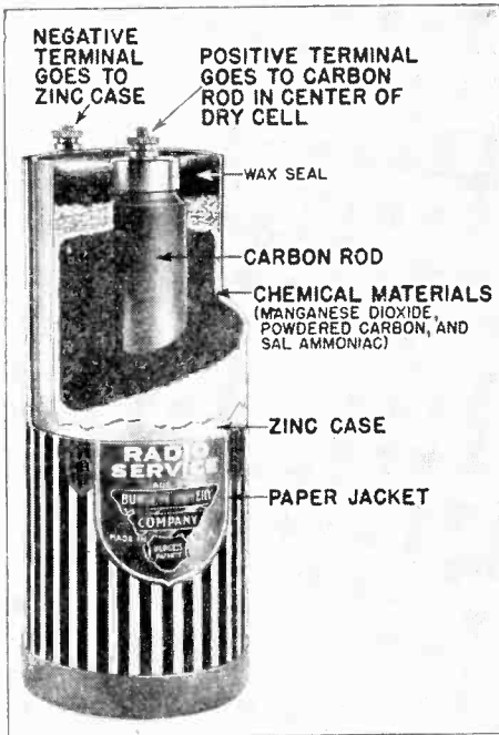
FIG. 17. Construction of a standard dry cell.
