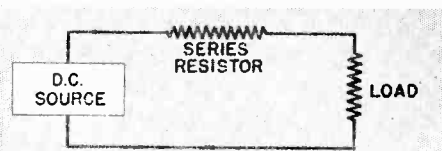
FIG. 5. Basic radio circuit in which the source voltage is too high for the load.
