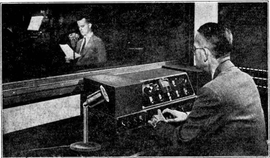
FIG. 5. The monitor man in the control room watches the performers in the studio through a large glass window as he "rides gain." The small microphone at the left of the control unit is used principally for intercommunication between the monitor room and studio prior to a broadcast or during rehearsals, for the wall between the two rooms is sound-proof.
