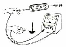
A Voltmeter in Series With a Capacitor and Connected Between B+ and Ground Gives a Reliable Check for Leaky Capacitors.
