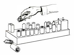
In Tube-Type Receivers, Most Troubles are Repaired by Replacing a Defective Tube.
