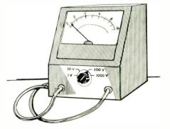
The Highest Meter Range Giving a Readable Deflection Provides the Most Accurate Voltage Readings.
