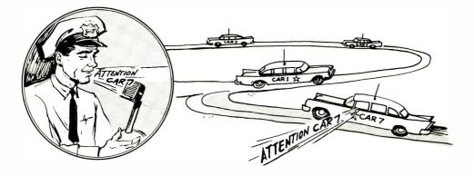
Quik-Call Radio Provides Selectivity Within a System: One Car may be Called Separately--the Remaining Vehicles in the System are Silent.
