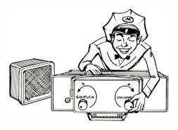
A Quick Check On Receiver Operation is Made by Turning the Volume Full-On and Opening the Squelch.
