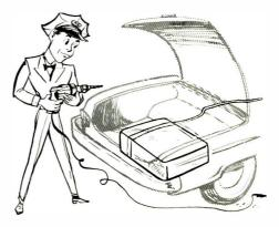
Be Sure to Avoid the Gas Tank, Gas Line and Similar Parts of a Vehicle when Drilling Holes and Mounting Two-Way Radio Equipment.
