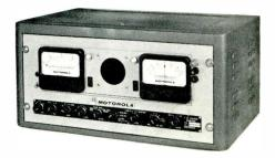
The Motorola Monitor Measures Both Frequency and Deviation.
