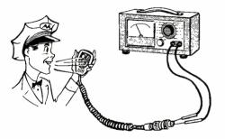
Establishing the Amount of Mike Voltage--As Measured on a Sensitive AC Voltmeter--is Helpful in Diagnosing Modulation Problems.
