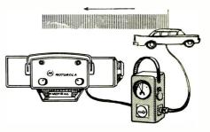
If a Thruline Output Meter is Used, the Transmission Line Should Terminate into the Antenna.
