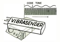
The Vibrasender Insures that the Correct Coding Tone Modulates the Transmitter and Reaches the Receiver.
