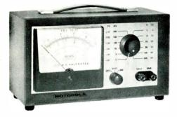
The Motorola Transistorized AC Voltmeter Will Measure Small AC Voltages Accurately and is Very Useful in Trouble Shooting Low Level Audio Circuits.
