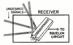
At the Private Line Receiver, Undesired Signals Cannot Operate the Vibrasponder and Cause the Squelch to Open.
