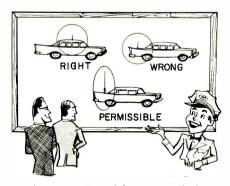
Wherever Possible the Mobile Antenna Should be on the Roof Top. Long (Lo Band) Antennas may be Mounted on a Fender if Necessary.
