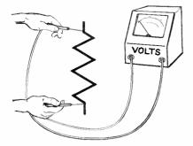
Voltage Measurements are Always Made by Placing the Voltmeter in Parallel with the Unit Being Tested.
