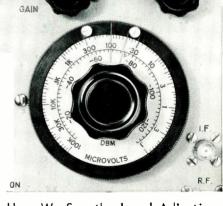
Here We See the Level Adjusting Dial of the Signal Generator. The Setting Accurately Indicates the Generator Output Voltage.
