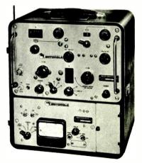
This Portable Motorola Meter Accurately Measures the Frequency and Deviation of Transmitters. between 20 and 100 MC
