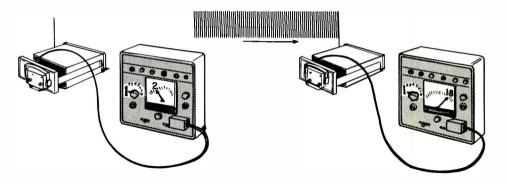
Comparing Meter Readings With and Without a Channel Signal is Very Helpful in Trouble Shooting the Receiver.
