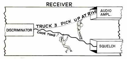
Inside the Receiver the Code Tone is Separated from the Message and Applied to the Squelch Circuit. The Correct Code Tone Causes the Squelch to Open, and the Message Reaches the Speaker.
