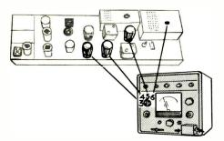
Test Set Measurements Help to Quickly Isolate "Low Output" Trouble to a Specific Stage of the Transmitter.
