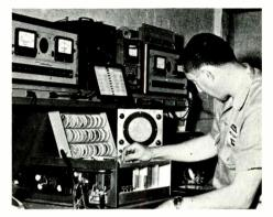
Besides Measuring Transmitter Frequency and Deviation, the Motorola Frequency Meter may be used as a Generator for "Nettina" Receivers.
