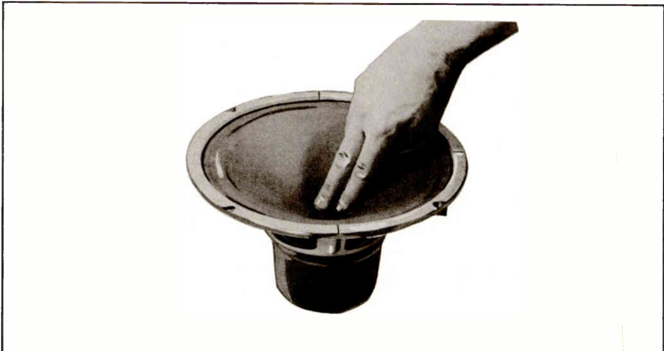
Fig. 25. Testing for a "Frozen" Voice Coil.
