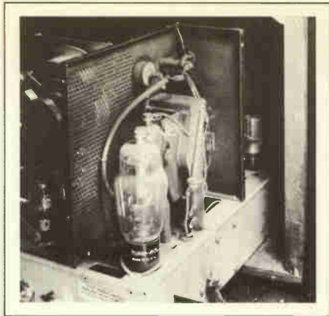
Fig. 28. Cover removed from high-voltage compartment reveals horizontal transformer and tubes.
