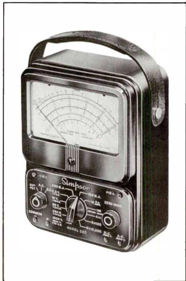
Fig. 17. A Multimeter Showing Ohms Scales and Zero Adjustments. (Courtesy Simpson Electric Co.)
