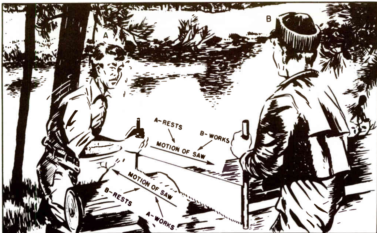
Fig. 7. Push-Pull Applied to Timber Cutting. The Lumberjacks Can Each Take a Rest While the Other is Pulling the Saw. Push-Pull Amplifier Systems Operate in a Similar Manner.
