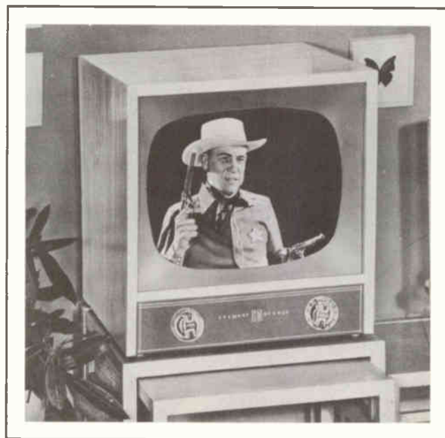
Figure 19. Good reproduction of Vertical Detail makes it possible to sharply outline edges of actor's hat. (Courtesy Stewart-Warner.)
