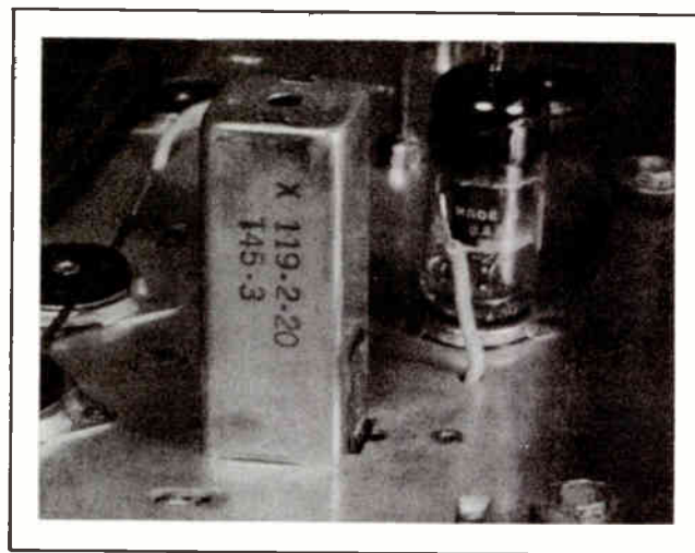
Fig. 14. Can-enclosed I-F transformer mounted on top of chassis.
