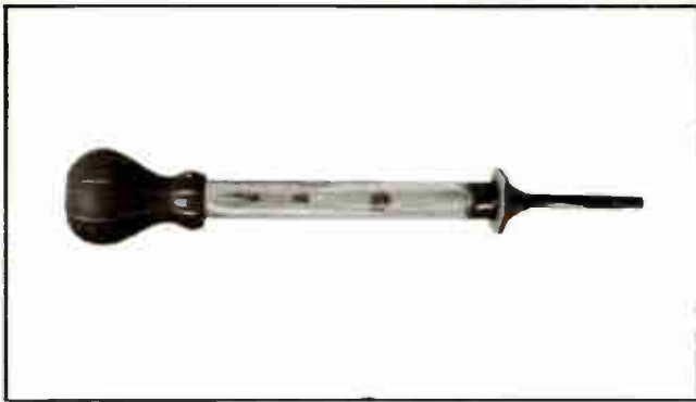
Fig. 18. A Hydrometer Used for Checking the Conditions of Storage Batteries.
