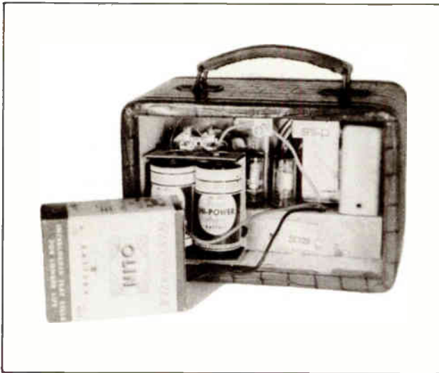
Fig. 11. Note the Absence of Power Cord in this Battery Portable.
