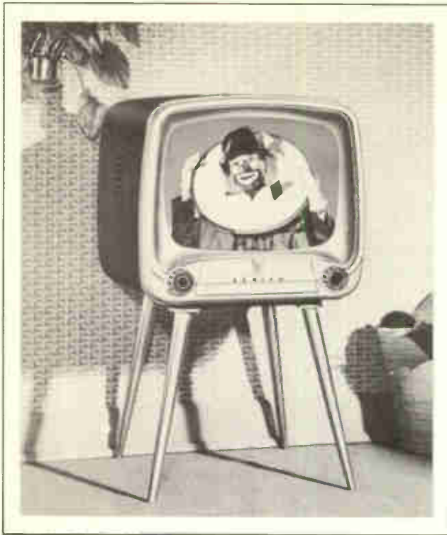
Figure 3. Circular Objects in a picture can be used to check the Aspect Ratio. (Courtesy Zenith.)
