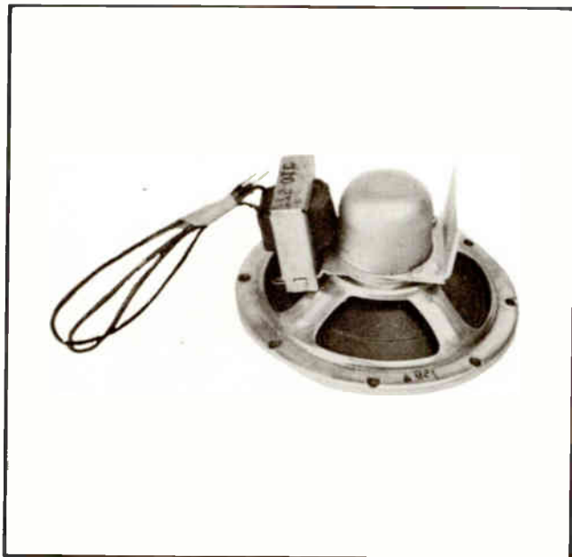
Fig. 7. Output Transformer Mounted on the Speaker.
