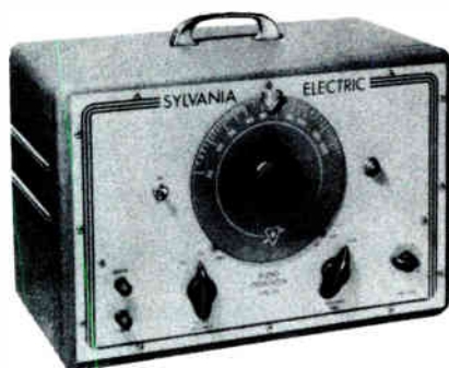
When disturbance tests fail to isolate the defective stage, an audio oscillator may be employed to check a-f and v-f circuits by the signal substitution method.
