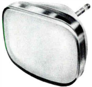
A 21-inch rectangular picture tube of the self-focusing type. With roster and sound present, loss of picture may be due to a defect in the picture tube circuits, or in the tube itself.
