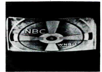
4. INSUFFICIENT VERTICAL HEIGHT H
