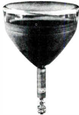
The 10BP4 picture tube provides a small screen with electromagnetic deflection.
