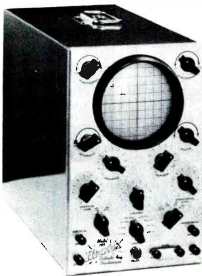
Service cathode ray oscilloscopes are useful for checking the wave-forms of the sync pulse and deflection voltages in the circuits of a television receiver.
