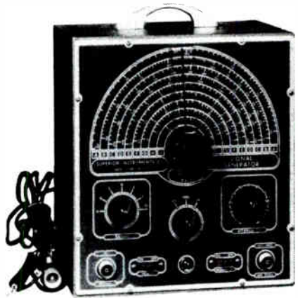
R-f signal generator of the type employed for aligning tuned circuits in radios and other electron equipment.
