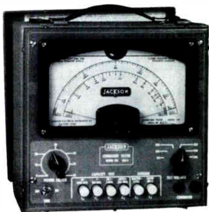
The "Condenser Tester" is a useful test instrument and often is added to the essential shop equipment.
