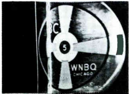
TSM-6 24. HORIZONTAL FOLD-OVER FIGURE 11
