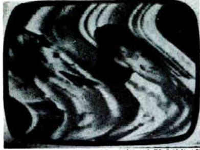
COURTESY RADIO AND TELEVISION NEWS PICTURE PULLING FIGURE 18
