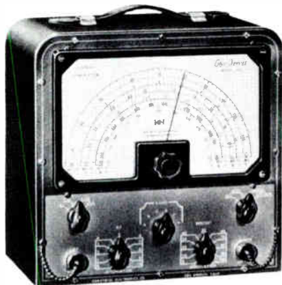
An r-f generator is needed for checking r-f and i-f stages by signal substitution. This generator provides modulated or unmodulated r-f output over a total range from 170 kc to 124 mc.
