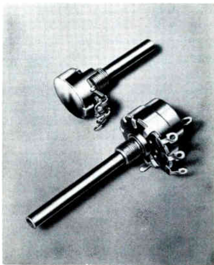
Potentiometers of the types used as volume controls in receiver a-f circuits. Noise produced in the speaker when the volume control is adjusted generally is due to dirt which has collected inside the control.
