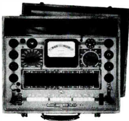
One of the first steps in a troubleshooting routine consists of checking the tubes either in a tube tester, such as the unit shown, or by replacement with known good tubes.
