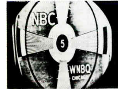
3. INSUFFICIENT HORIZONTAL WIDTH. EXCESSIVE VERTICAL HEIGHT. C
