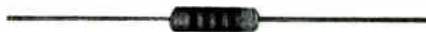
A small ceramic capacitor of the type used in high frequency circuits.
