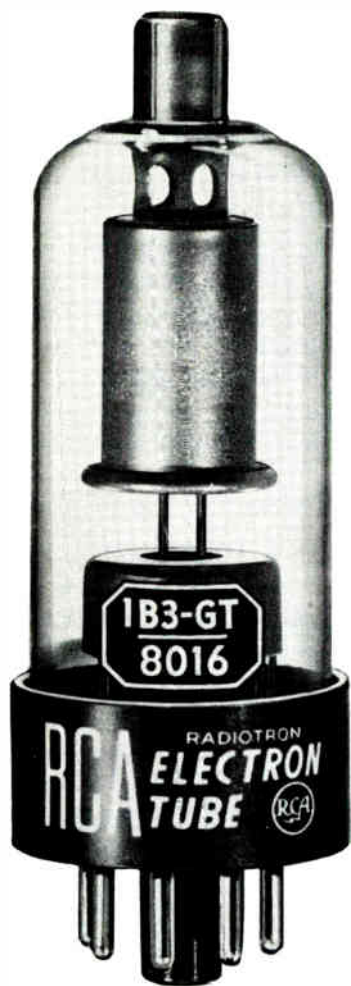
Rectifier tube of the type most employed in the flyback H.V. supply of television receivers. When this tube is defective, no voltage is applied to the second anode of the picture tube, and consequently no raster appears on the screen.
