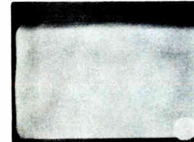
COURTESY RADIO AND TELEVISION NEWS RASTER PULLING FIGURE 12
