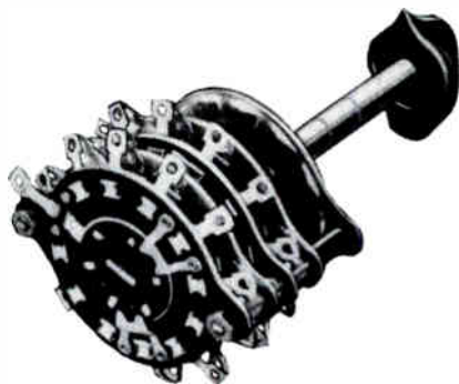
Three-deck band selector switch. Corrosion forming between the individual contacts and the contact ring is frequently the cause of intermittent operation.
