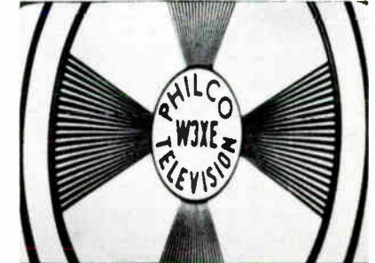
COURTESY PHILCO CORPORATION EXCESSIVE HEIGHT D
