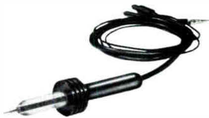
The high voltage probe is designed to permit readings with the service type voltmeter. Note the heavy insulation and safety flanges for protection of the serviceman. The multiplier resistor is visible inside the plastic tube near the tip.
