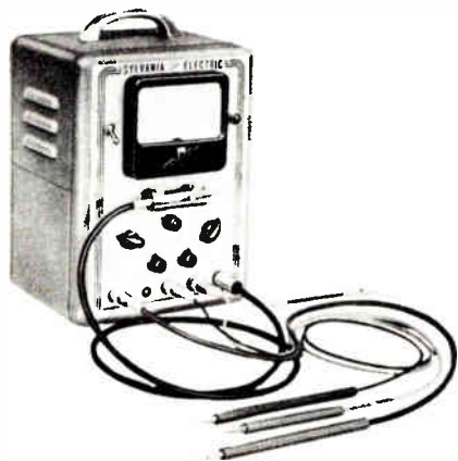
A vacuum tube voltmeter often is used as the resonance indicator when an FM receiver is aligned.
