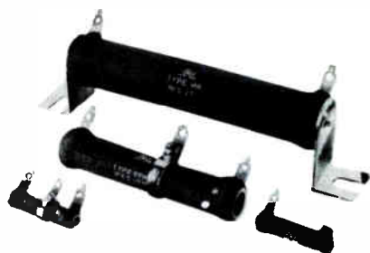
Wirewound resistors of various sizes. Occasionally, such units develop high resistance of the points where the terminals connect to the resistance wire.
