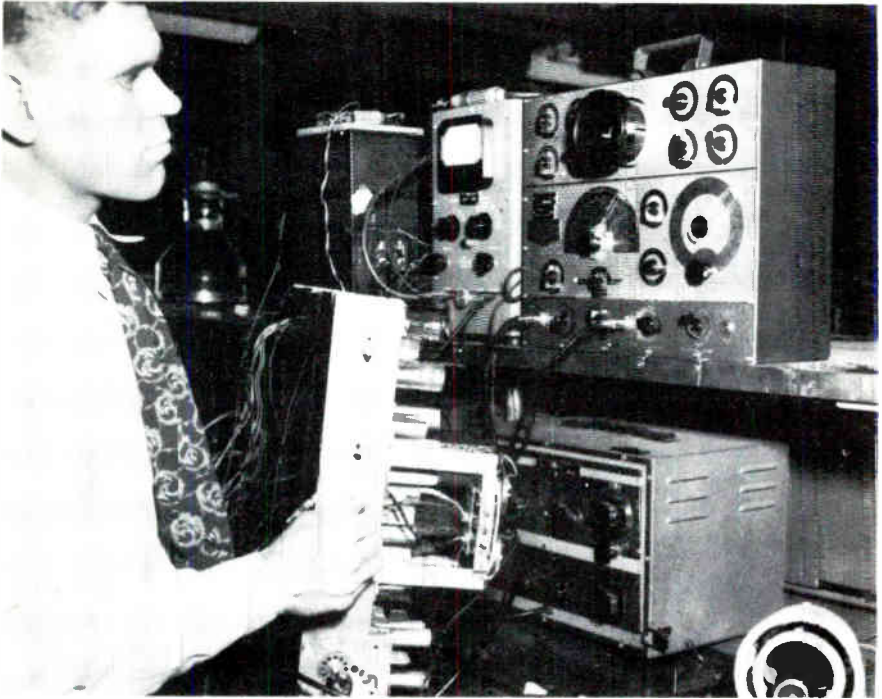
The VTVM, oscilloscope, and signal generator are the basic essential test instruments for the television service shop.
