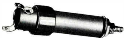
Wave trap resonant to 455 kc prevents radiated i-f signals from passing through the input circuits of a radio receiver.
