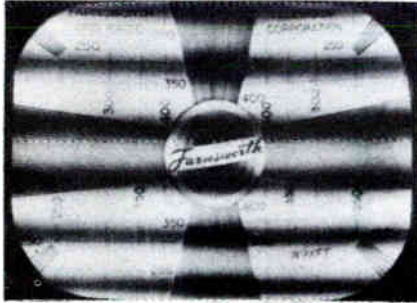
44. SOUND BARS FIGURE 6 COURTESY-FARNSWORTH
