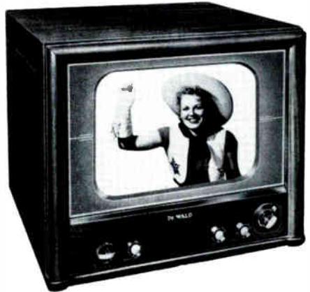
A rectangular picture tube with a "black" face to reduce glare is employed in this table model receiver.
