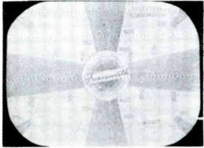
INSUFFICIENT CONTRAST FIGURE 7
