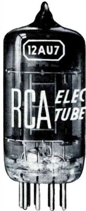
Often, disturbances in the television picture are caused by microphonic tubes, or tubes which are excessively noisy.
