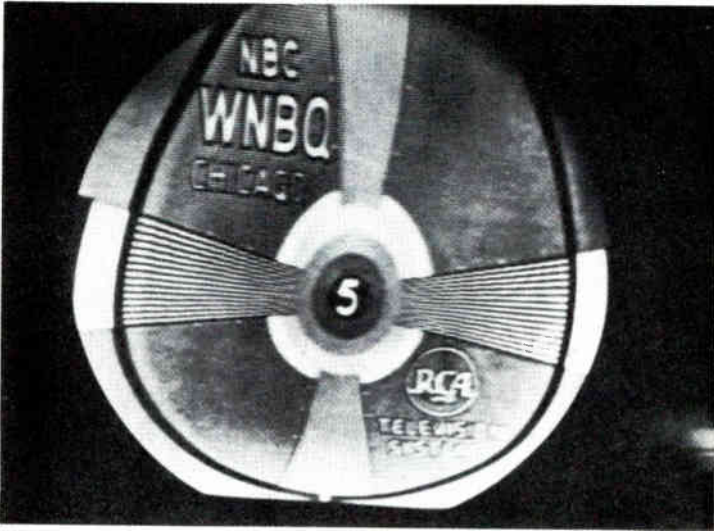
9. Poor Vertical Linearity. Adjust vertical linearity control.
