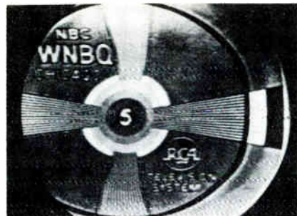
5. POOR HORIZONTAL CENTERING A
