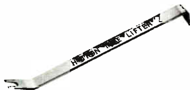
A handy tool which may be added to the service kit. It is used to remove tubes from the socket.
