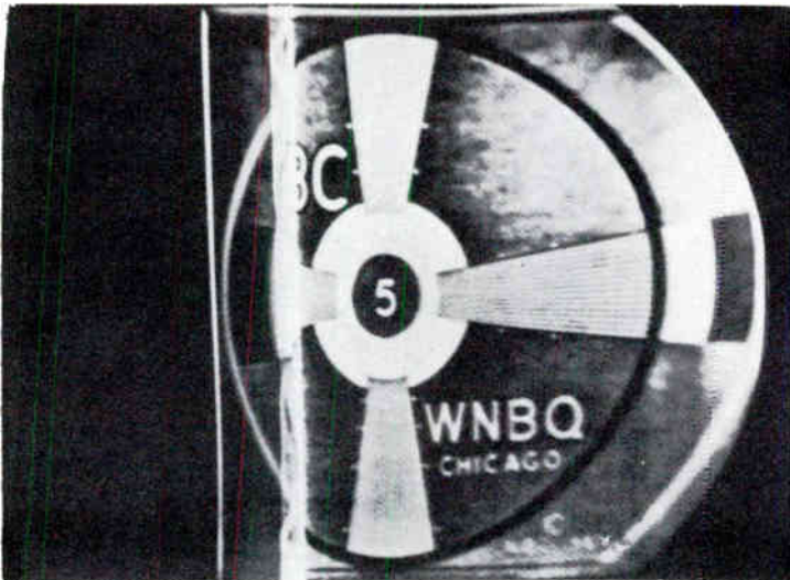
24. Horizontal Fold-over. Shorted damper tube. Open capacitor in linearity control circuit.
