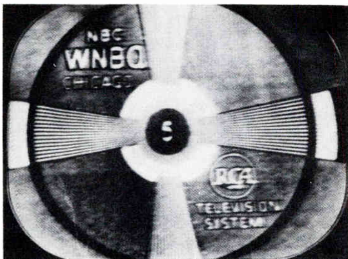
14. Smear. Poor Detail. Check fine tuning. R-f and i-f alignment.
