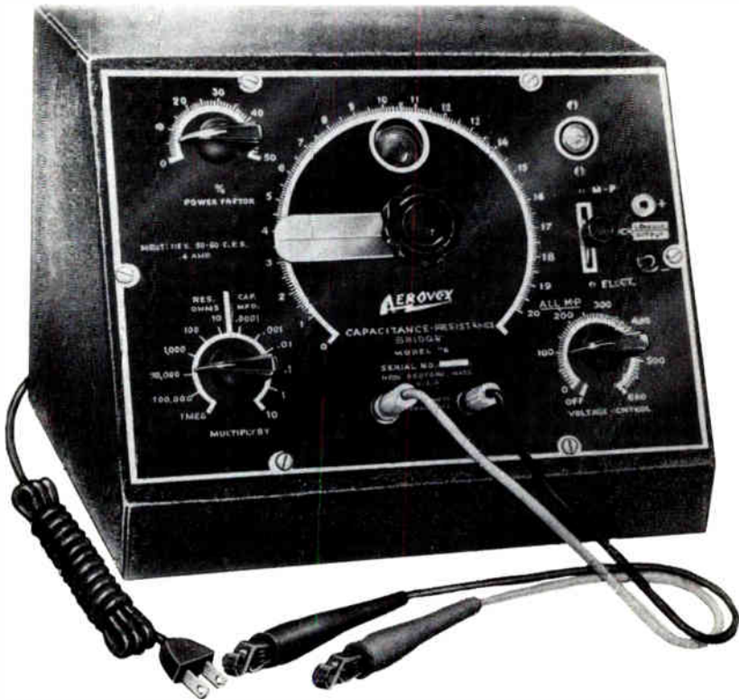
A service type instrument for checking capacitors and resistors.
