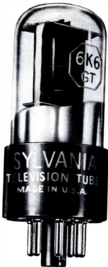
Tube used in the audio power output stage of television and radio receivers. Considerable distortion in sound output may be produced by a weak power output tube.
