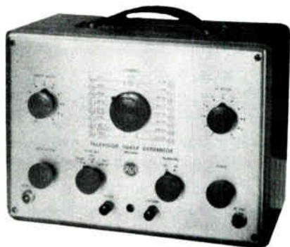
The selector switch sets the sweep oscillator to the center frequencies of the indicated channels and thus permits rapid channel changing in this TV sweep generator.
