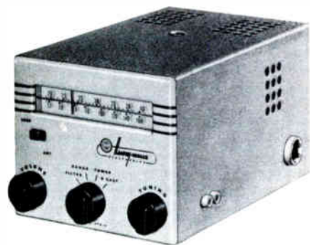
Transceiver used in aircraft communication. A wave trap may be needed to prevent interference from an r-f source of this type.
