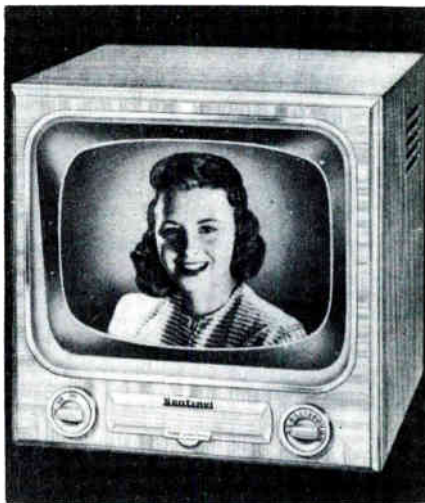
A large screen table model receiver. The same receiver chassis may be used in various type cabinets, however, the chassis number does not change unless a change is made in the receiver circuits.
