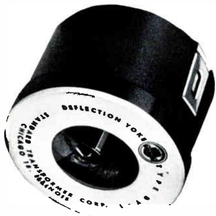
A tilted picture, reversed picture, or keystone shaped raster, etc. can be produced by a deflection yoke which is improperly positioned, incorrectly connected, or shorted.
