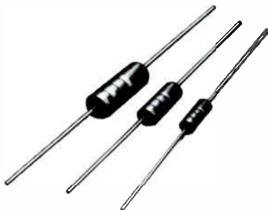
Distorted sound output may result from changes in resistance of carbon resistors due to heavy current overloads or to aging.
