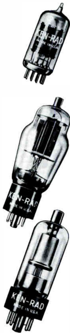
Nearly worn out or defective tubes are frequent sources of intermittent troubles.
