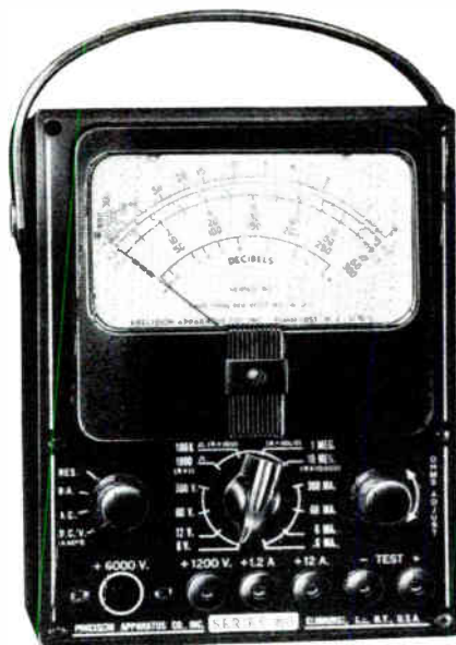
Typical multimeter of the type employed as an output meter for aligning AM receivers.
