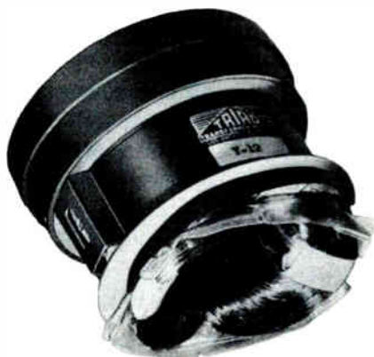
A no raster condition results when there is an open in either of the vertical or horizontal coils of the deflection yoke.
