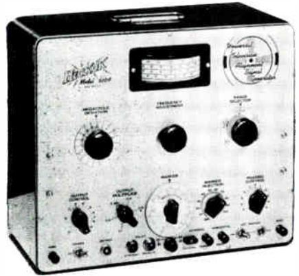
Sweep signal generator for aligning television receivers. The unit contains a marker generator and means for employing the signal from an external marker oscillator.
