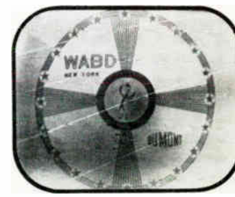
COURTESY A. B. DUMONT LABS., INC. CONTRAST TOO LOW H
