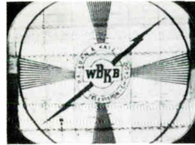
47. IGNITION INTERFERENCE A
