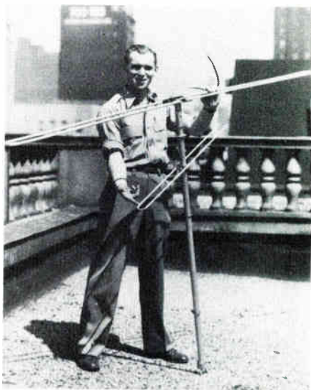
Carried around the roof, a test antenna connected by a temporary lead-in to the receiver may be employed to find a ghost-free location to which the regular antenna may then be moved.
