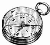
A small magnetic compass. The blue end of the magnetized needle is the north seeking pole.
