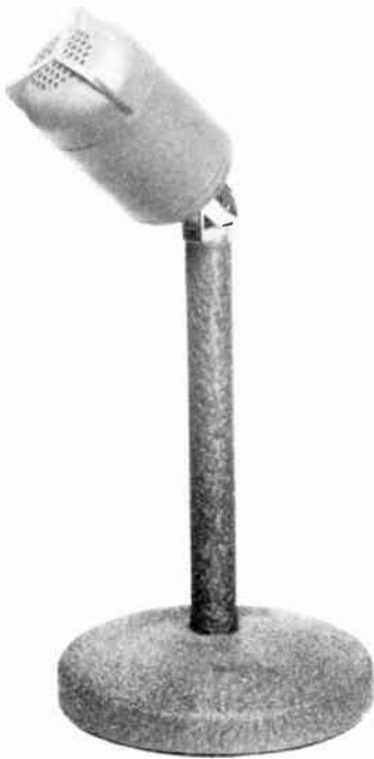
This microphone is mechanically a miniature speaker.
