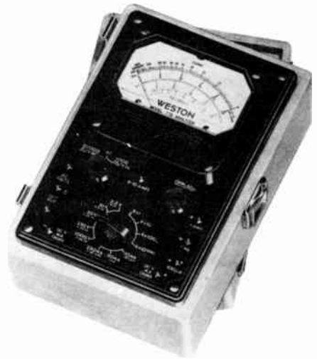
This multimeter has two sensitivity ratings: 20,000 \Omega/v on d-c and 1,000 \Omega/v on a-c.
