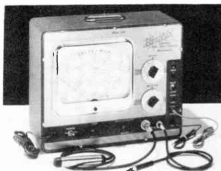
This vacuum tube voltmeter and capacitance checker is used not only to service radios, but TV sets, and other electronic equipment as well. The capacitance checker is just added scales for the ohmmeter to indicate the proper kick for each size capacitor.
