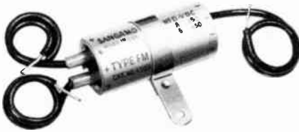
Electrolytic capacitor with two 8 \mu f sections. The negative plates are tied to a common lead.
