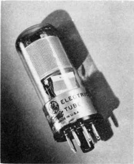
Surrounding the tube elements in this pentode, the perforated metal cylinder is connected to the screen grid and helps to shield the plate from the control grid.
