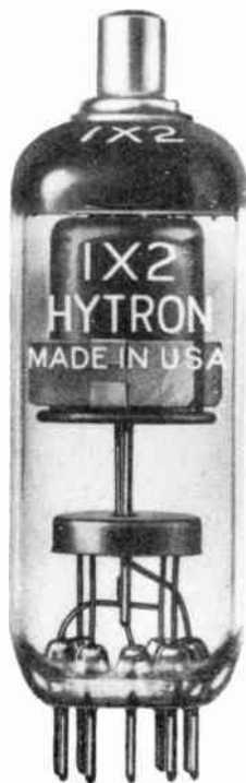
A high voltage rectifier used in television receivers. The plate connection is through the cap on top.
