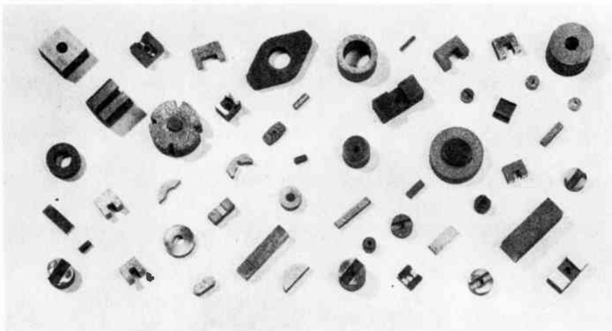
For various applications, permanent magnets are fashioned into a wide variety of shapes and sizes. Pictured are a few representative types.
