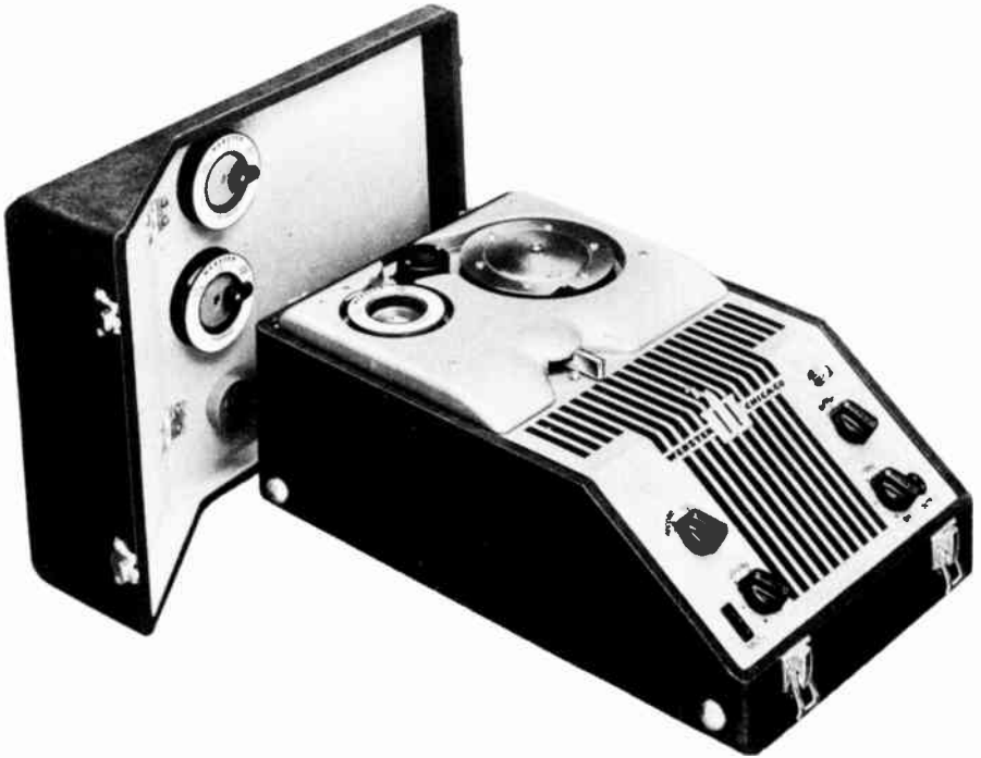
A wire recorder utilizes an electromagnet which magnetizes a special type of iron wire. Although easily magnetized the wire retains the magnetism. Note the extra spools of wire in the cover.
