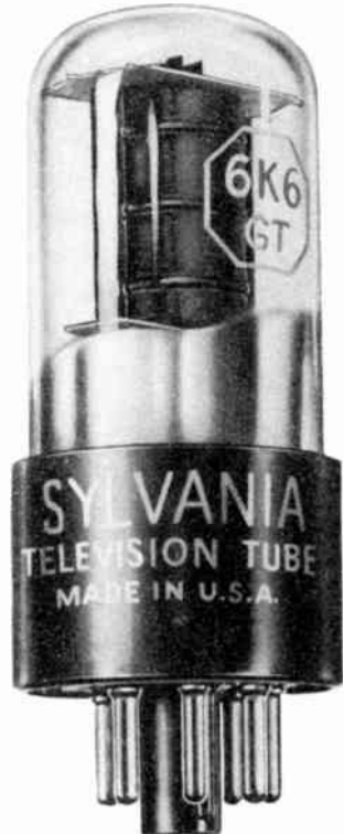
The mirror-like finish on the inside of the envelope is due to the deposit of the getter on the glass after it has been flashed.
