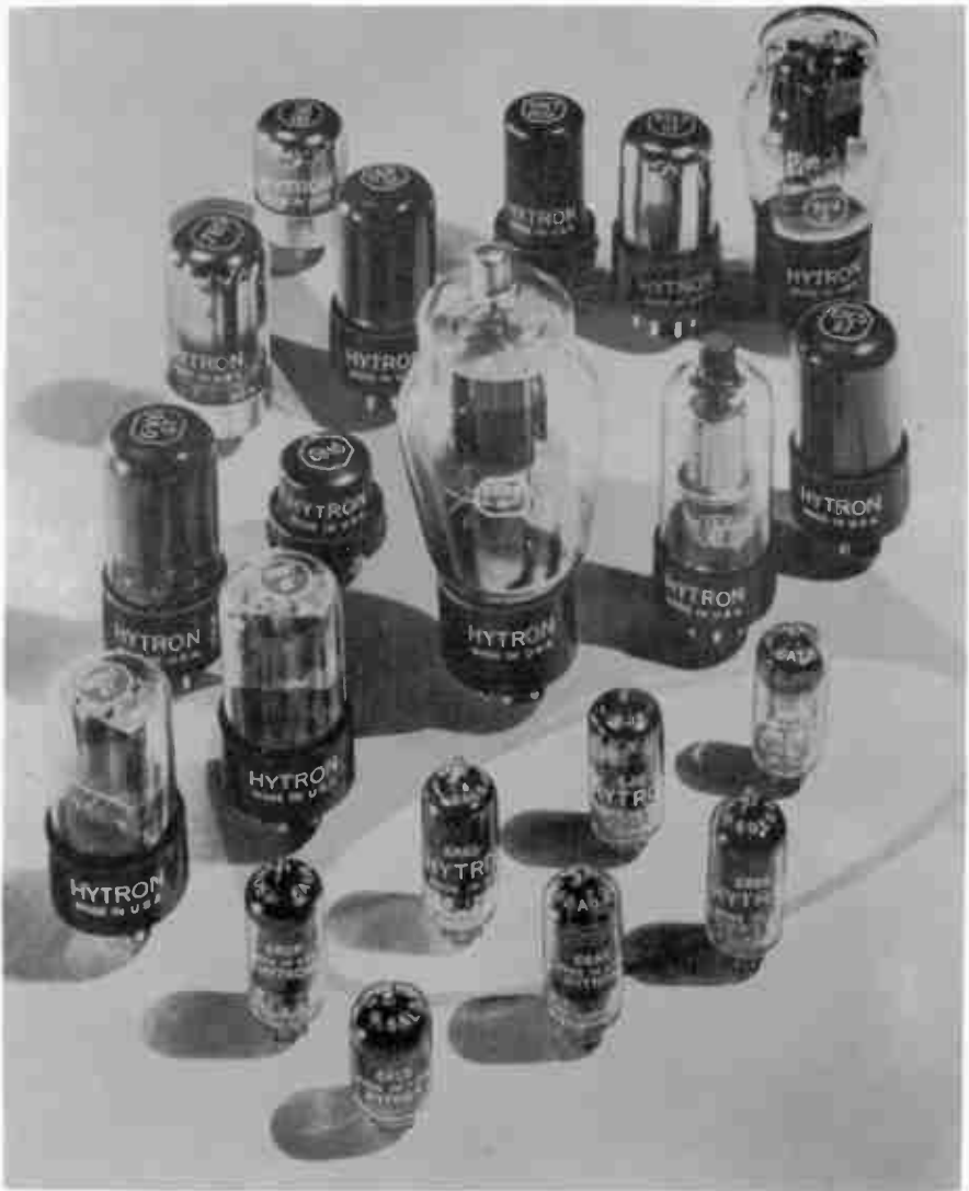
These are but a few of the large number of tubes having various sizes and shapes that are used in electron equipment. In fact, all of the tubes shown here are used in one television receiver.
