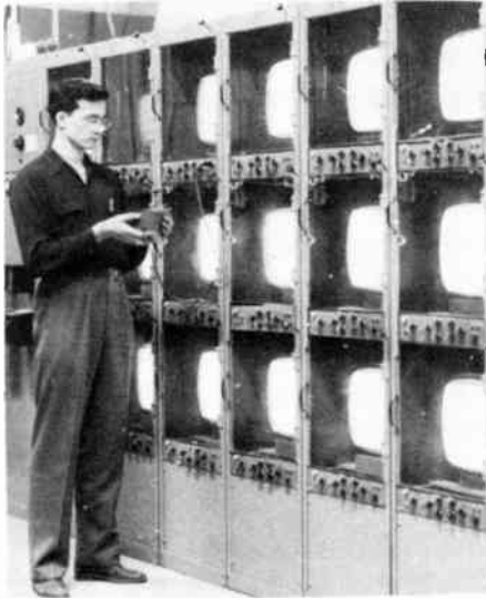
Life tests are being run on these television picture tubes. They are periodically checked by a technician.
