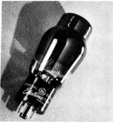
Tubes designed for power amplifier applications are usually larger than other amplifier tubes to make them more capable of dissipating the heat generated.
