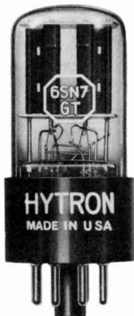
Two complete triode units are mounted in this evacuated tube to conserve space and material.
