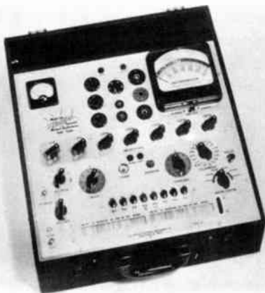
Shown is one type of tube checker. It tests the tube while operating in a circuit built in the instrument.
