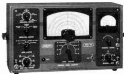
This service type instrument generates a wide range of frequencies which are needed to tune oscillators and i-f transformers to their proper frequencies.
