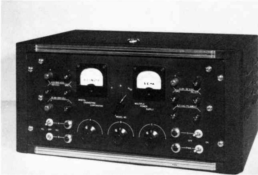
Front view of a complete laboratory power supply having three ranges of variable voltage.
