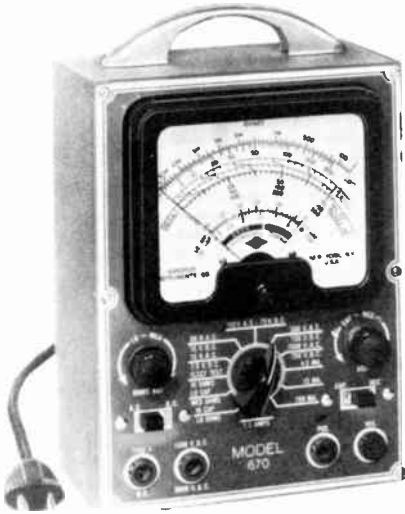
The electronic voltmeter above can be used for voltage, resistance, and capacitor measurements.
