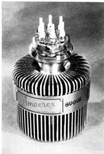
Tubes designed to deliver very powerful signals must use fins like these or a water cooling system to keep from overheating.
