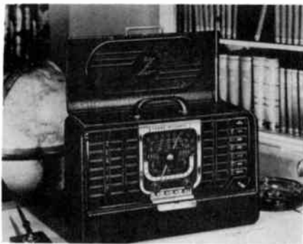
To make it easy to carry, this multi-band radio has a number of circuits in a small space. Point-to-Point testing is a very effective means of servicing it.
