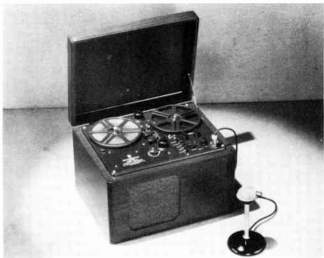
This tape recorder incorporates an amplifier to build up the signals from a microphone or radio until large enough to operate the "recording head".
