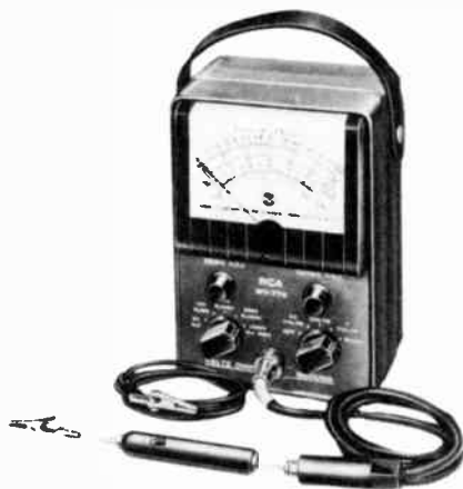
Here the direct probe plugs into the d-c probe, thereby eliminating a third lead.
