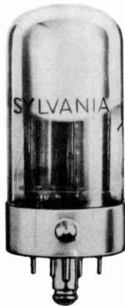
This lactol type tube is held securely in its socket by a locking arrangement of the center guide pin at the bottom of the tube.
