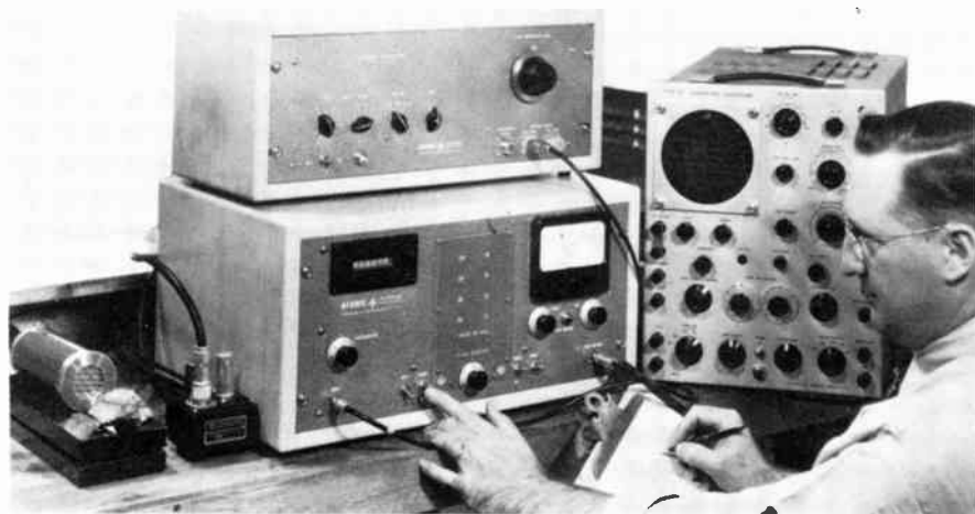
Amplifiers are important in these nuclear laboratory instruments used to measure the radioactivity of a sample in front of the counter tube in lower left corner.
