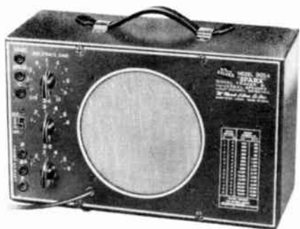
A signal tracer is a detector, amplifier, and speaker used to trace a signal through every stage of a radio.
