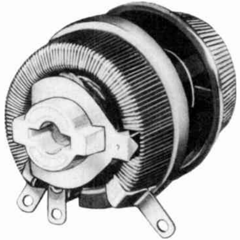
A typical wire-wound potentiometer with adjusting knob attached. For better heat dissipation, the wire is left exposed.
