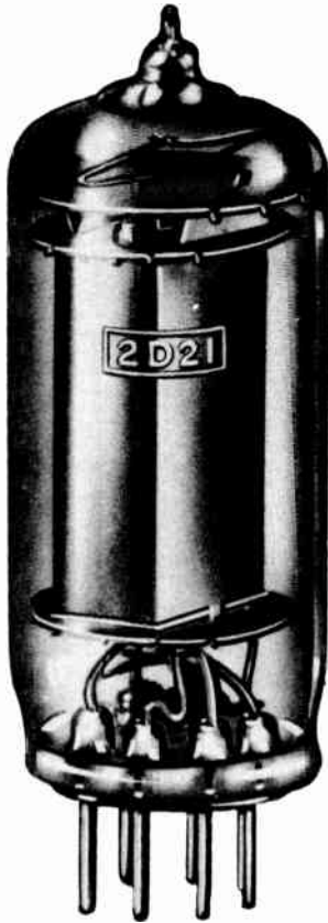
A four electrode inert gas tube that is used in pulse circuit applications.
