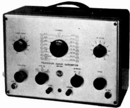
A good sweep generator is essential for accurate reproduction of the i-f amplifier response curve on an oscilloscope screen.
