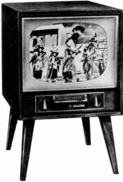
A modern television receiver like the one above is basically a radio receiver with cathode ray tube and pulse circuits added.
