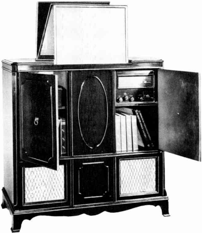
In this projection television receiver the picture is reflected onto the semi-transparent screen by a mirror mounted at an angle of 45°.
