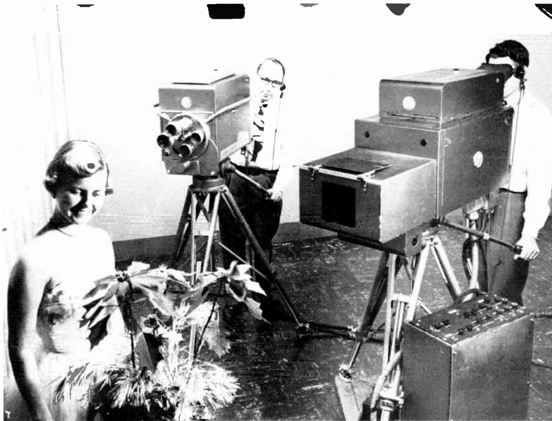
A single tube color TV camera is shown on the left. The one on the right is a three tube color TV camera.
