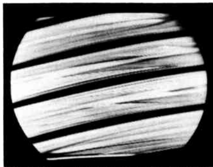
The picture becomes a meaningless blur when the TV receiver lacks horizontal sync.
