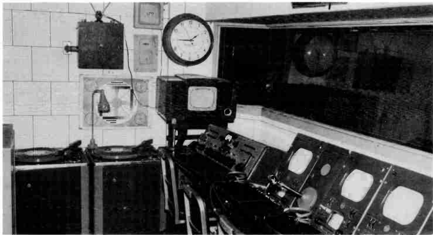
The monitor console for a television studio. The home type receiver (under clock) may be used to monitor the transmitted program. Each of the monitoring units contains its own high voltage supply.
