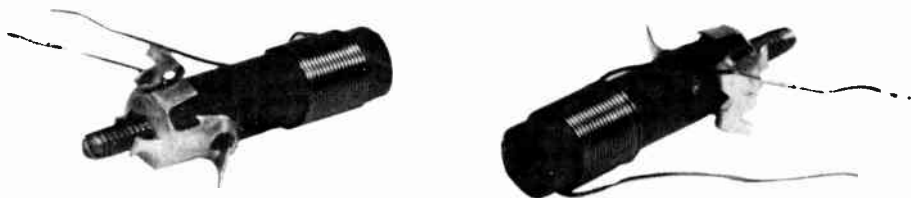
I-f coils designed for simple impedance coupling. The metal clips are used to mount the coil in chassis holes and to hold the powdered iron cores in position. These cores are screwed up or down from the top side of the chassis until the proper inductances are obtained.
