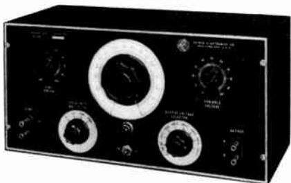
The relaxation oscillator used in this generator provides a square wave voltage for test purposes. Courtesy Reiner Electronics Co.
