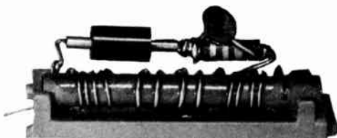
UHF tuning strips. The preselectors, crystal mixer, i-f output transformer, and harmonic selector are mounted on the strip at left. The harmonic generator, bias network, and the VHF mixer and oscillator tuning coils are shown on the strip at right.
