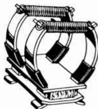
Examples of single and double frame beam benders. Sometimes these are erroneously called "ion traps."
