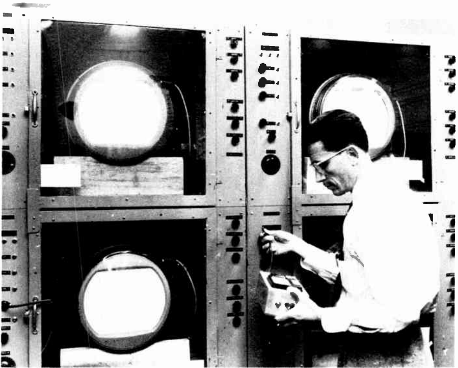
Color picture tubes are given a life test by producing an unmodulated raster on the screen. The raster is produced by deflection oscillators similar to those used in the TV receiver.
