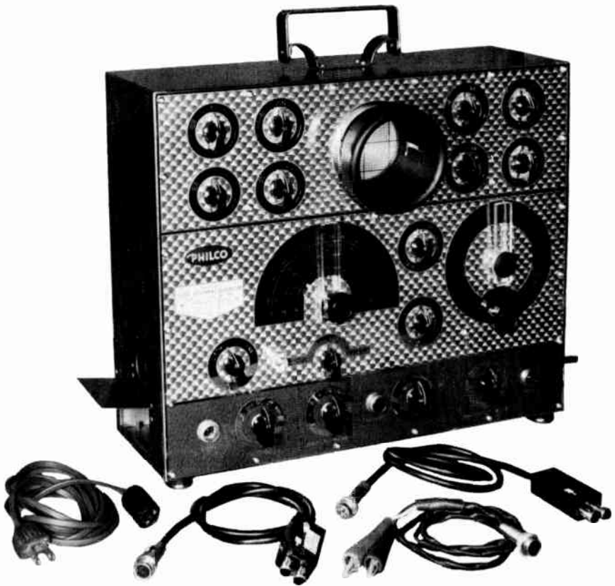
A combination oscilloscope and sweep generator designed specifically for TV receiver alignment.
