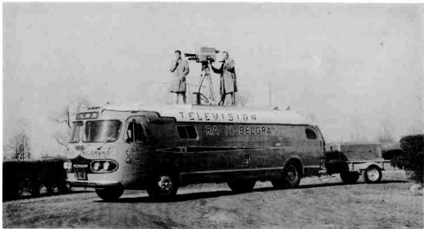
The mobile television unit, a complete studio on wheels, is used to pick up field events and relay the program to the main studio.
