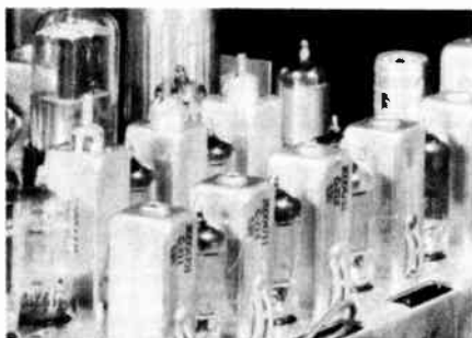
A Dual Channel TV receiver sound and video i-f strips. The coils are mounted inside the shield cans between the tubes in order to reduce interaction through unwanted magnetic coupling.
