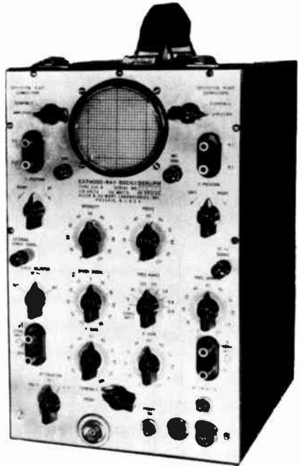
A control on the front panel of the oscilloscope provides selection between three sources of voltage to synchronize the horizontal sweep oscillator.
