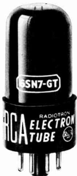
The 6SN7 duo-triode is a popular tube for multi-vibrator circuits.
