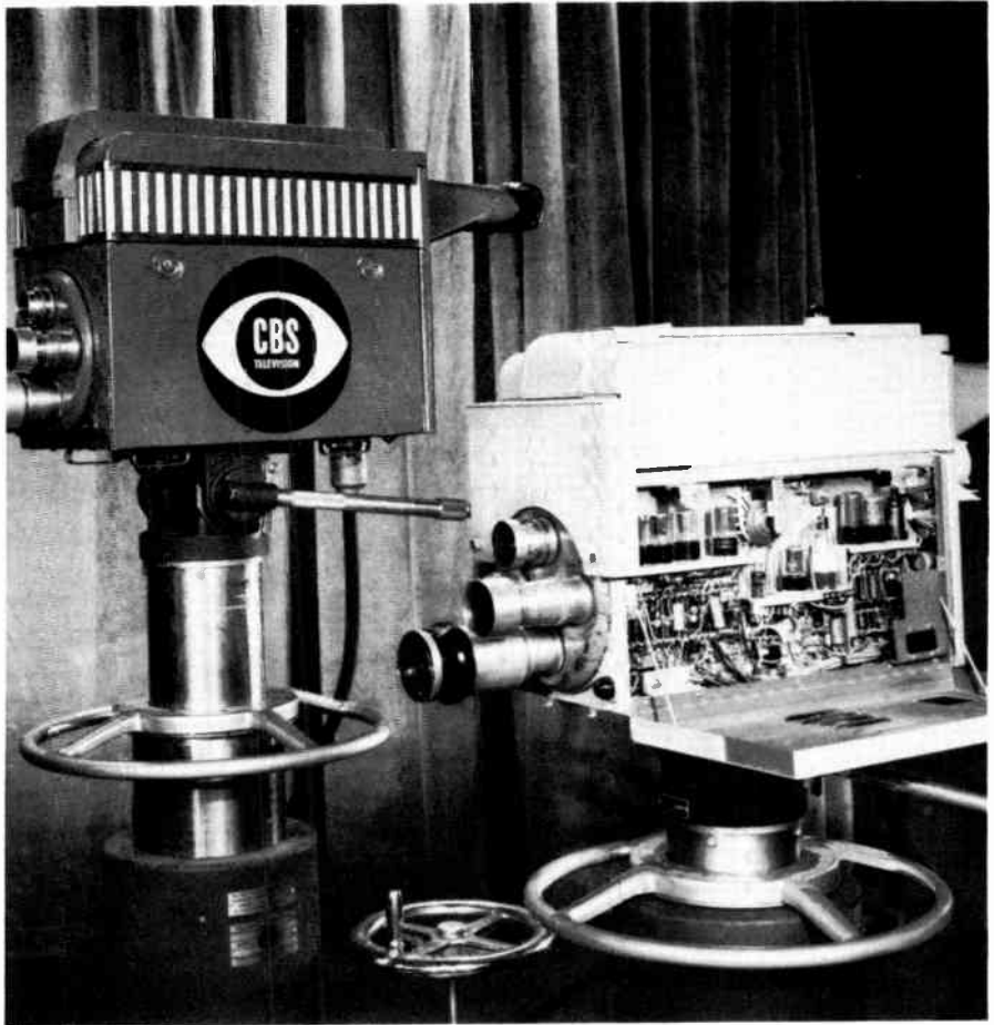
The color television camera on the right is equally as compact and maneuverable as the standard black and white television camera. This color camera provides field sequential color television pictures which are converted to the NTSC color television signal. Only one image orthicon is required.
