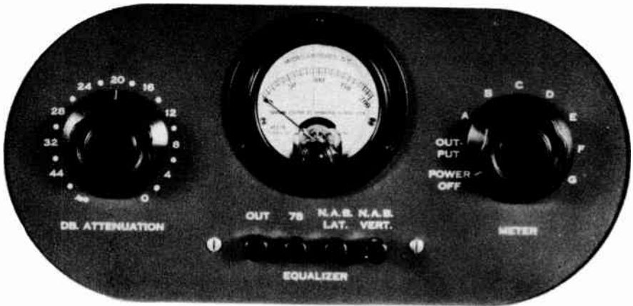
An attenuation and equalizer panel designed to control audio frequency voltages in the recording industry.
