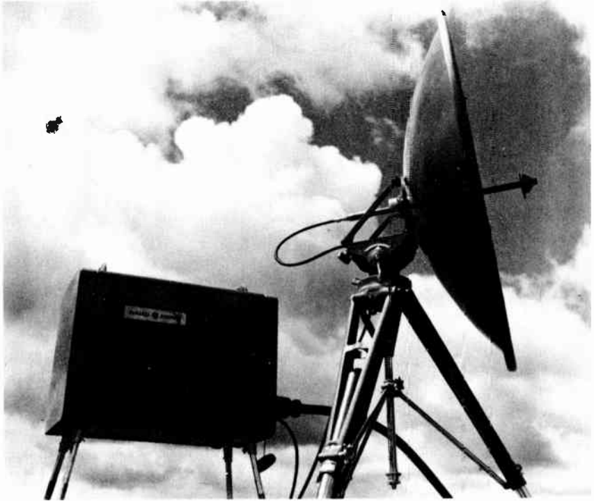
A microwave antenna (parabolic dish) and associated equipment used to beam television programs from remote points to main studios. Coming out of the rear of the reflector is the coaxial transmission line used to supply r-f power from mobile transmitter.
