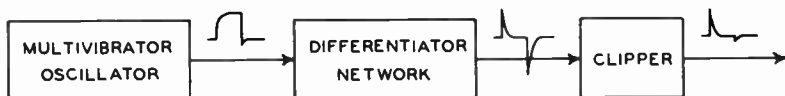
The block diagrams of two types of timing circuits used in radar. Note the output pulse is similar in each system.
