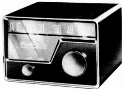
The UHF tuner, continuously tunable from Channel 14 through Channel 83, is designed as a separate unit to provide UHF reception with existing VHF receivers.
