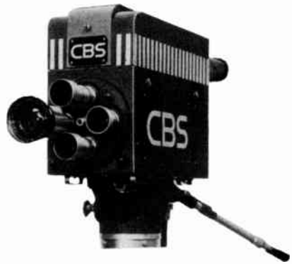
The television camera changes the scene into electric pulses which are amplified and transmitted.
