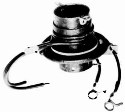
A horizontal deflection transformer of the air core type found in TV receivers.
