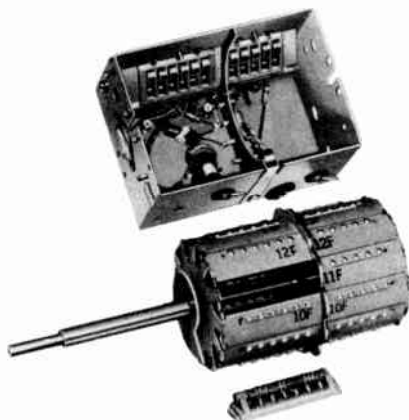
The turret tuner is disassembled to show circuit wiring and method of connecting the tuning strips.
