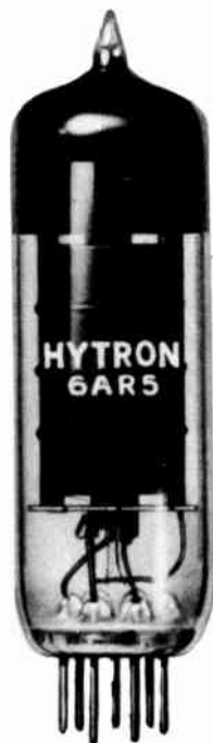
The 6AR5 has a G_m of 2400 \mu mhos which makes it suitable as the video amplifier output stage.
