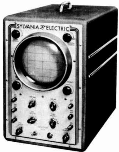
In an oscilloscope the switch labeled "course frequency" selects the RC combination which determines the frequency and wave shape of the sawtooth sweep voltages.
