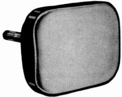
The rectangular type CRT is designed to reproduce a picture with the standard aspect ratio of 4 to 3 without wasting screen space.
