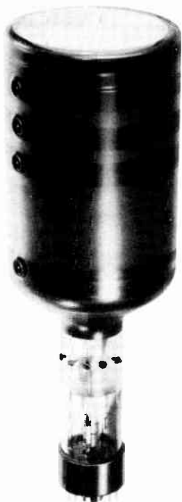
The 5RP4 Cathode ray tube is an electrostatic deflected projection tube. Due to the high anode and deflecting voltages, the connections are made through the neck instead of the base.
