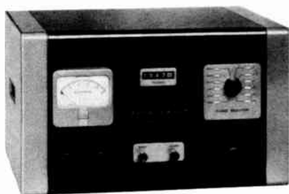
Many nuclear instruments also require wide range amplifiers to amplify the short pulses encountered during normal application. This particular instrument measures the time required for a predetermined number of particles to ionize a Geiger tube.
