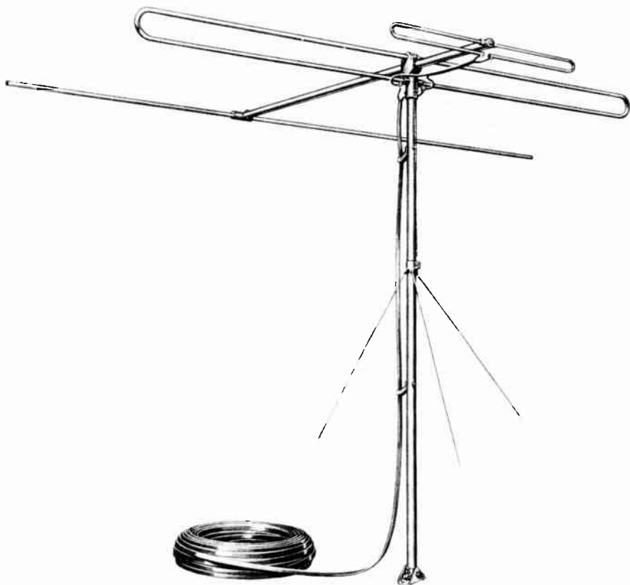
A hi-law television antenna. To effect greatest transfer of energy from antenna to receiver, the impedances of the antenna, transmission line, and receiver input must be matched.
