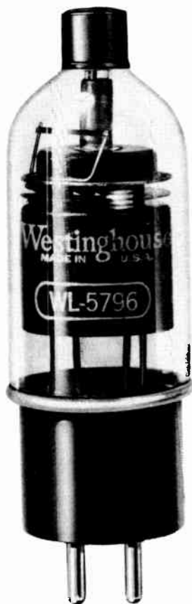
An inert gas thyratron of the type used in electronic control applications.
