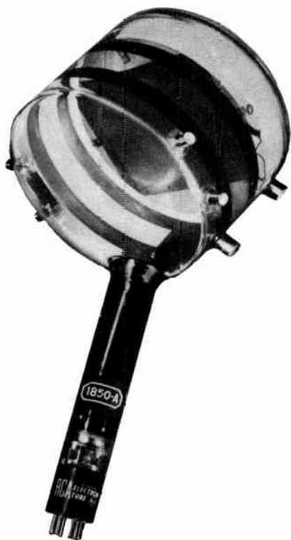
An iconoscope camera tube. The pictures are focused on the mosaic mounted inside the face of the tube.
