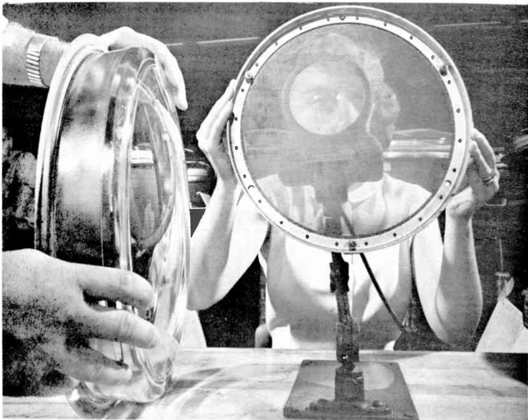
On the left, a face plate and on the right a shadow mask of a color picture tube are being inspected at the factory.
