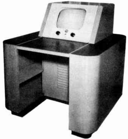
A monitor is used in the studio to observe the picture being transmitted.
