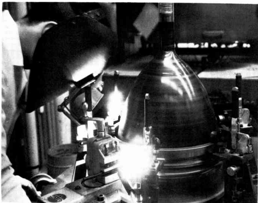
Precision machined flanges on the faceplate and bulb join the two sections of this color picture tube. The faceplate is corefully welded to the bulb cone.
