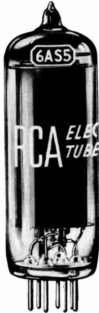
The 6AS5, a miniature beam power amplifier, often is used in the output stage of the sound section. Courtesy Radio Corporation of America
