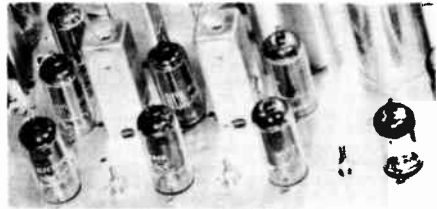
The i-f strips of a typical television receiver. Notice the clips and core screws for the video i-f coils in the foreground between the tubes.
