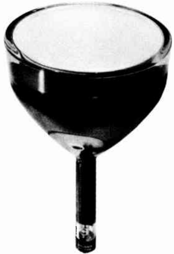
The inside of a glass CRT is painted with a conducting material called "aquadag" to provide a path from the screen to B+.
