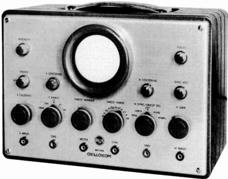
The relaxation type oscillator used in the oscilloscope supplies the necessary pulse voltage used for horizontal deflection of the cathode ray tube electron beam.
