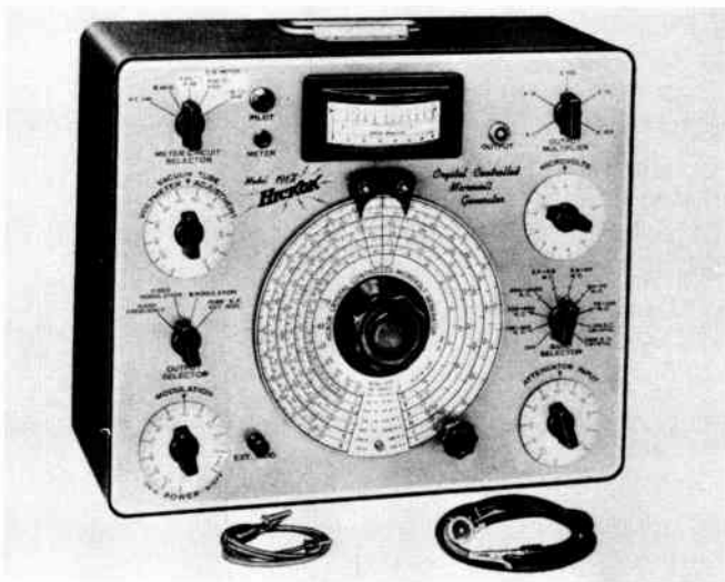
Resistance attenuators are used to control the amplitude of the various signals generated in this test instrument.
