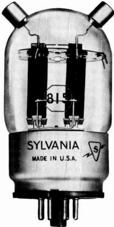
A transmitter type amplifier tube. The interelectrode capacitances depend upon the size, shape, and spacing of the electrodes. Note the glass bulb is made large to dissipate heat.
