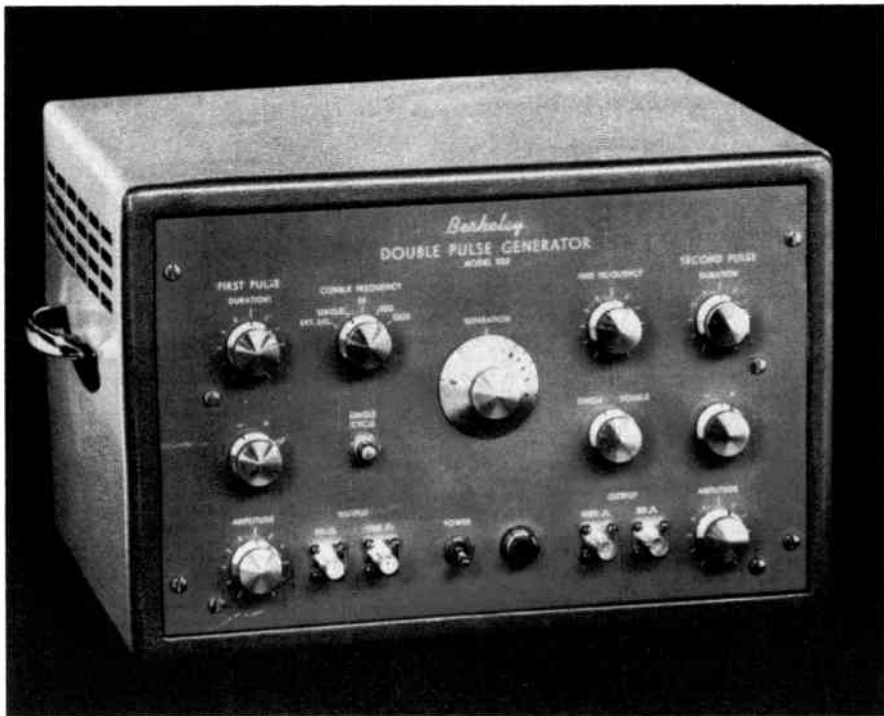
A double pulse generator which supplies either single or paired pulses. The pulses are individually variable in width, amplitude, and spacing.
