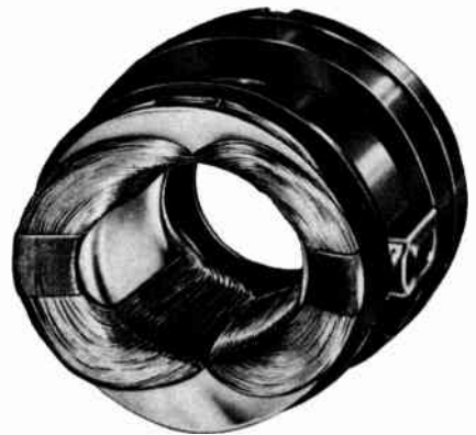
The deflection yoke contains both vertical and horizontal deflection coils shaped to fit around the neck of the CRT.
