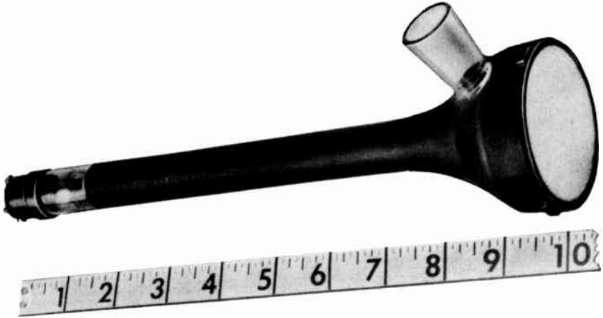
Projection tubes employ an added automatic brightness control circuit to protect the screen from immediate damage if the sweep circuits fail. The tube is biased to cutoff until sweep voltages applied to the control tube reduce the bias.
