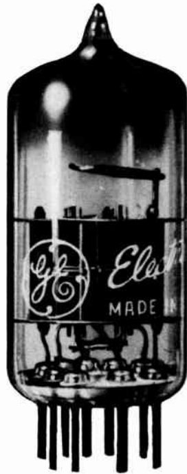
Due to its low interelectrode capacitances this twin triode, 12AT7, often is used in grounded grid amplifier circuits.
