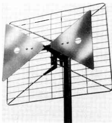
A "bow tie" antenna with a sheet reflector is suitable for all UHF channels. The two holes in the bow reduce wind resistance.
