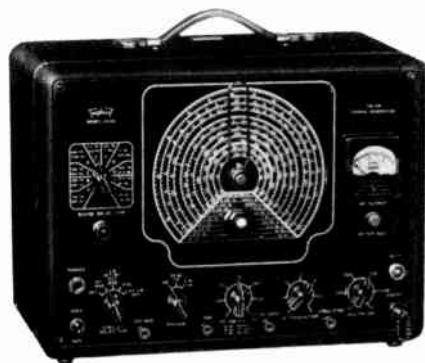
This signal generator provides a horizontal sync voltage for synchronizing the sweep generators of the oscilloscope used with it during receiver alignment.
