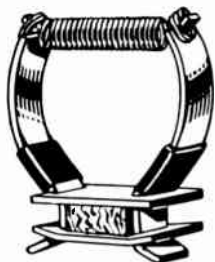
Examples of single and double frame beam benders. Sometimes these are erroneously called "ion traps."
