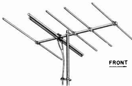
A small Yagi antenna. Only one reflector and three directors are used in this array. A six or eight element array is not uncommon for UHF reception.
