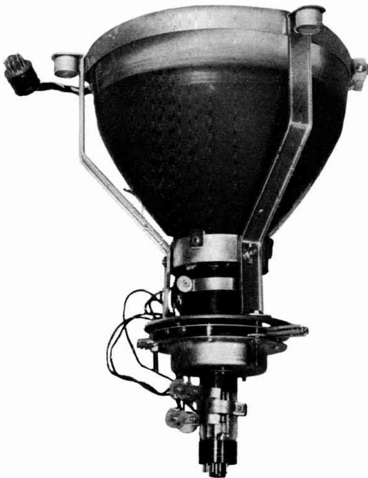
A round CRT mounted in brackets which also hold the deflection yoke and focus coil. An electromagnetic beam bender is shown mounted near the base of the tube.
