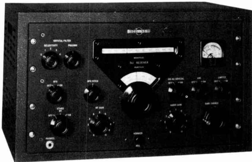
This elaborate communication receiver has provisions for switching the limiter in or out of the signal circuit.
