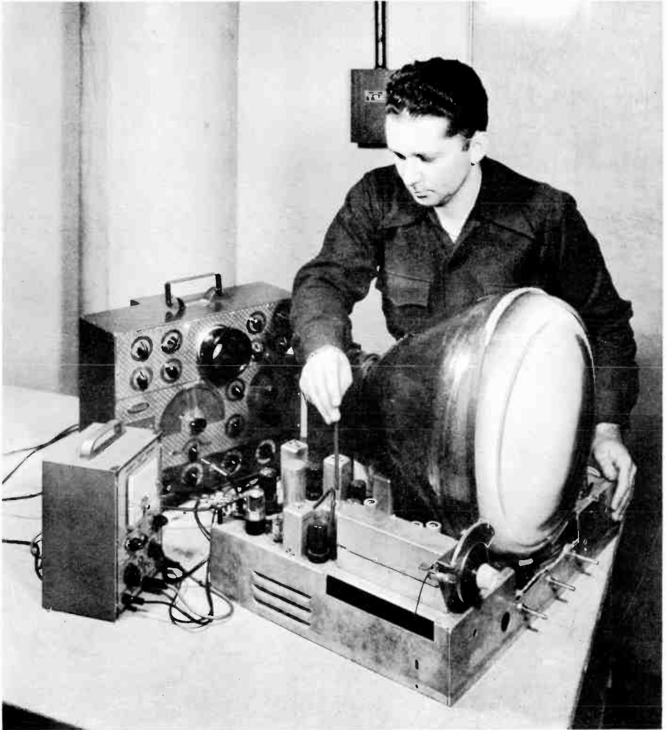
Fig. 1. This student in the Coyne School is aligning a television receiver. He is adjusting the i-f coupling transformers to their correct resonant frequencies.
