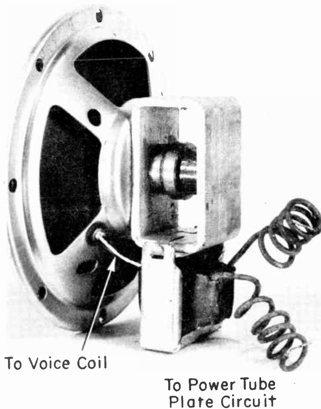
Fig. 10. Wire connections on an output transformer for the speaker.
