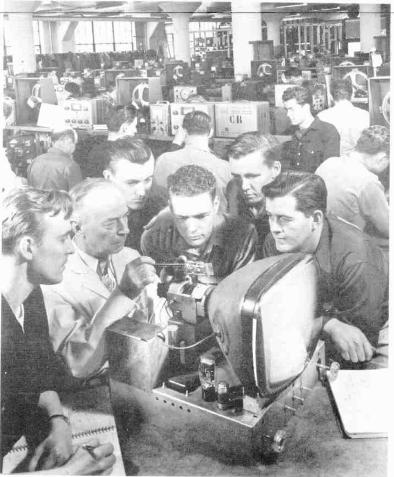
Fig. 1. Students in the Coyne School are examining the electron gun from a television picture tube.
