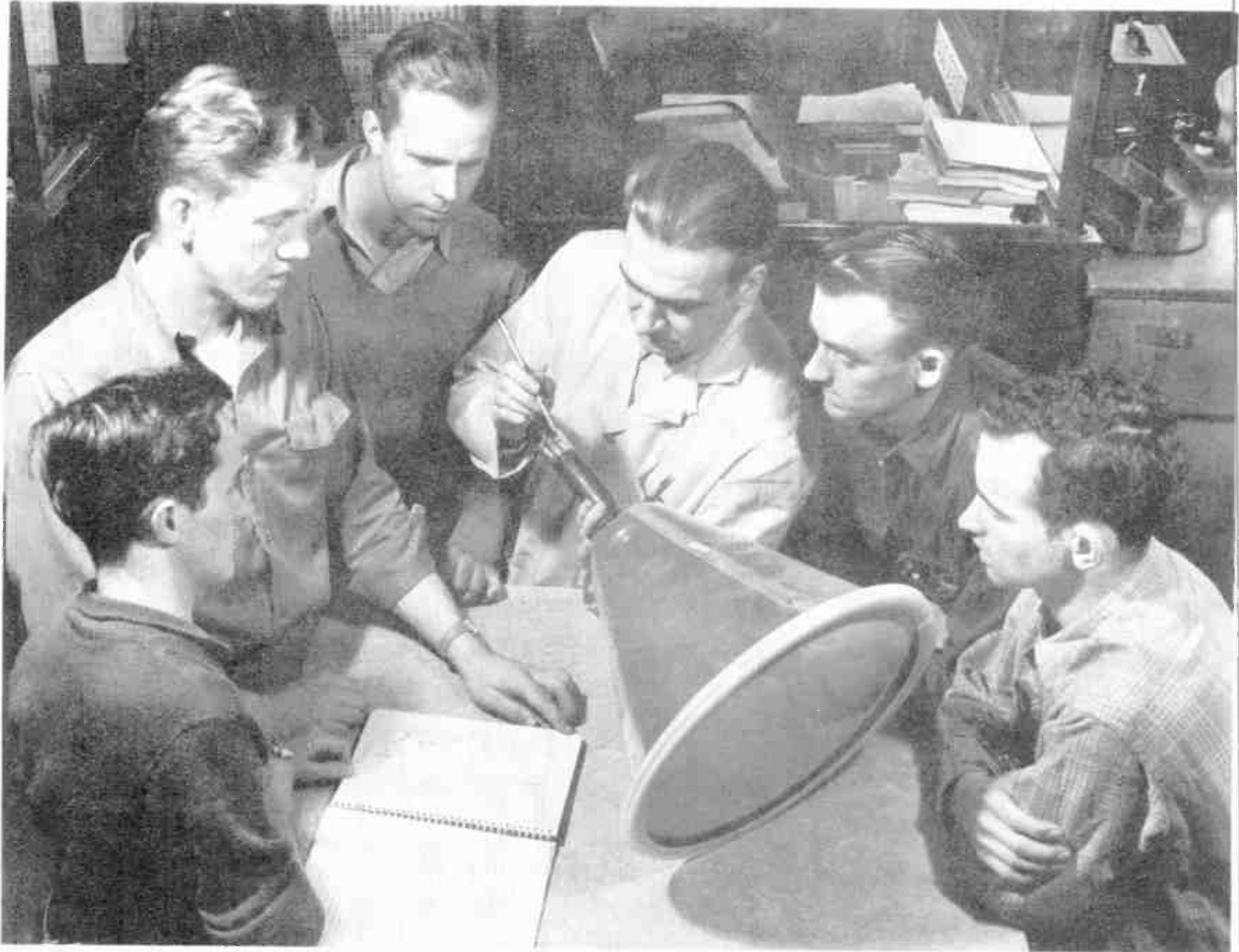
Fig. 1. Coyne students are examining a metal-cone picture tube fitted with a protective cover and an insulating ring around the lip.
