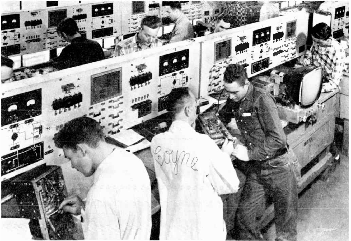
Fig. 1. These service benches in the Coyne School are equipped with instruments and convenient connections for tracing circuits.
