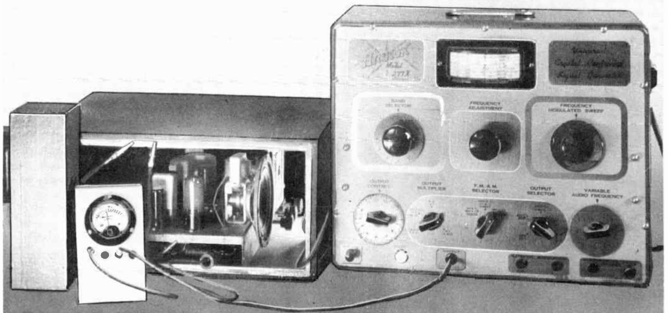
Fig. 8. The receiver is being tested for sensitivity by measuring strengths of signals at the antenna input and at the speaker output.
