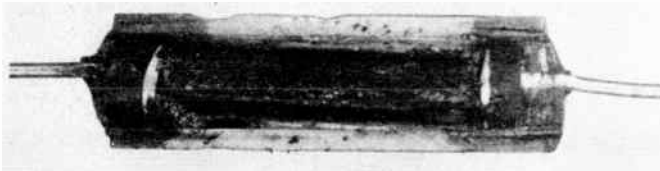
Fig. 9. A carbon type composition resistor cut open to show the internal resistance element and the outer protective insulation.
