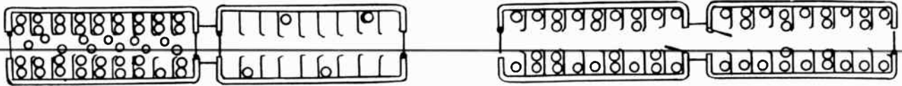
Fig. 7. Just as people like to move from an overcrowded car to one nearly empty, so electrons like to flow from where there are a great many to wherever there are fewer.
