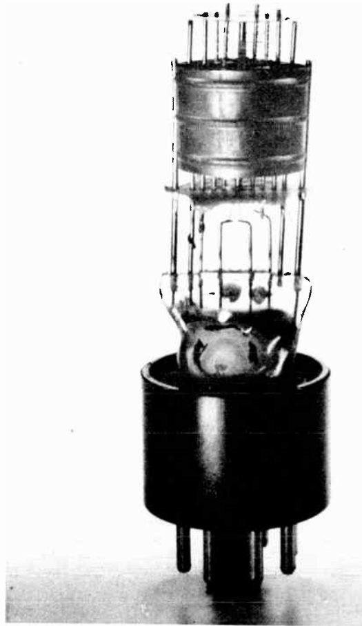
Fig. 6. The elements inside a tube are conductors because they are made of metal.
