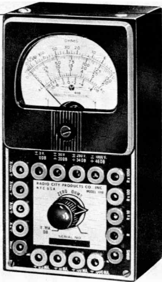
Fig. 18. A volt-ohm-milliammeter with pin jacks instead of a selector switch.
