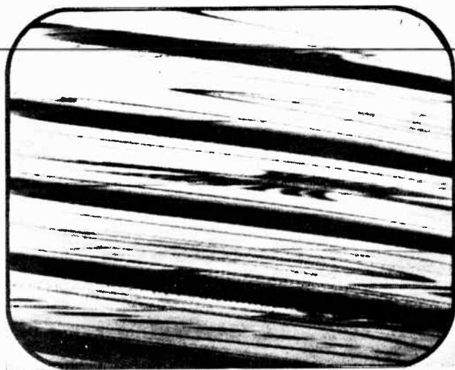
Fig. 18. Failure to hold picture synchronization might result from faults in a video amplifier section.
