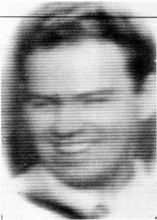
Fig. 5. A television picture is not continuous, but consists of many horizontal lines.
