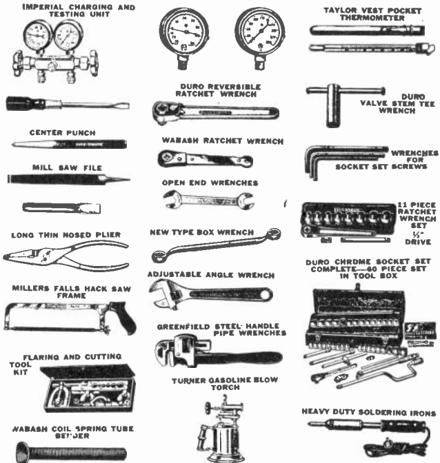
Fig. 10. Above are shown some of the most commonly used refrigeration service tools.
