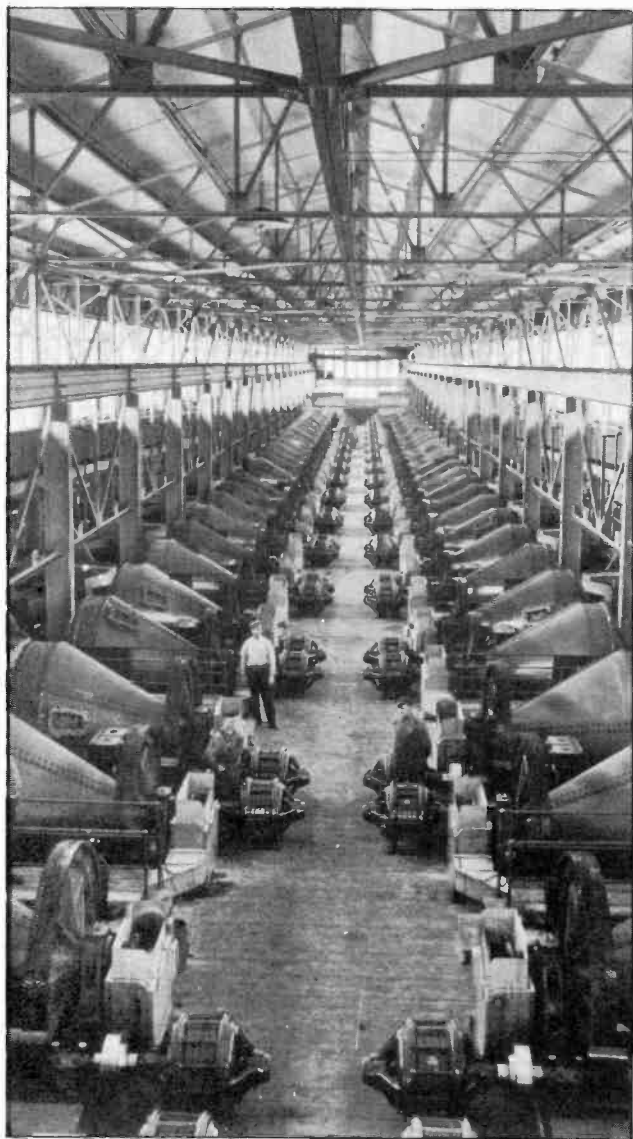
Regrinding mill, in copper plant. These machines grind ore bearing rock that was regarded as waste years ago.
