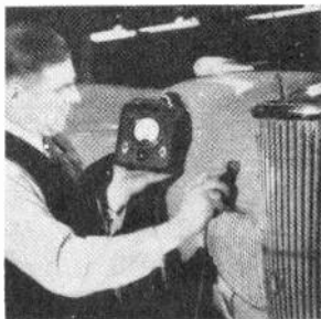
Film-thickness gage measures thickness of nonmagnetic materials—such as enamel, lacquers, glass, mica—when placed on steel. Standard scale range is 0 to 0.1 inch.
