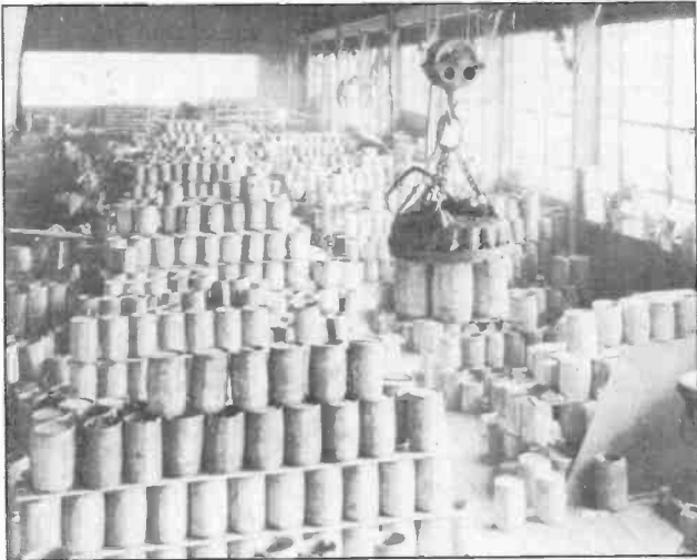
Fig. 8. Direct current is used to operate powerful electro-magnets of the above type for handling metal materials in industrial plants, warehouses, foundries, and iron yards. Note the manner in which these kegs of bolts are lifted by the magnet, even though the wooden heads of the kegs are between the magnet and the metal to be lifted. In plants where the principal supply of electricity is alternating current small motor generators are often used to supply the direct current for magnets of this type.
