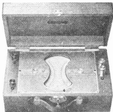
Fig. 13. This photo shows a high grade portable combination voltmeter and ammeter combined in one convenient carrying case. Such instruments are very handy for maintenance electricians.
