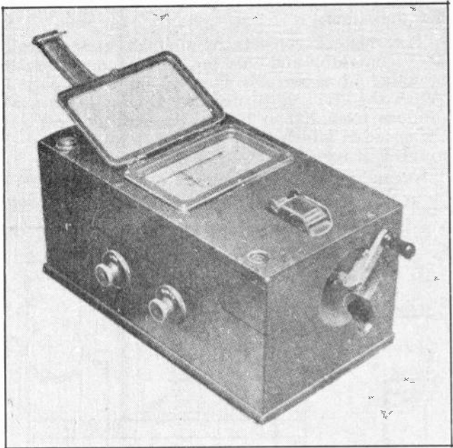
Fig. 16. The above photo shows a "Megger", or device used for measuring the resistance of insulation and high resistance circuits. This instrument contains its own D. C. generator as well as meter element.
