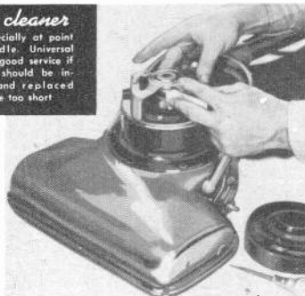
22 CLEAN COMMUTATOR WITH FINE (8-0) SANDPAPER
