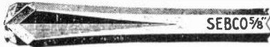
Fig. 27. This view shows the cutting nose of a star drill, such as used for drilling holes in masonry for attaching or running conduit in buildings of masonry construction.
