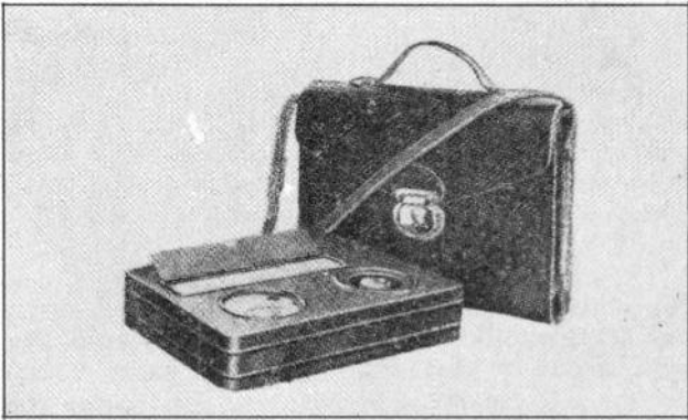
Fig. 16. A foot-candle meter is a very convenient instrument used for measuring illumination intensities right on the job.
