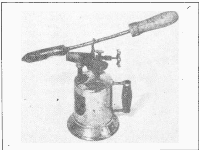
Fig. 2. This photo shows a gasoline blow torch such as commonly used for heating soldering coppers, and splices in electrical conductors.
