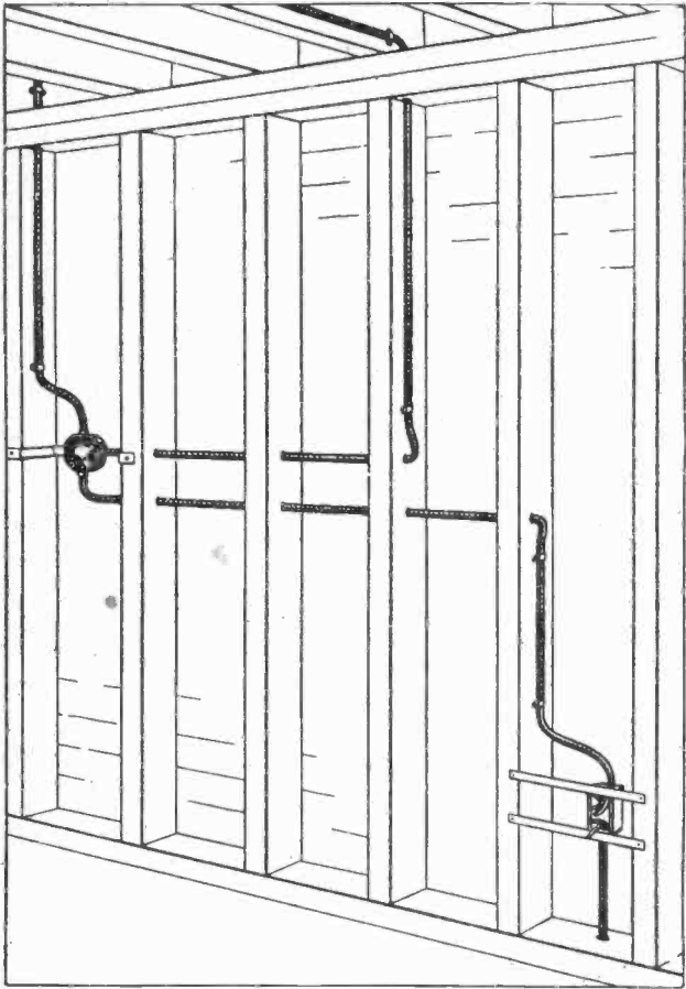
Fig. 13. A section of an installation of RomeX, showing how it is run through and along joists of a building.
