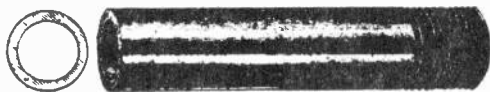
Fig. 16. Piece of rigid conduit or pipe, in which wires are run in conduit systems.
