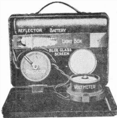
Fig. 17. This view shows the important parts of a foot-candle meter. Note the arrangement of the standard lamp behind the paper screen, and also the rheostat and voltmeter used in making proper adjustments.
