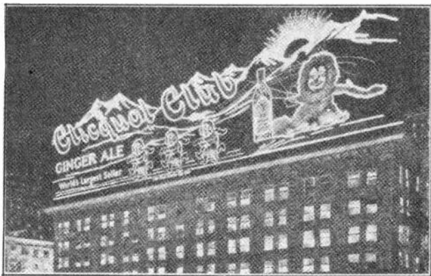
Fig. 20. Large signs of the above type often use several flashers, and a combination of lamps and Neon tubes to produce very beautiful effects.
