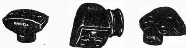
Fig. 8. Weather head fittings of the types shown above are used on the end of conduit at the service entrance to prevent water from entering the conduit.
