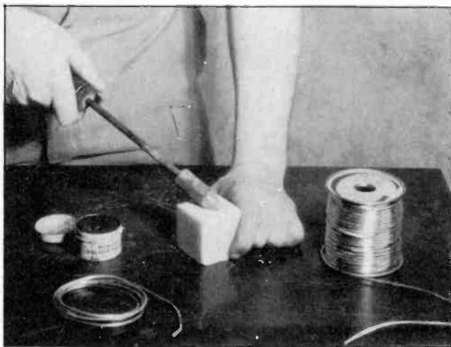
Fig. 4. This photo shows the method of cleaning and tinning a soldering copper with a block of salammoniac.
