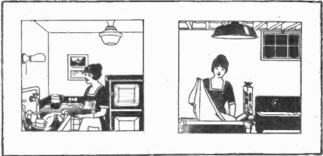
Fig. 19. At the left is shown the arrangement of ceiling unit and wall bracket light for kitchen. On the right a very efficient type of reflector for laundry rooms and basement lighting.
