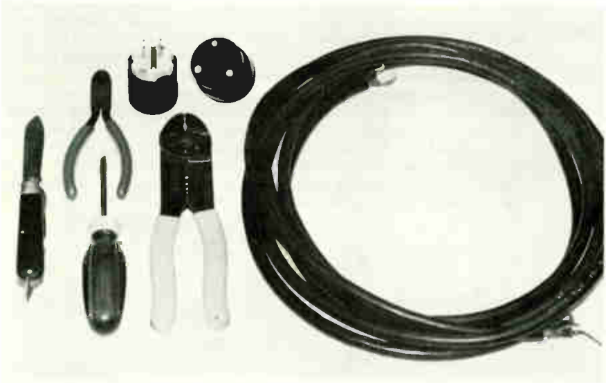
Fig. 25 First step in any project: organize your work and tools. For our portable heavy-duty extension cord, we'll use Type SJT, AWG #14/3 (three-conductor) cord. Markings on the outer covering of the cord identify these parameters. This cord was taken from an extension cord whose receptacle had been damaged. Clockwise from the cord—the tools we'll use in this project: wire stripper, flat-bladed screwdriver, pocket knife, diagonal wire cutter, and replacement male plug and female receptacle.
