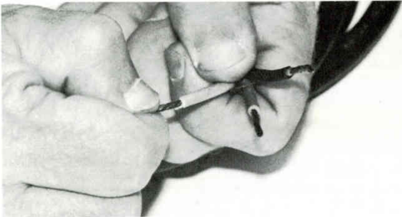
Fig. 31 Tightly twist the exposed ends of the stranded conductors in a clockwise direction using your thumb and forefinger in a clockwise direction. Make sure all of the strands are twisted together. Loose strands can become short circuits when you put the finished product to use.
