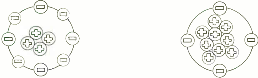
(a) Negative ion (more electrons than protons) (b) Positive ion (fewer electrons than protons)
