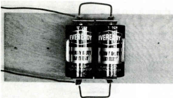
Fig. 4 Batteries connected in parallel.
