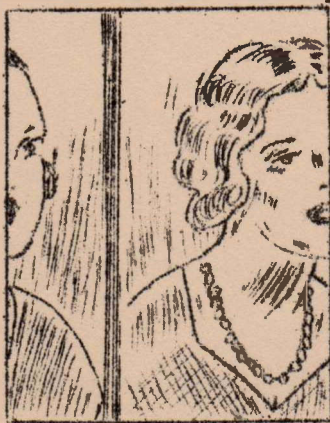
FIGURE 2. HORIZONTAL DISPLACEMENT OF PICTURE DETAIL AS RES- ULT OF LACK OF CORRECT LINE SYNCHRONISATION.
