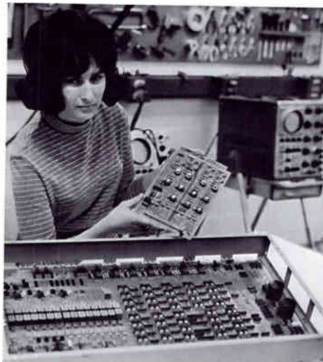
The basic Prodac 2000 computing control system is made up of only four large plug-in circuit boards such as the one in the foreground. The four boards take the place of the considerably larger number of smaller boards, such as the one the girl is holding, in traditional computer construction. One advantage is that, if something goes wrong, the user can quickly replace the faulty board with a spare instead of having to check dozens of small boards to find the fault.
