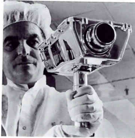
Lightweight television camera was used in the Apollo 9 mission and is scheduled for use in the lunar-landing mission. It is built to operate in atmosphere or vacuum and in the searing heat and intense cold of the lunar day and night. The image tube's wide sensitivity range will enable it to produce pictures during lunar night as well as lunar day.
