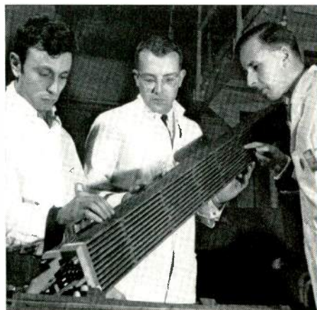
Fig. 3 (Far left) Fuel pellets and tubes for the fuel elements. (Left) A completed fuel element.
