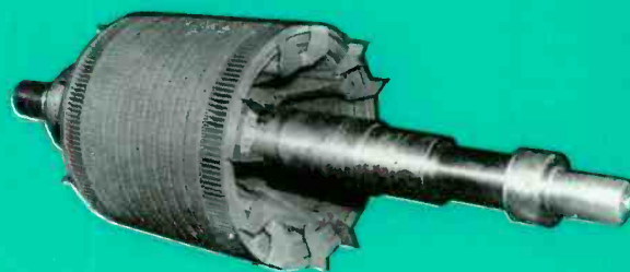
Fig. 4—Large brazed rotor, showing bar and end ring arrangement (400-hp double cage motor).
