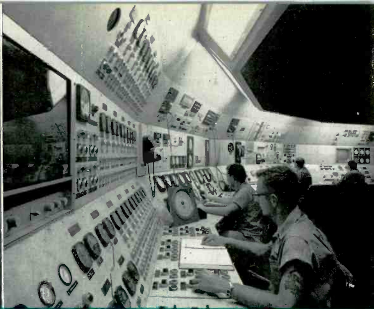
With these instruments in the main control room, flight conditions are simulated in the tunnel. In the supersonic portion, speeds of about 3000 mph at 100 000 feet can be simulated.
