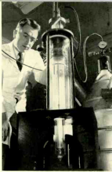
Here Dr. John Hulm of the low-temperature laboratory prepares a demonstration of superconductivity. The container is double-walled; the inner portion contains liquid helium, the outer, liquid nitrogen. For the demonstration a ring of superconducting material is immersed in the helium, and power applied. After removal of the power source, current continues.
