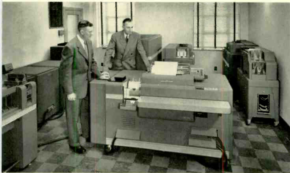
This card-program-calculator installation is typical of the increasing use of computers in engineering departments. This computer is directed by information from punched cards as they are read into the machine.
