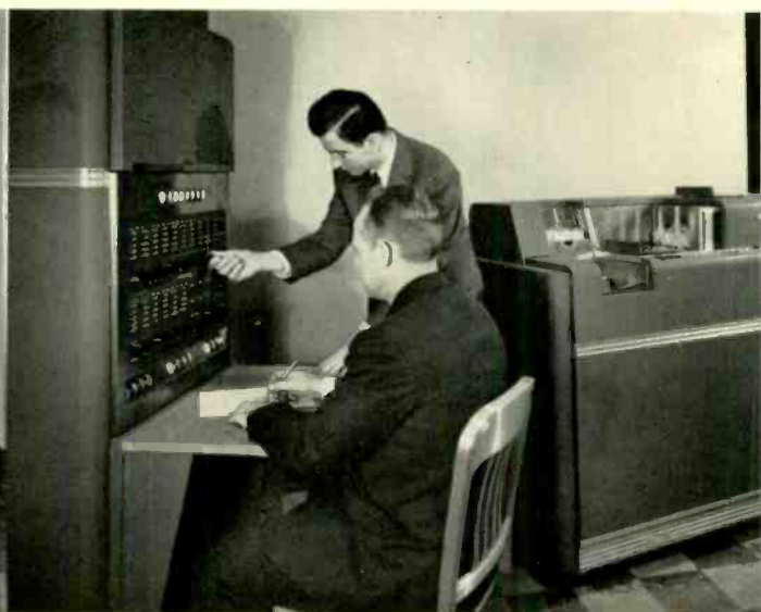
The data processing machine is another computer now employed for engineering design work. This machine has a "memory" for 2000 ten-digit words.
