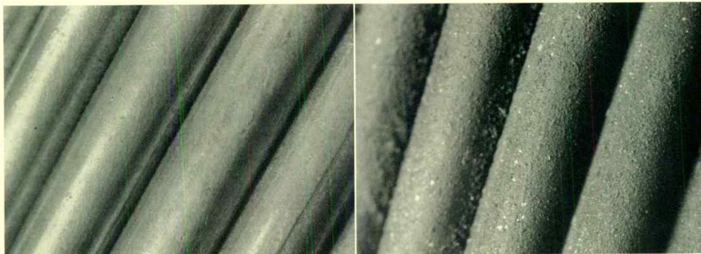
Fig. 1—You can see from these microphotos how the appearance of a two-inch ACSR conductor changes with age. The picture at the left is a new conductor. The one at the right is
